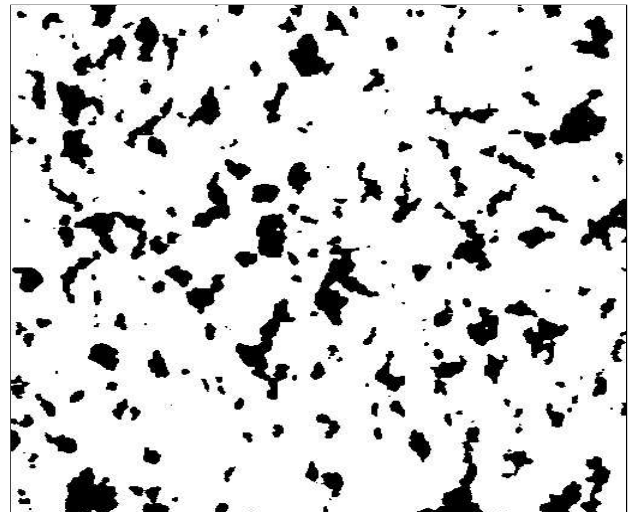
Figure 3.19 : Fe/Cu CIC H329 - c_{Fe} = 16,1\% - \times 60
