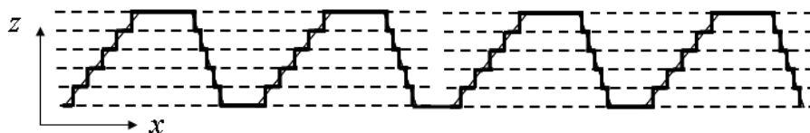
Figure 4.9: Slicing of a one-dimensional grating, invariant following y in a superposition of lamellar gratings.
