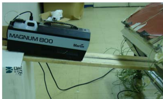
Figure 3 - Photo of the smoke machine in front of the inlet section.
