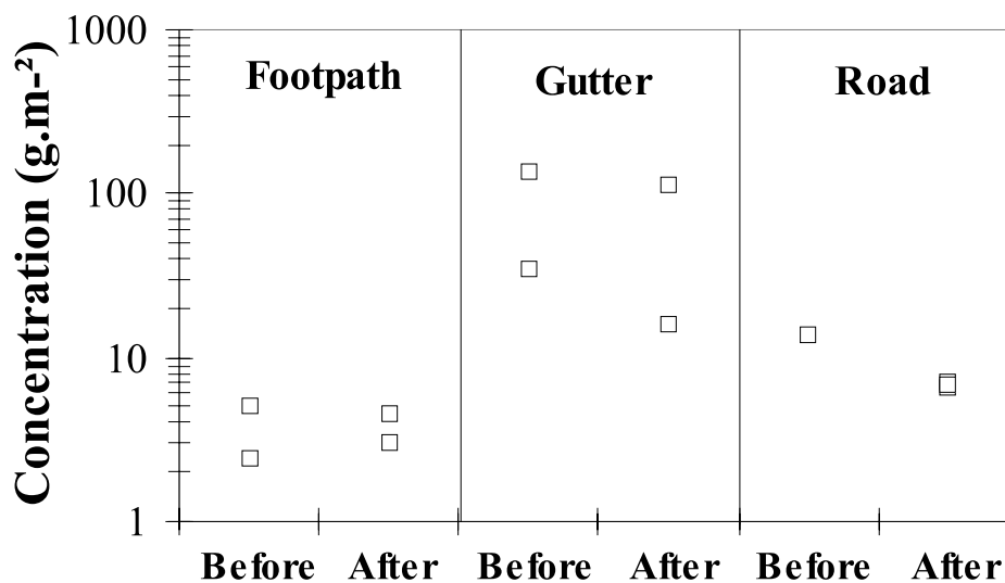
Fig. 6 Assessment of street cleaning efficiency on particle surface loads at Béarn street (June 19 th 1997) : comparison of bulk particles surface loads prior and after street cleaning
