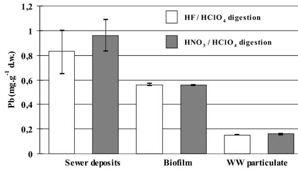
Figure 4: (a) Comparison of the dissolved metal determination using acidification at pH 1 or HNO<sub>3</sub>/HClO<sub>4</sub> digestion, and (b) of the particulate lead determination using HF/HClO<sub>4</sub> or HNO<sub>3</sub>/HClO<sub>4</sub> digestion
