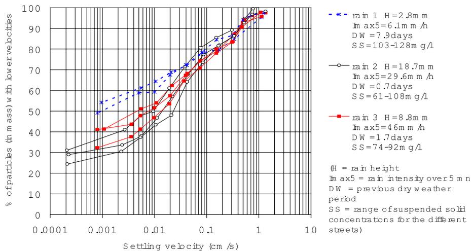
**Figure 4 :** Settling velocities, measured on street runoff event mean samples from 3 different streets and for 3 rain events
