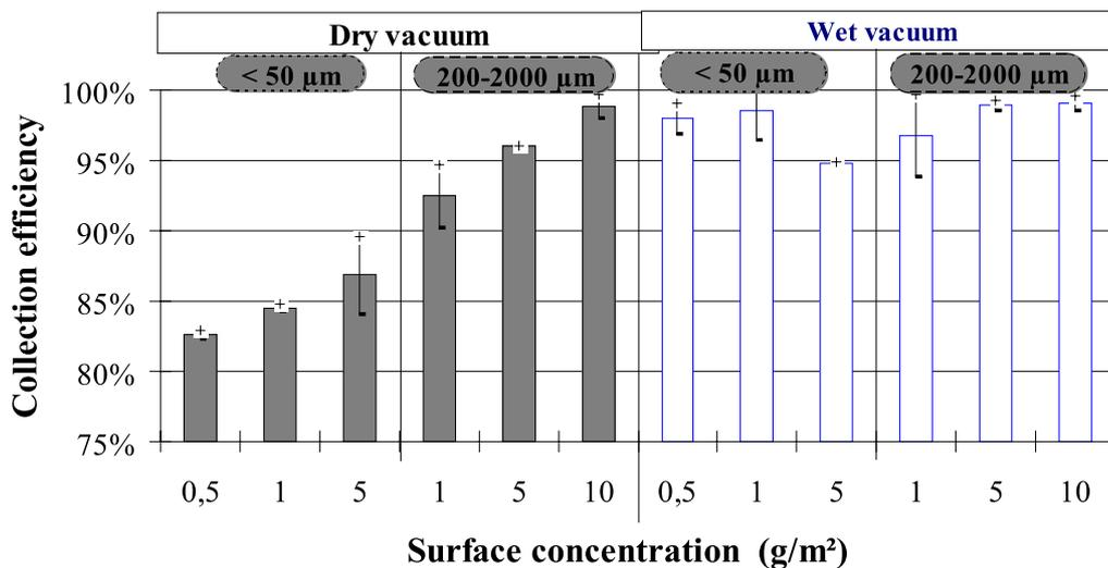
Fig. 3 Collection efficiencies of model experiments using dry (left diagram) or wet vacuum sampling (right one) and various surface concentrations of calcinated and sieved clay (< 50  $\mu\text{m}$ ) or gutter sediments (200 – 2 000  $\mu\text{m}$ ) deposited on the laboratory floor (see Fig. 1) : mean  $\pm$  dispersion of duplicates
