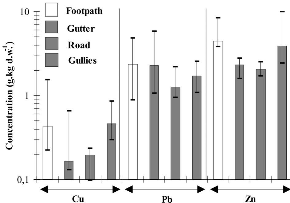
Fig. 4 Particulate metal concentrations in Béarn street deposits : median and variation range ( $n = 7-8$ ) on June 12<sup>th</sup> and 19<sup>th</sup> 1997 samples collected on footpath, gutter and road. Comparison with median and deciles metal concentrations in particles sampled on 3 gullies within the experimental urban catchment (Fig. 2) in 1996 – 1997 ( $n = 15$ )
