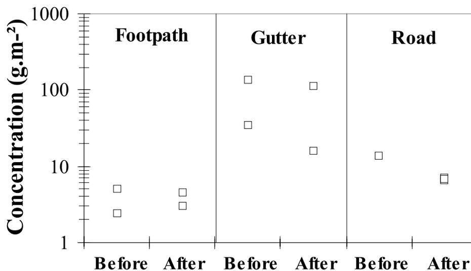
Fig. 6 Assessment of street cleaning efficiency on particle surface loads at Béarn street (June 19<sup>th</sup> 1997) : comparison of bulk particles surface loads prior and after street cleaning
