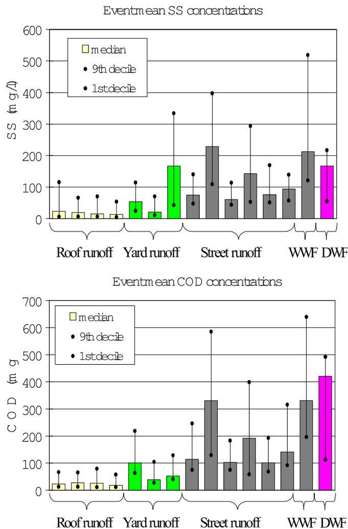
Figure 2 : Median concentrations in SS and in COD and upper-lower decile range, for the different measurement sites (in mg.l<sup>-1</sup>).
