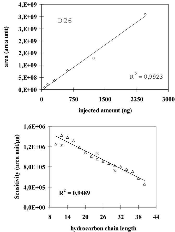
Figure 2: (a) Sensitivity determination: area of perdeuterated Dodecane D<sub>26</sub> peaks vs. injected mass, (b) sensitivity vs. hydrocarbon chain length with (□) non perdeuterated or (\*) perdeuterated hydrocarbons
