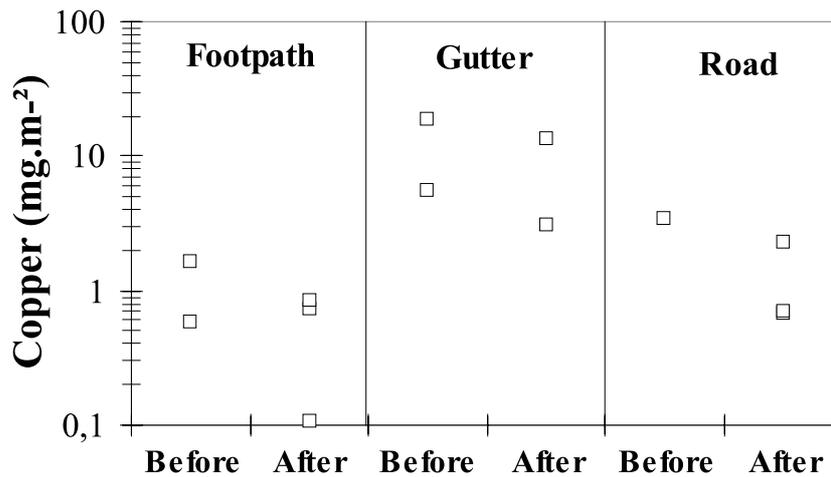
Fig. 7 Assessment of street cleaning efficiency on metal surface loads at Béarn street (June 19<sup>th</sup> 1997) : comparison of bulk particulate copper, lead and zinc surface loads prior and after street cleaning
