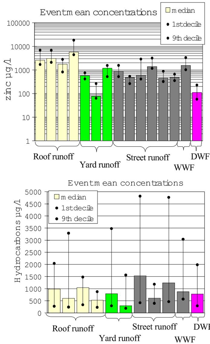
Figure 5 : Median concentrations in zinc and in hydrocarbons, and upper – lower decile range, at different measurement points (in  $\mu\text{g.l}^{-1}$ ).
