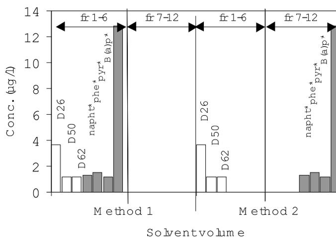
Figure 3: Comparison between two separating methods of aliphatic and aromatic hydrocarbons, using adsorption chromatography: fr i-j refers to the volume (ml) of eluting solvent and D<sub>26</sub> to Dodecane, D<sub>50</sub> to Tetracosane, D<sub>62</sub> to Triacontane and napt\* to Naphtalene D<sub>8</sub>, phe\* to Phenanthrene D<sub>10</sub>, pyr\* to Pyrene D<sub>10</sub>, B(a)p\* to Benzo(a)pyrene D<sub>12</sub>
