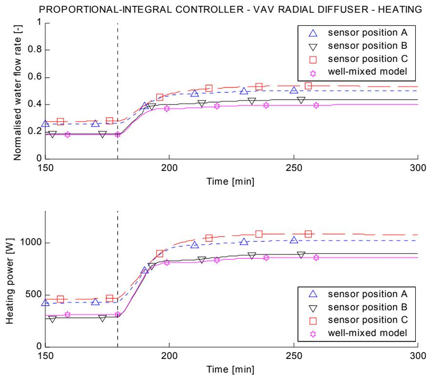
Figure V - 30: Normalised water flow rate through coil and heating power
