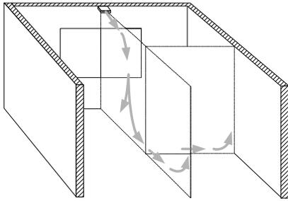
Figure II - 6: Airflow pattern: type 2 – high positive buoyancy forces
