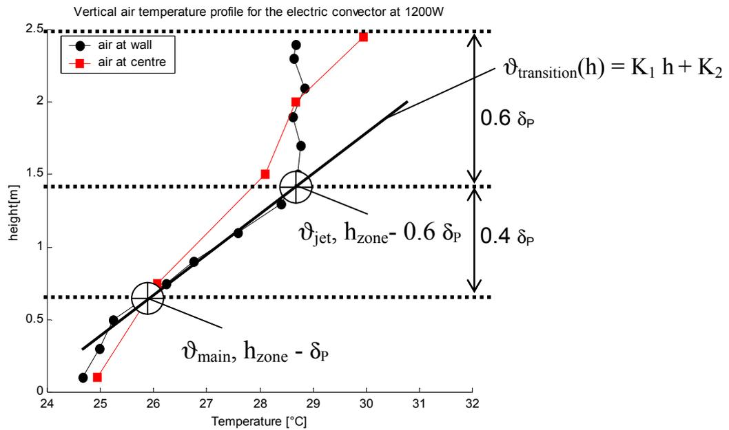
Figure IV - 26: Definition of the function for the temperature in the zone of transition of the wall jet
