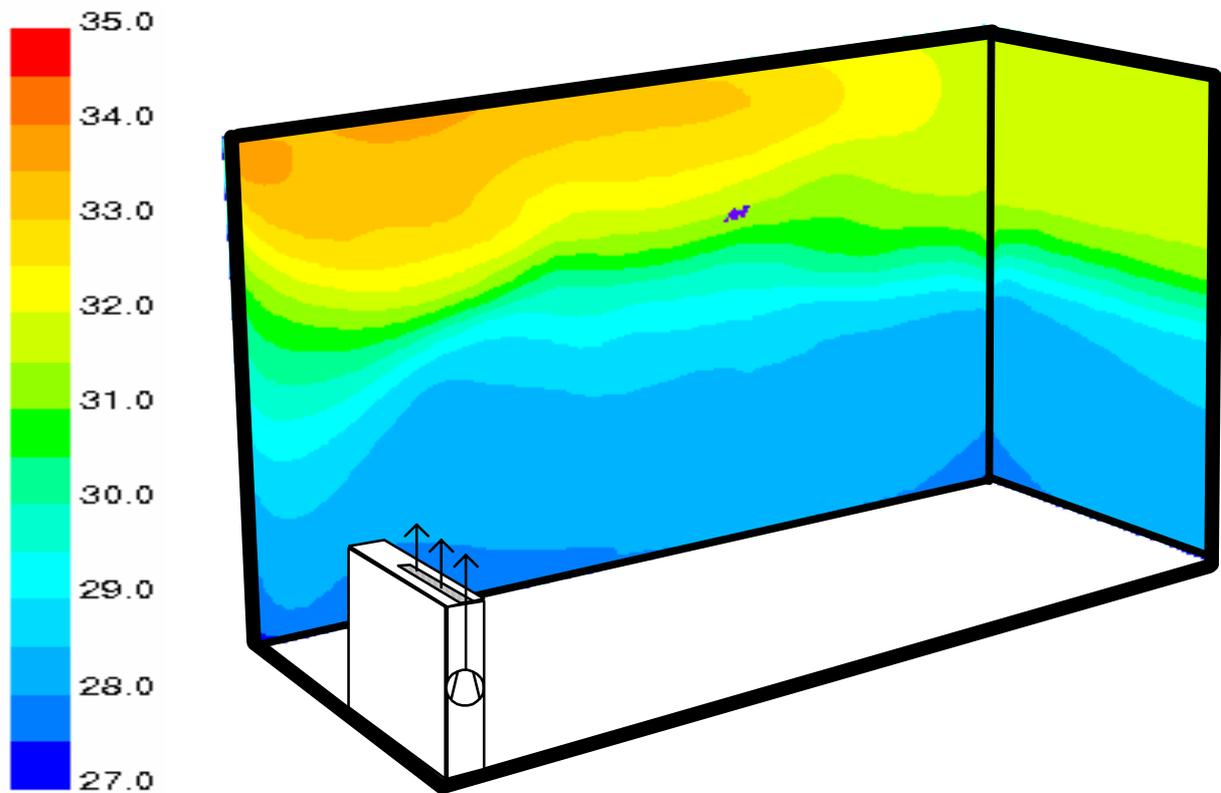
Figure II - 40: Simulated temperature profile 5cm from walls and ceiling for the fan coil unit (fan speed 1)
