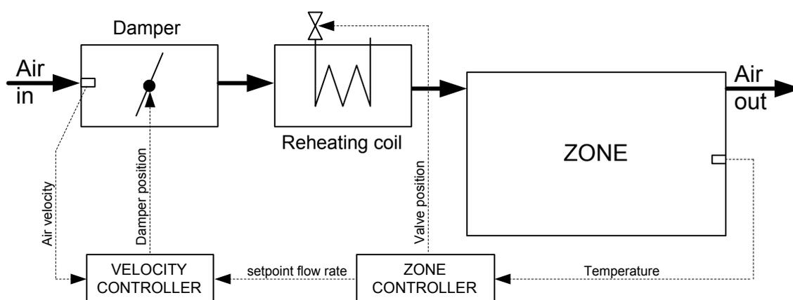
Figure V - 5: VAV system on the room level
