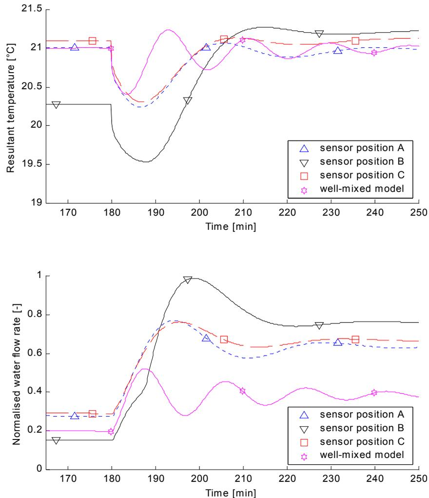
Figure V - 33: Single zone simulation after tuning of the controller using zonal model and sensor position B
