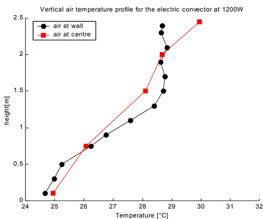
Figure II - 33: Vertical temperature profile - convector – favourable boundary layer - EREDIS
