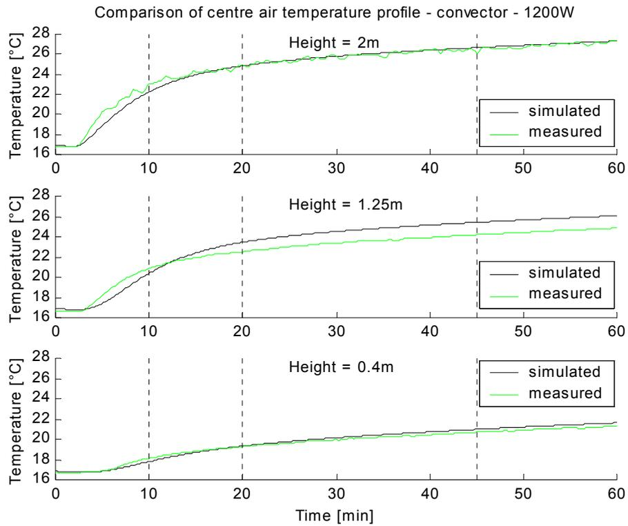
Figure IV - 39: Validation of the room model for the electric convector - centre temperature - 1200W
