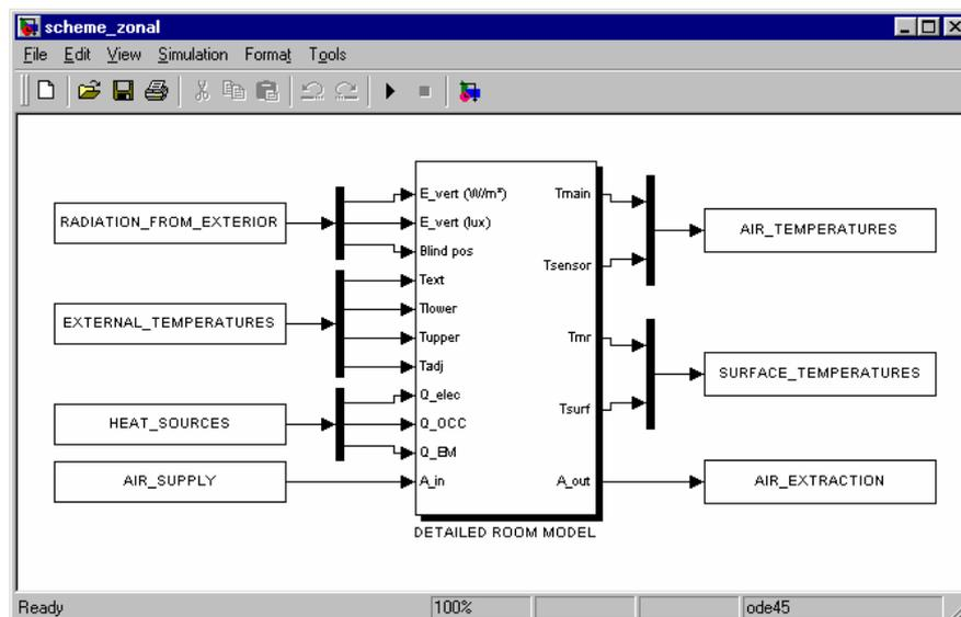
Figure IV - 29: Room model with principal inputs and outputs
