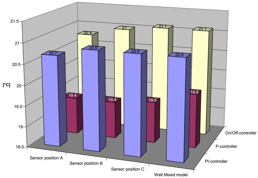
Figure V - 24: Mean resultant temperature - VAV slot diffuser heating
