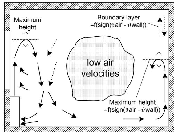
Figure II - 18: Airflow pattern B in the EREDIS test room with a cooling system – smoke visualisation
