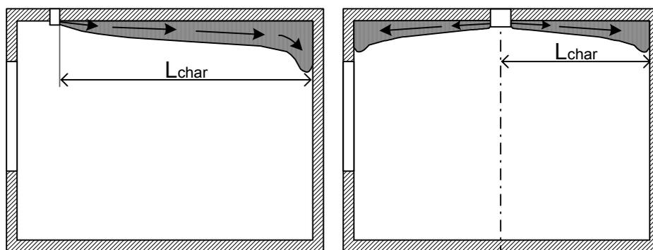
Figure V - 3: Diffuser design by jet mapping
