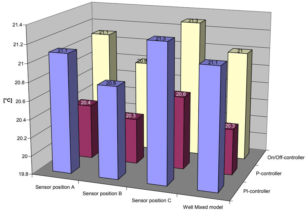
Figure V - 10: Mean resultant temperature - FCU heating
