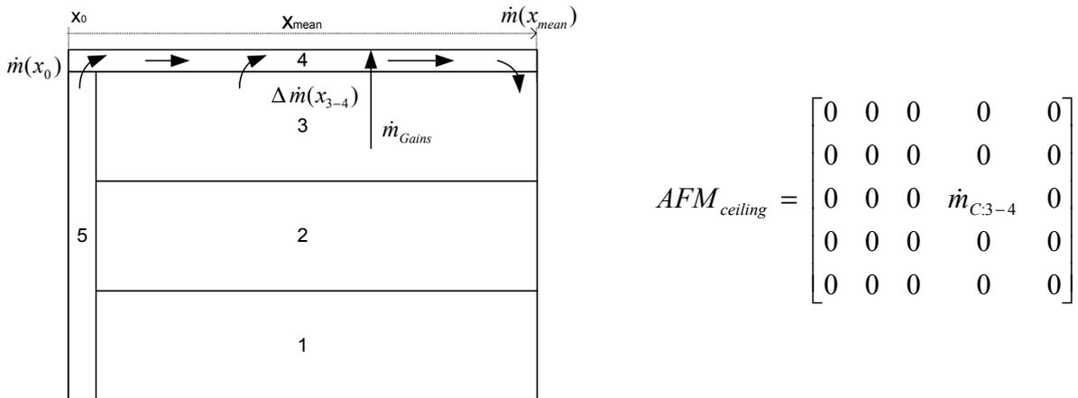
Figure IV - 19: Air flow due to the ceiling jet
