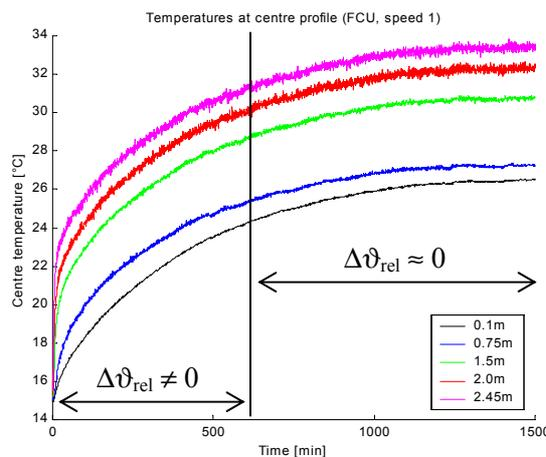
Figure II - 49: Evolution of air temperatures at centre profile (test OFF → ON) - EREDIS
