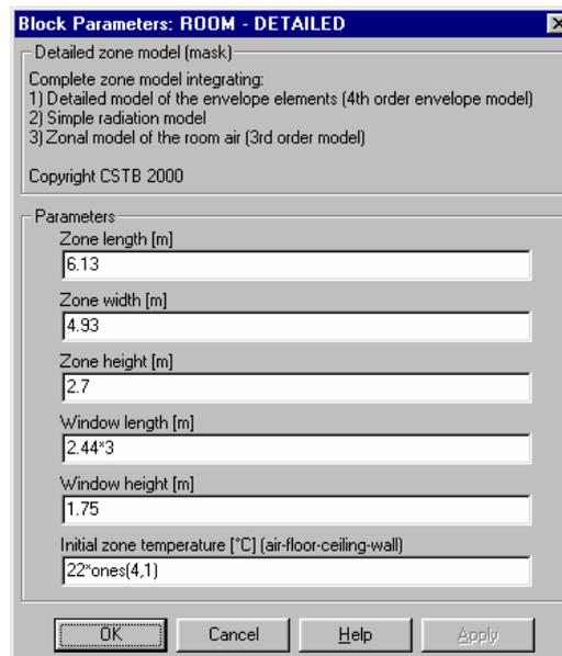
Figure IV - 30: Main parameters of the room model
