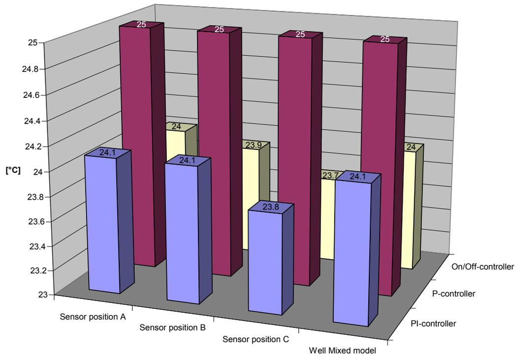
Figure V - 21: Mean resultant temperature - VAV radial diffuser cooling
