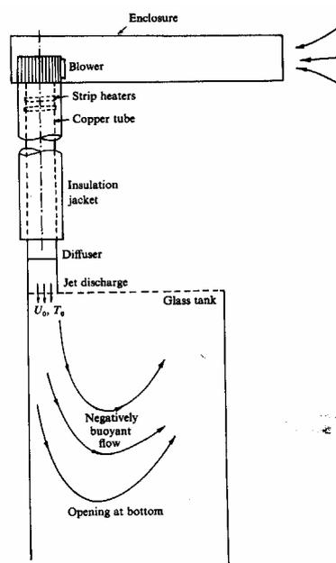
Figure IV - 12: Experimental arrangement used by [Kapoor88] and [Goldmann86]
