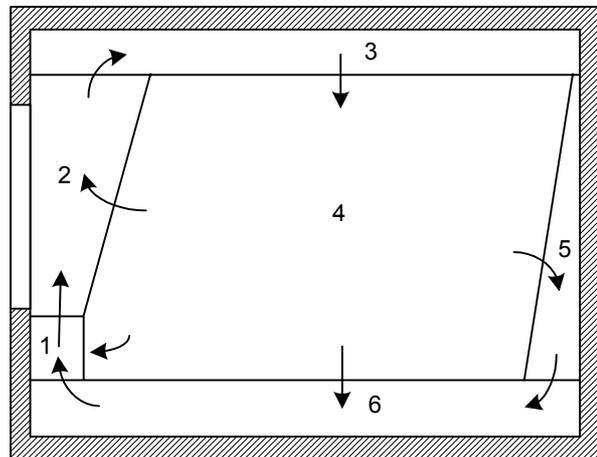
Figure III - 11: Zone with convector/radiator ([Inard88])
