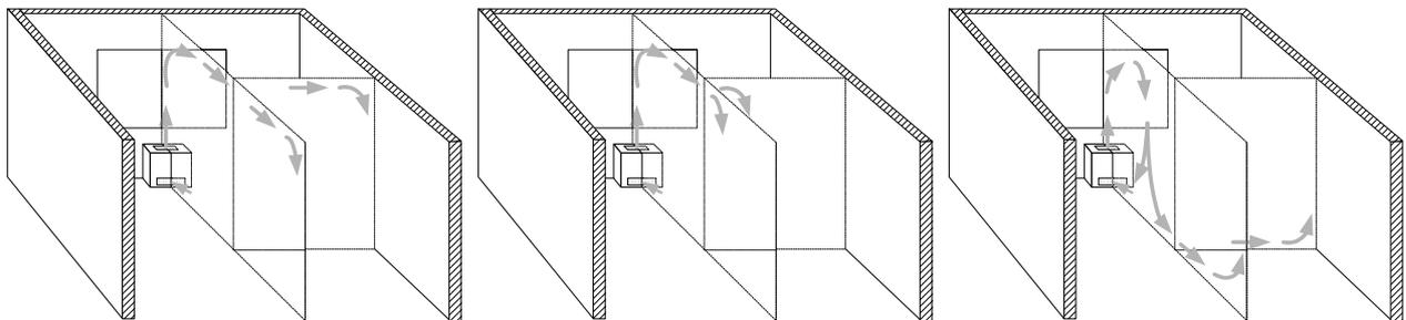
Figure II - 3: Airflow pattern: type 1 – high positive buoyancy forces
