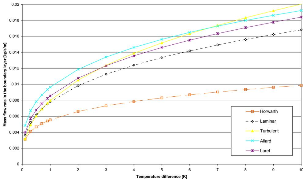
Figure IV - 11: Flow rate in a boundary layer for varying temperature difference
