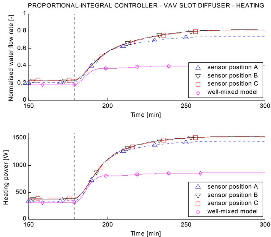
Figure V - 26: Normalised water flow rate through coil and heating power
