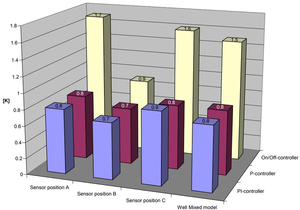
Figure V - 8: Maximum amplitude in resultant temperature - electric convector
