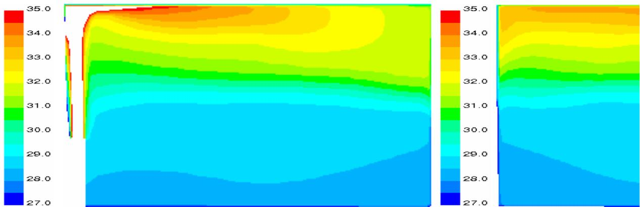
Figure II - 23: Zone temperature on symmetric axis and on vertical cut through centre (FCU, speed 1)
