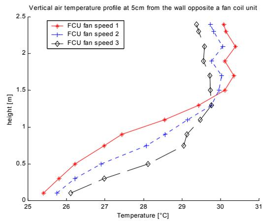
Figure II - 47: Measured stratification of sensor air temperature for a fan coil unit - EREDIS
