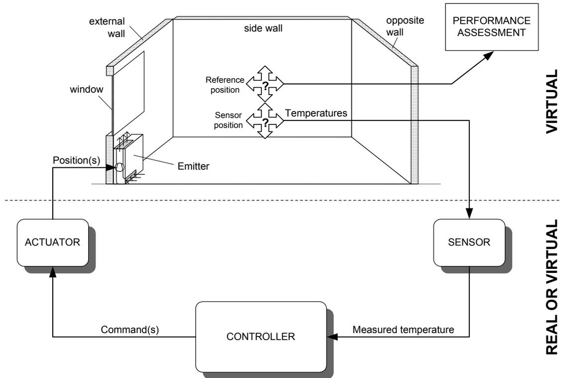
Figure III - 2: Principle of controller test and performance assessment
