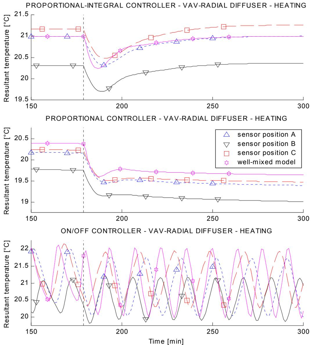
Figure V - 27: Resultant temperature - VAV system with radial diffuser - heating
