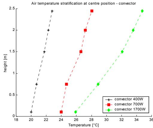
Figure II - 24: Temperature stratification at centre position – electric convector - EREDIS test cell
