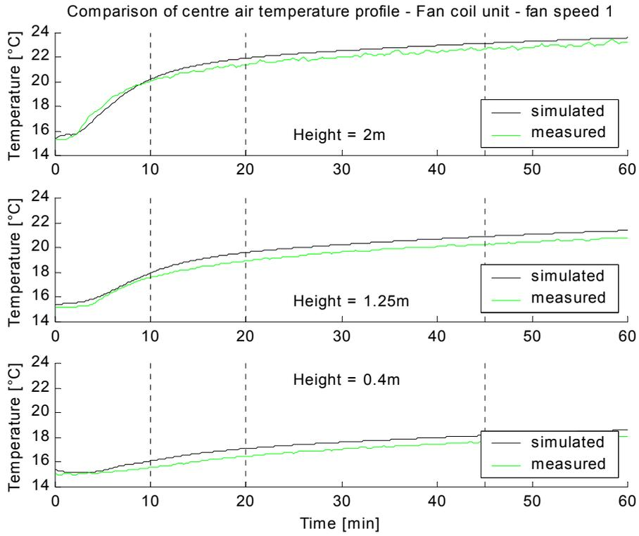
Figure IV - 41: Validation of the room model for the fan coil unit - centre temperature - fan speed 1
