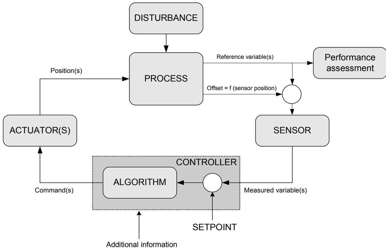
Figure I - 3: Revised scheme of a control loop
