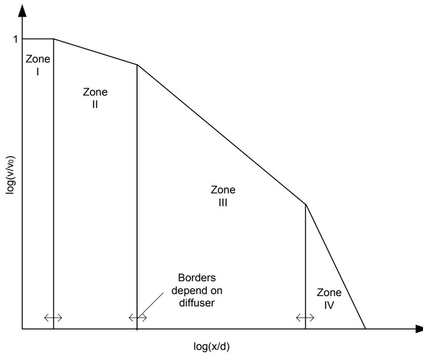
Figure IV - 8: Zones of expansion of a jet
