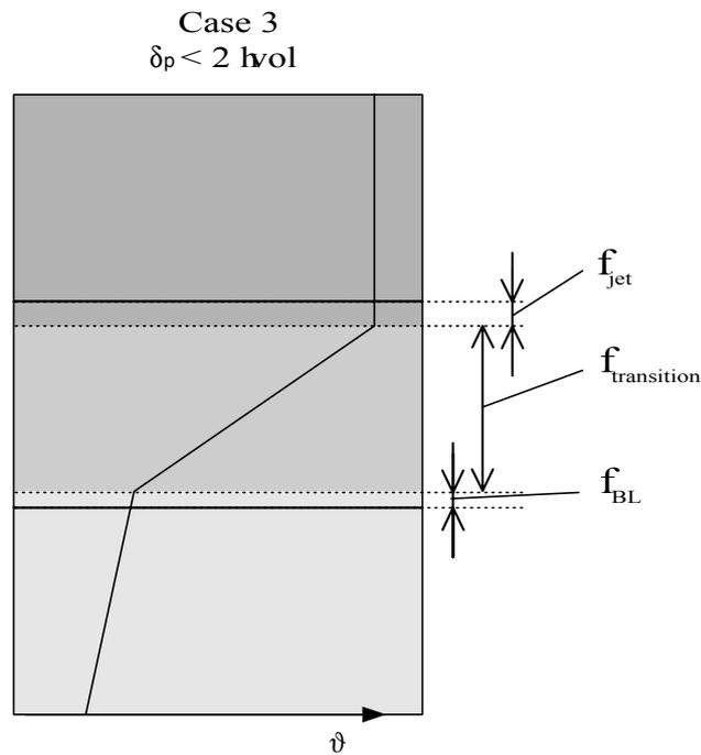
Figure IV - 28: Definition of the weighting factor for the calculation of sensor temperatures
