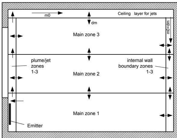
Figure IV - 3: Section AA through the room
