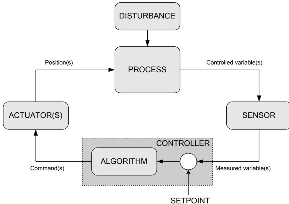
Figure I - 1: General principle of a control loop
