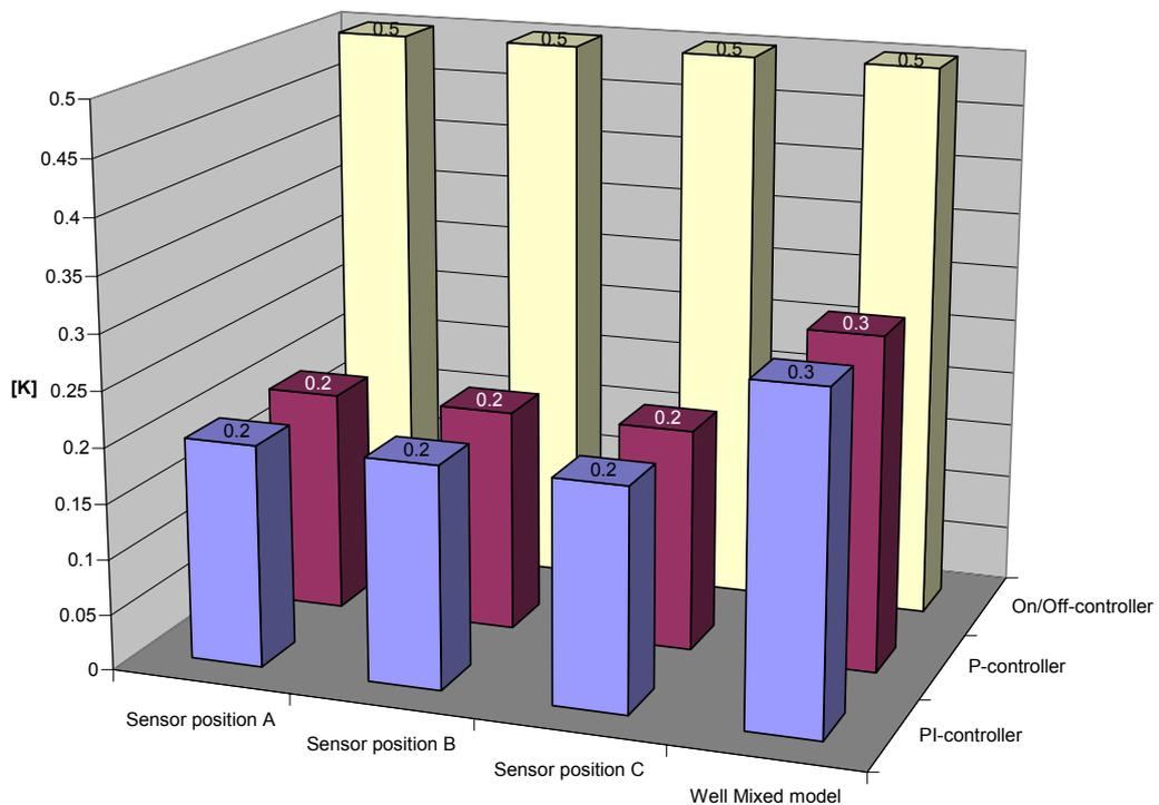
Figure V - 14: Maximum amplitude in resultant temperature - FCU cooling
