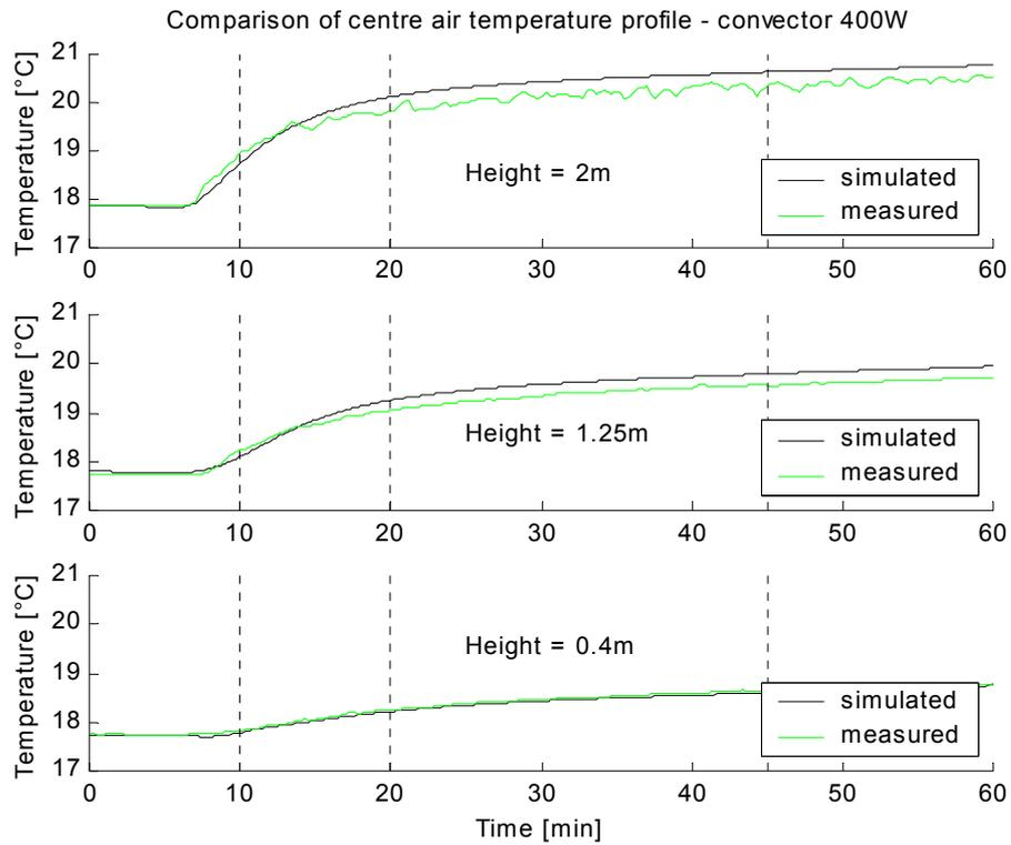
Figure IV - 35: Validation of the room model for the electric convector - centre temperature - 400W
