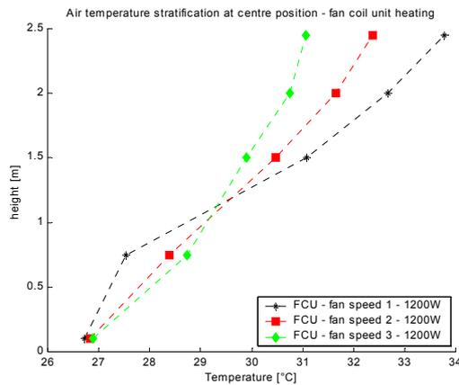
Figure II - 25: Temperature stratification at centre position – fan coil unit – heating - EREDIS test cell
