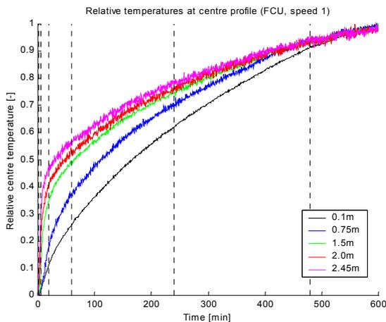
Figure II - 51: Evolution of relative temperature at centre profile (test OFF → ON) - EREDIS
