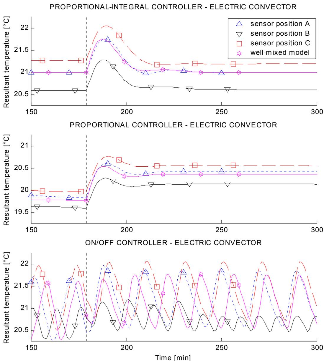
Figure V - 6: Resultant temperature - electric convector
