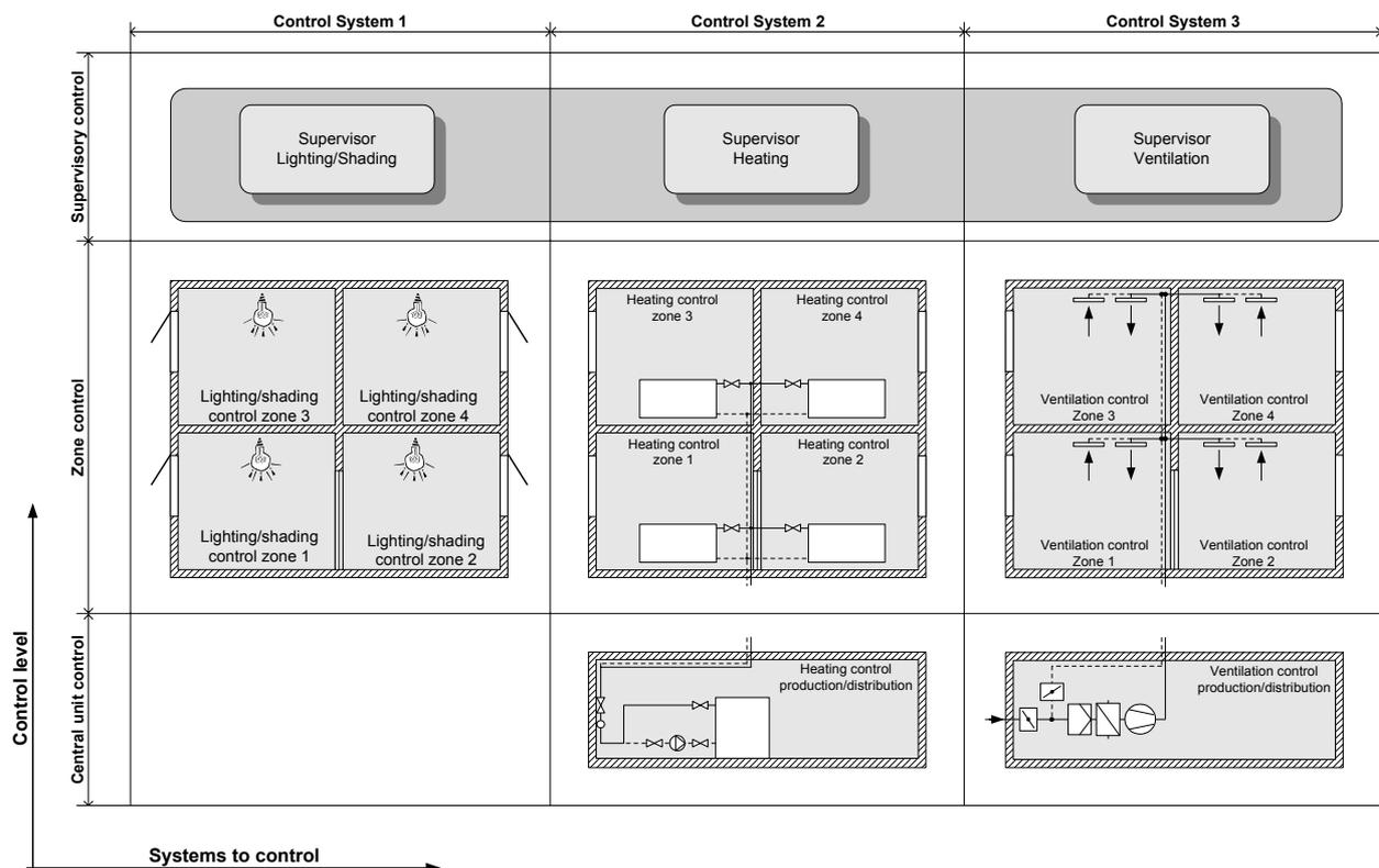
Figure I - 2: Example for different levels of building control
