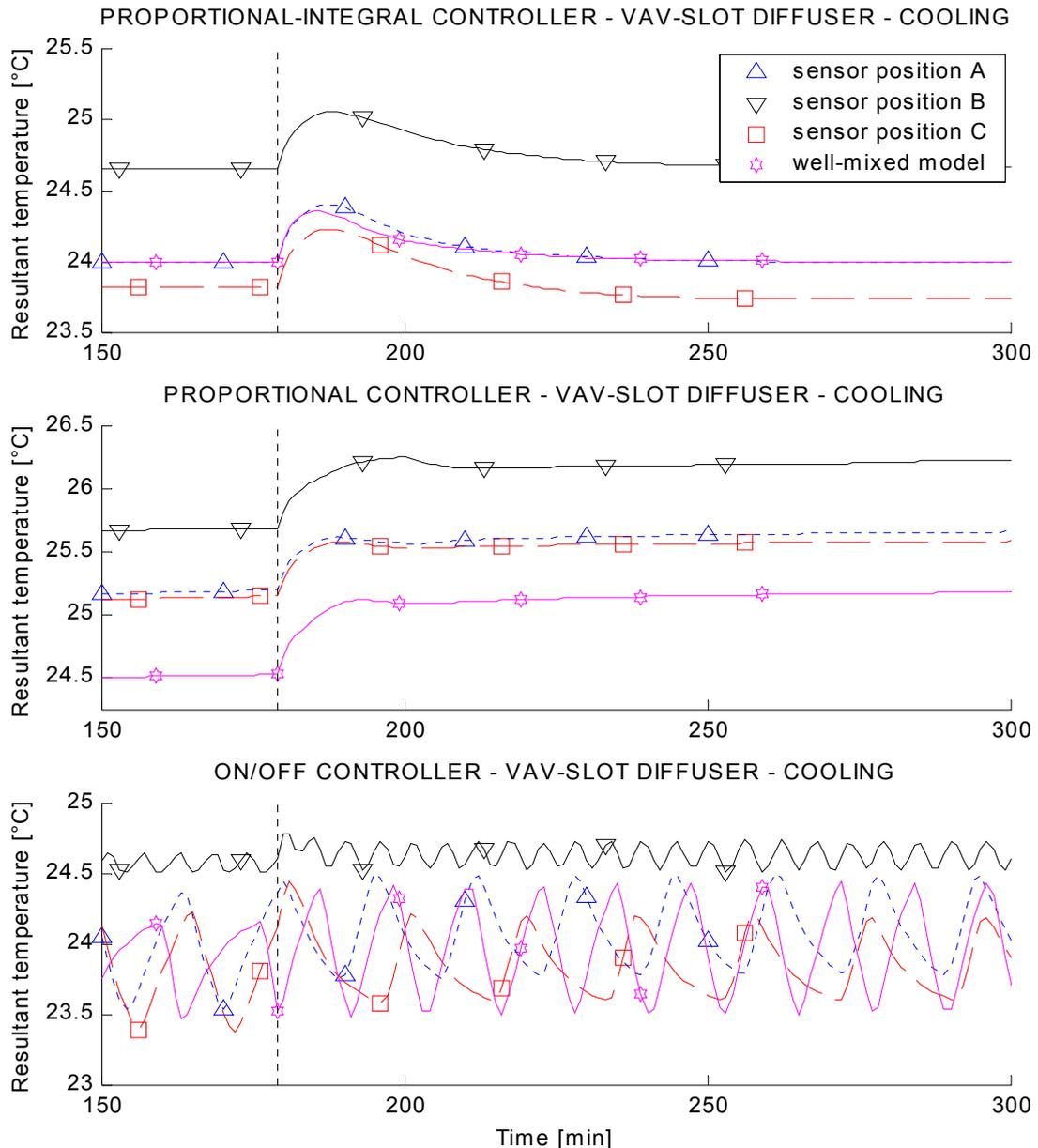
Figure V - 16: Resultant temperature - VAV system with slot diffuser - cooling
