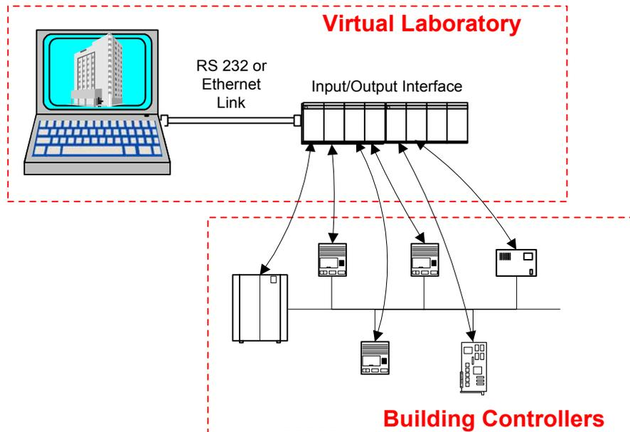
Figure I - 4: Principle of a virtual laboratory used for the test of real building controllers
