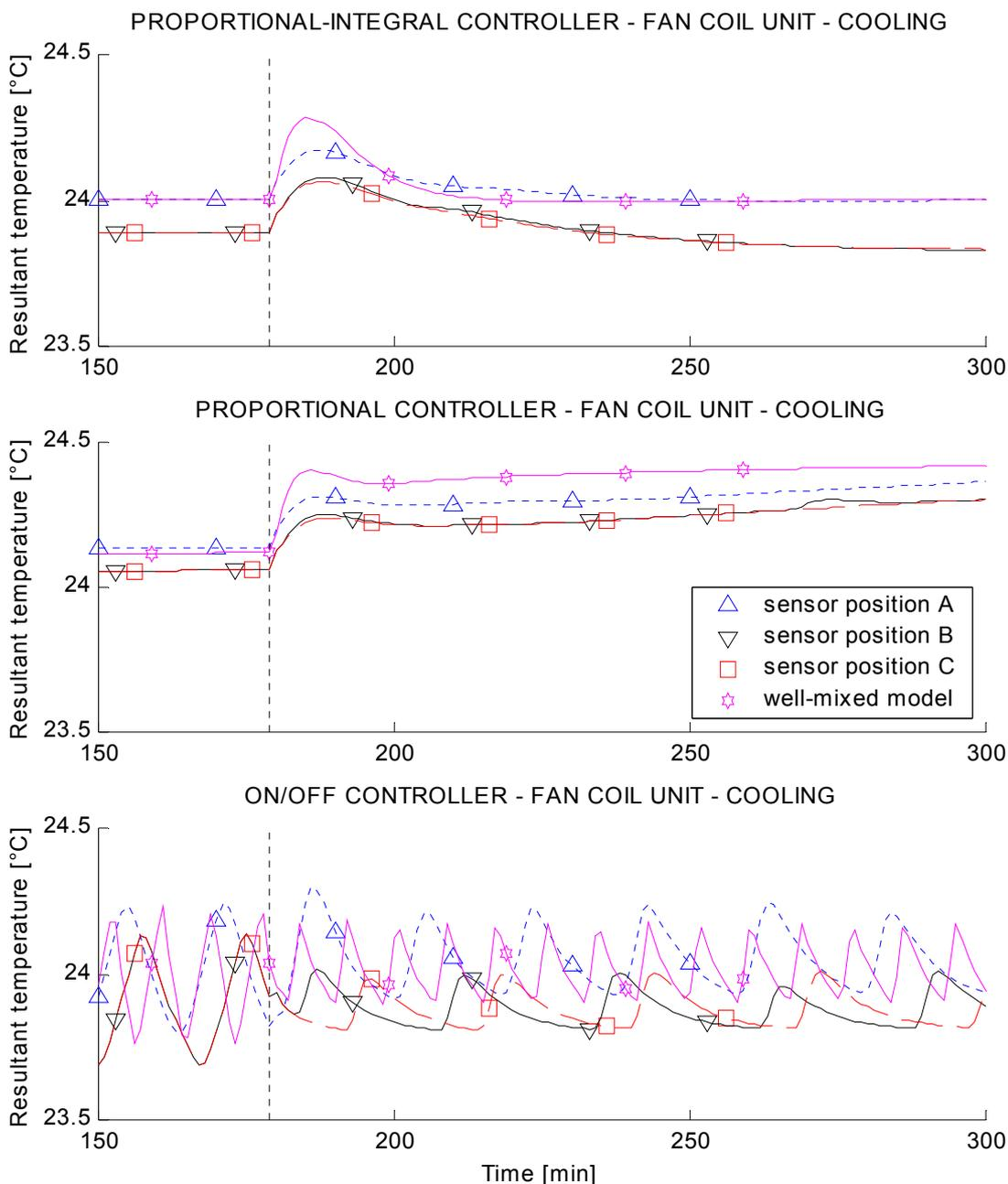
*Figure V - 12: Resultant temperature - fan coil unit - cooling*
