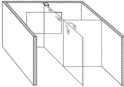
Figure II - 7: Airflow pattern: type 2 – low buoyancy forces
