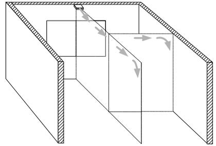
Figure II - 8: Airflow pattern: type 2 – high negative buoyancy forces
