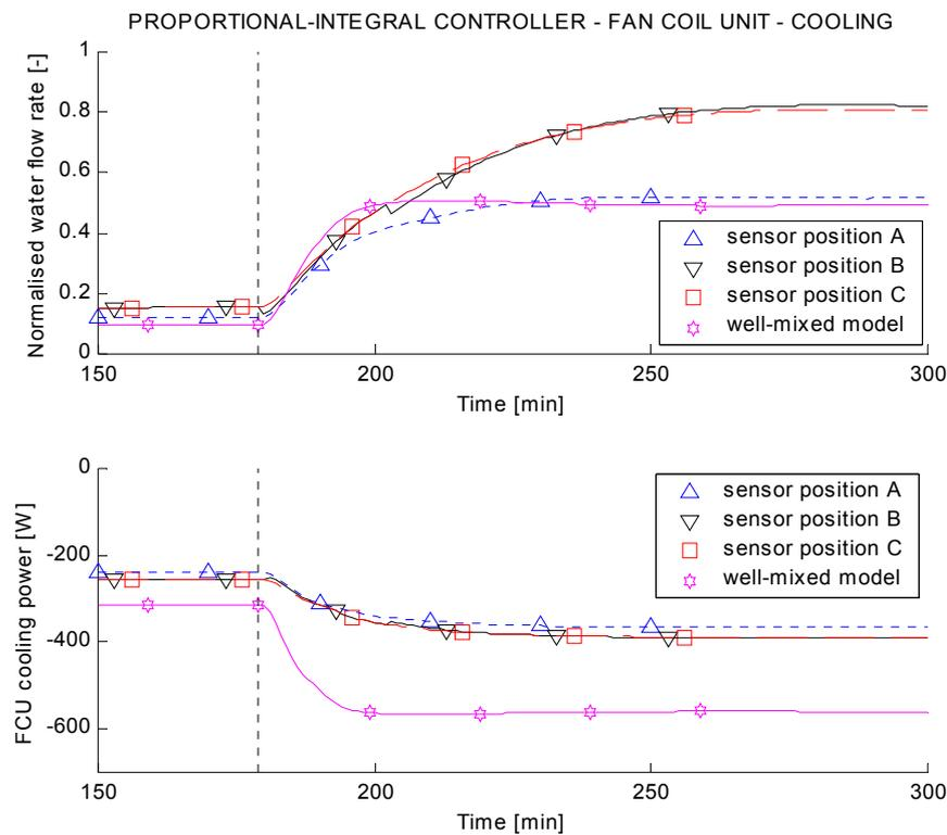
Figure V - 15: Normalised water flow rate through coil and FCU cooling power
