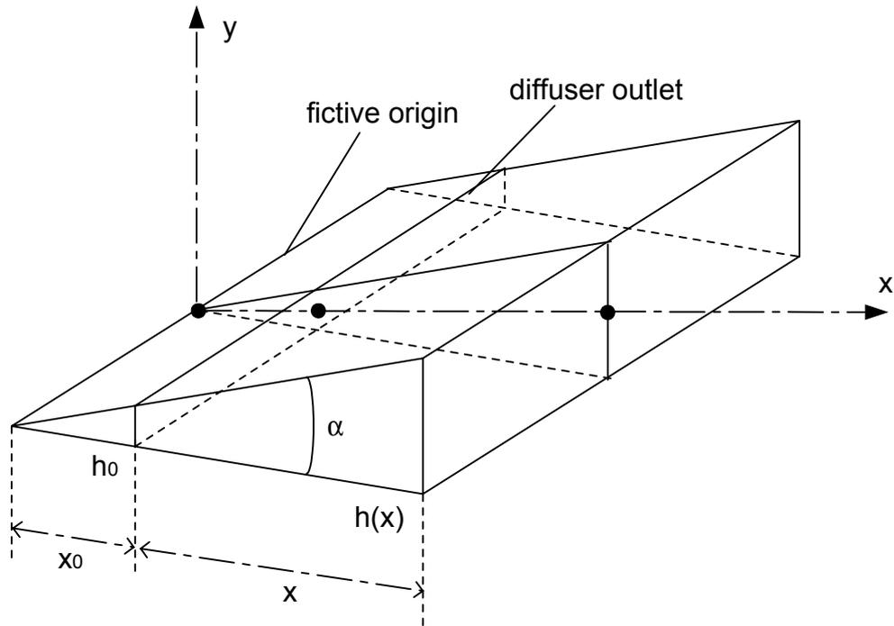
Figure IV - 6: Scheme of the plane jet with definitions
