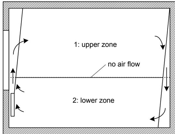
Figure III - 9: Zone with radiator ([Horwarth80])
