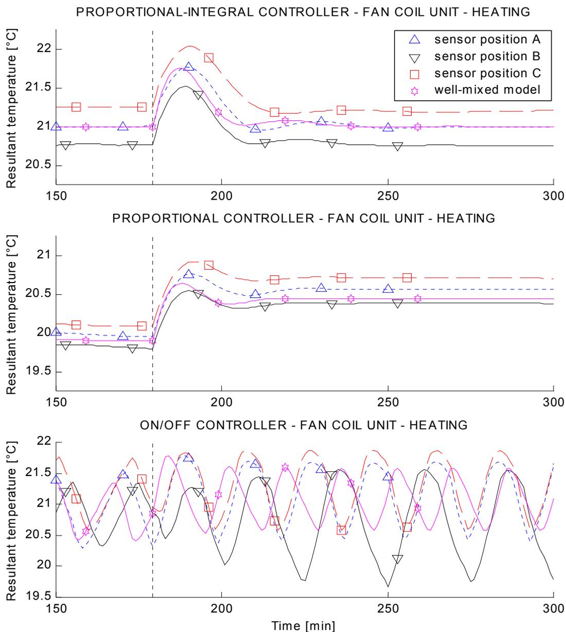
Figure V - 9: Resultant temperature - fan coil unit - heating
