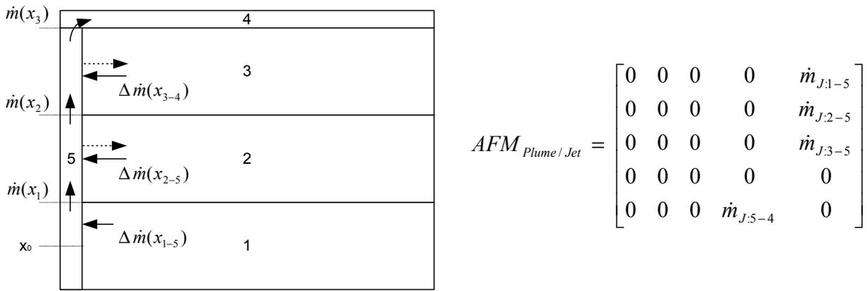
Figure IV - 17: Use of the plume/jet correlation in zone 4
