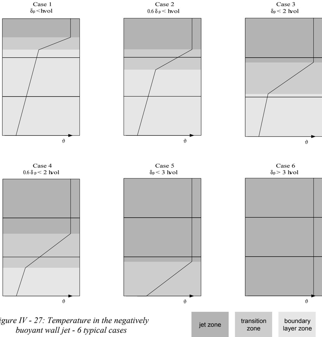
Figure IV - 27: Temperature in the negatively buoyant wall jet - 6 typical cases
