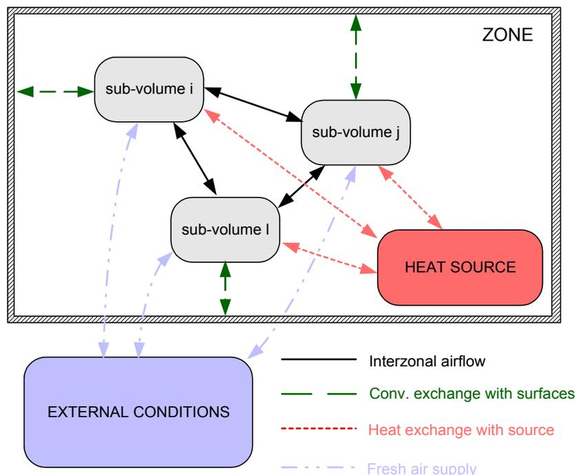
Figure III - 7: Principle of a zonal model
