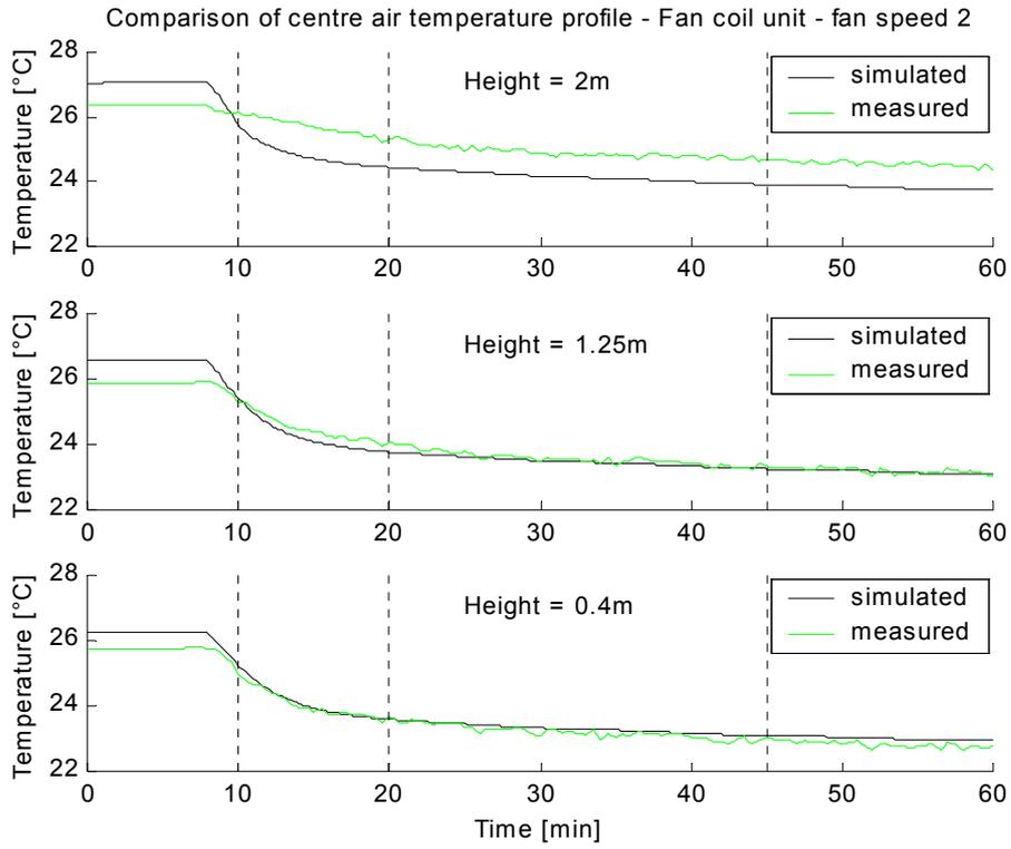
Figure IV - 47: Validation of the room model for the fan coil unit - centre temperature - fan speed 2
