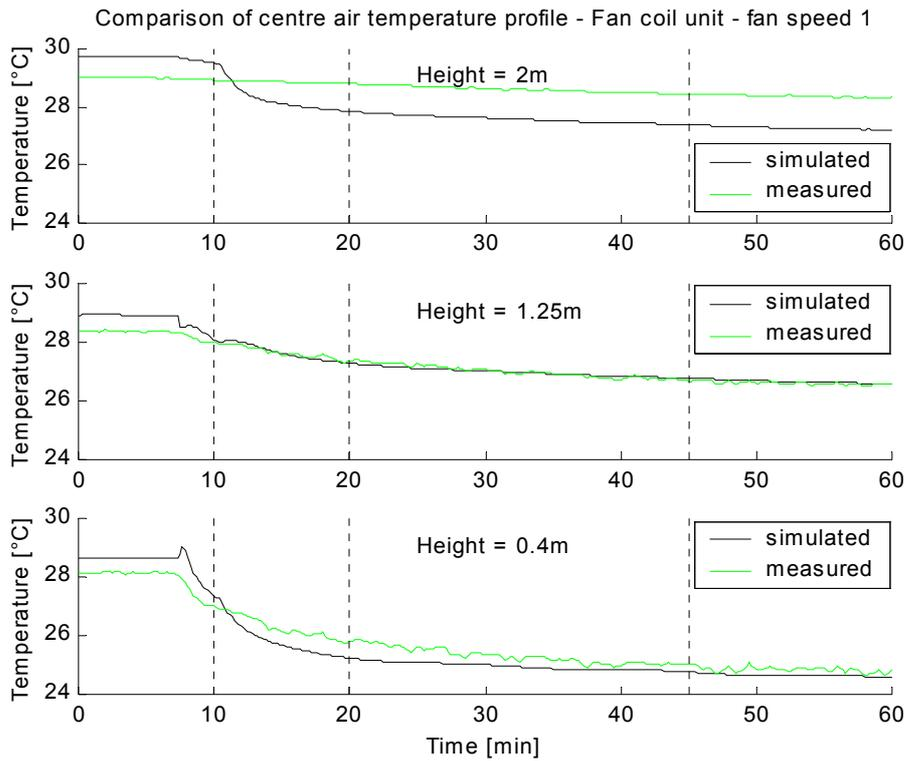
Figure IV - 45: Validation of the room model for the fan coil unit - centre temperature - fan speed 1
