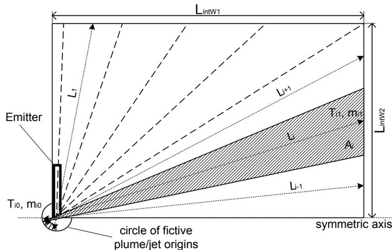
Figure IV - 20: Calculation of mean jet entrainment length
