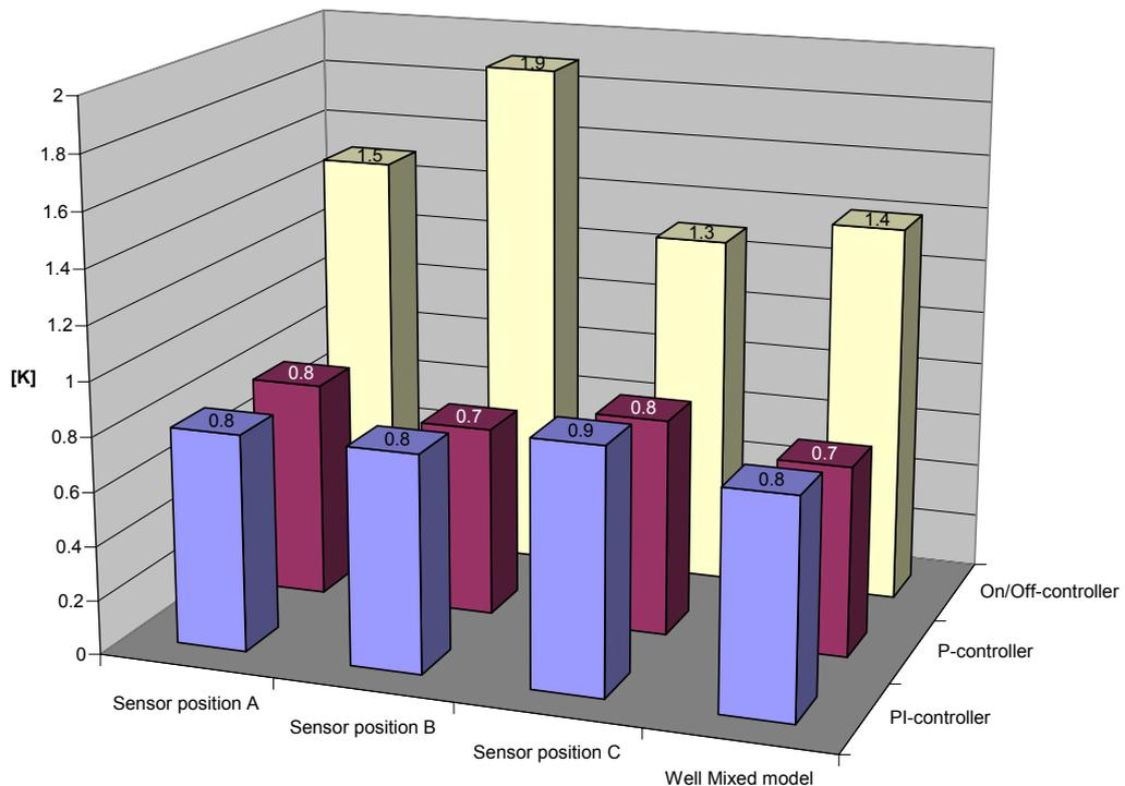
Figure V - 11: Maximum amplitude in resultant temperature - FCU heating
