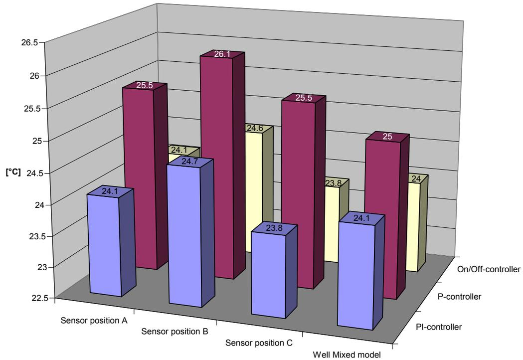
Figure V - 17: Mean resultant temperature - VAV slot diffuser cooling
