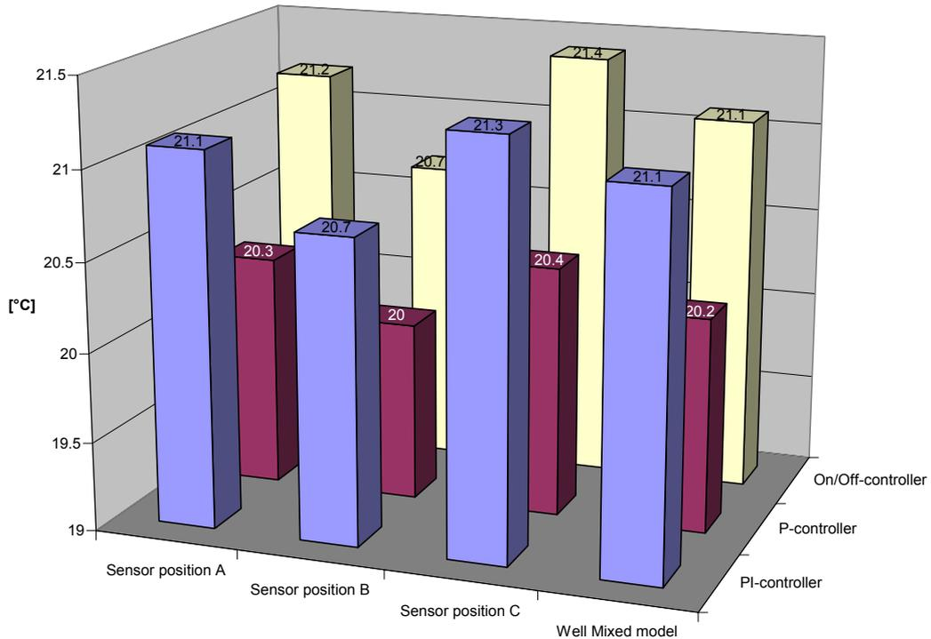
Figure V - 7: Mean resultant temperature - electric convector
