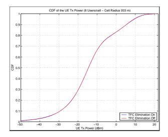
Figure 4.13: CDF of the UE transmission power (TFC Elimination "On and "Off", 8 UEs per cell, cell radius  $933~\mathrm{m}$ ).
