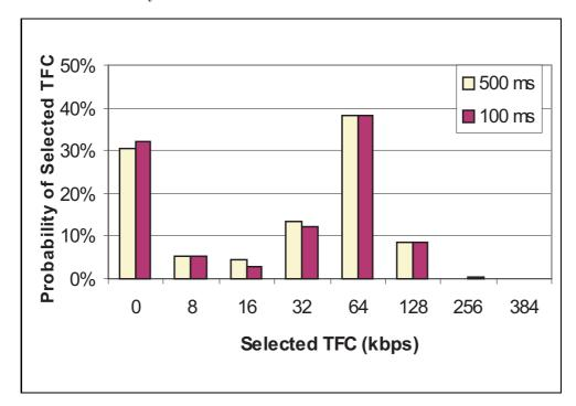
Figure 5.13: Probability of selected TFC for all of the users in the system, for the cases the packet scheduling period is 500 and 100 ms, (columns 1 and 2 respectively, 32 UEs per cell, traffic model scenario A).
