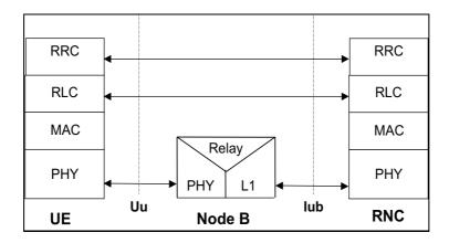
Figure 2.3: Control Plane protocol stack when dedicated channels are established between the UE and the network.
