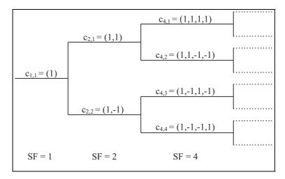
Figure 2.4: Code generation tree of the orthogonal variable spreading codes used in UTRAN.
