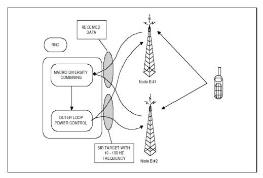
Figure A.2: Model of the outer loop power control in uplink.
