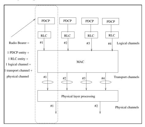
Figure 2.5: Configuration of an UE supporting more than one radio bearers (user plane protocol stack).
