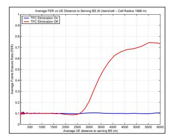
Figure 4.17: FER as a function to the distance from the serving BS (TFC Elimination "On" and "Off", 8 UEs per cell, cell radius 1866 m).
