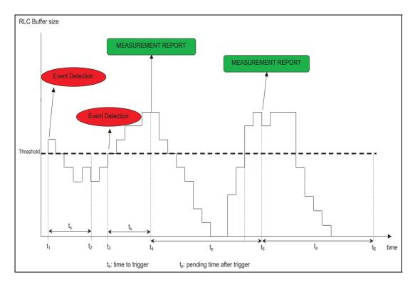
Figure 4.3: Timings in the Measurement Report sending procedure.
