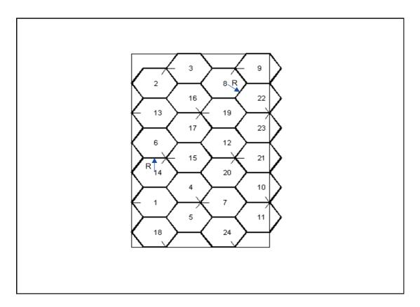
Figure 4.9: Network layout consisted of three-cell sector configuration with directional antennas.
