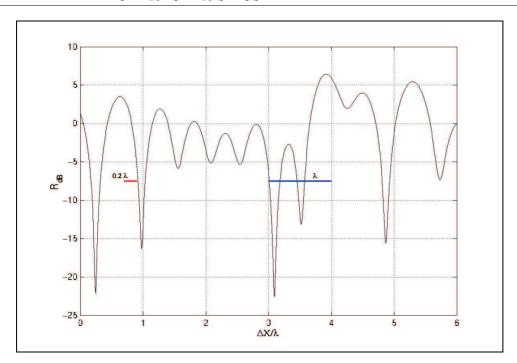
Figure B.1: Fast fading in relation with the TTI size.
