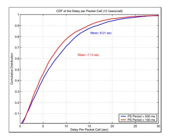
Figure 5.15: CDF of the delay per packet call, for the cases the packet scheduling period is 500 and 100 ms (12 UEs per cell, traffic model scenario B).
