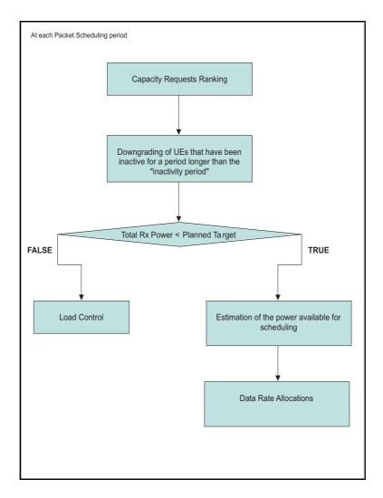
Figure 4.6: Functioning of the PS at each packet scheduling period.
