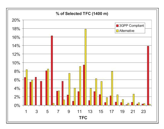
Figure 3.9: Probability of selected TFC for a distance to the Node B equal to 1400 m.
