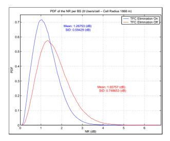
Figure 4.19: PDF of the noise rise (TFC Elimination "On" and "Off", 8 UEs per cell, cell radius 1866 m).
