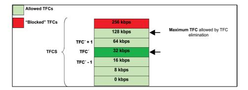
Figure 4.10: Transport Format Combination Selection Procedure.
