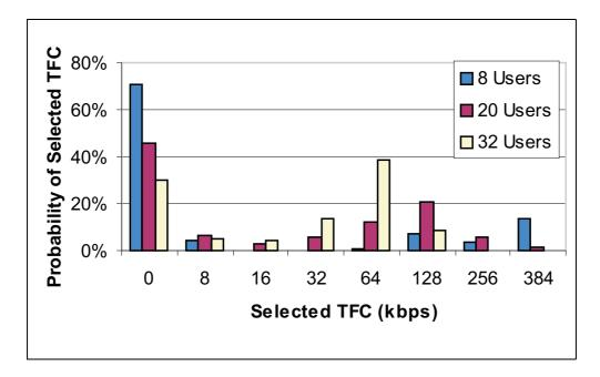
Figure 4.22: Probability of selected TFC for the cases of 8, 20 and 32 users per cell.
