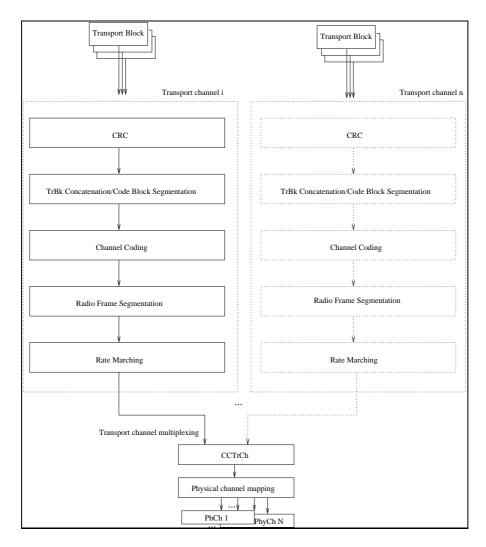
Figure 2.6: Physical layer processing model for the uplink. Model based on the one in [67].
