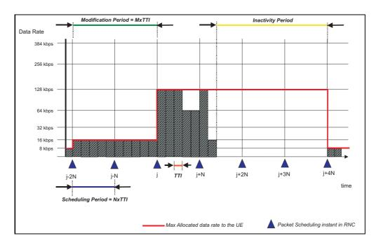
Figure 4.5: Time intervals in the packet scheduling procedure.
