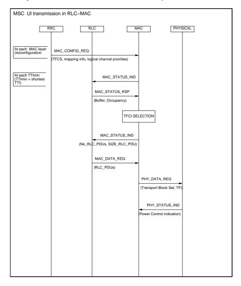
Figure 3.4: Uplink transmission in MAC layer in dedicated mode (UE side).
