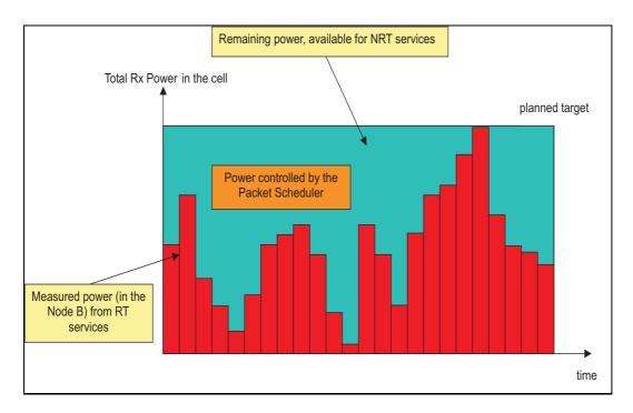
Figure 4.1: Division of the total received (Rx) power in uplink between RT and NRT traffic.
