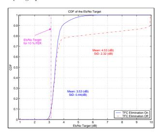
Figure 4.18: CDF of the Eb/No target (TFC Elimination Mechanism "On" and "Off", 8 UEs per cell, cell radius 1866 m).
