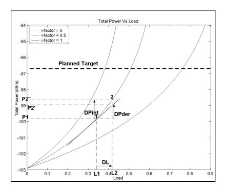
Figure 4.8: Estimation of the new total received power due to the change of the load of a user.
