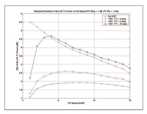
Figure B.3: Standard deviation of the UE transmission power versus UE speed for the cases the fast VSF is deactivated and activated.
