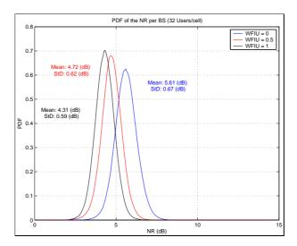
Figure 4.20: PDF of the noise rise (32 UE per cell, weighting factor for inactive users (WFIU) is set 0, 0,5 and 1 respectively).
