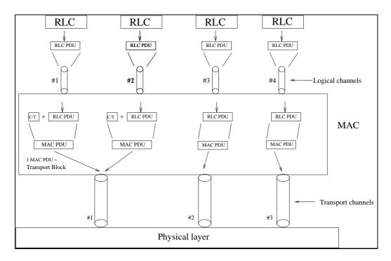
Figure 3.3: MAC protocol during uplink multi-traffic transmission. Transmission is done on dedicated logical and transport channels.
