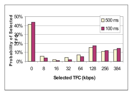
Figure 5.16: Probability of selected TFC for all of the users, for the cases the packet scheduling period is 500 and 100 ms, (columns 1 and 2 respectively, 12 UEs per cell, traffic model scenario B).
