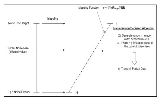
Figure 5.9: Packet data transmission mechanism in the decentralized scheme.
