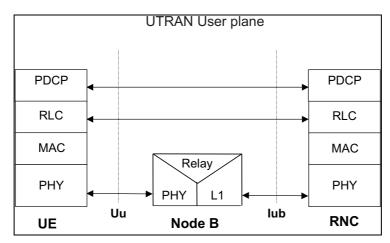
Figure 2.2: User Plane protocol stack in the case of establishment of dedicated channels between the UE and the network.
