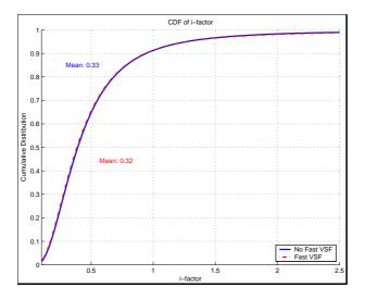
Figure 5.4: CDF of i-factor (fast VSF "On" and "Off", 12 UEs per cell, traffic model scenario B).
