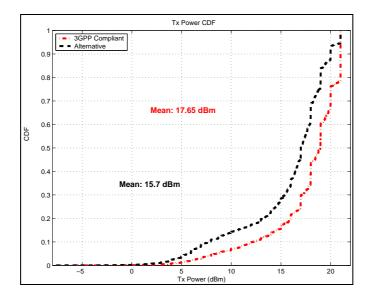
Figure 3.10: CDF of the UE transmission power for a distance to the Node B equal to  $1400~\mathrm{m}.$
