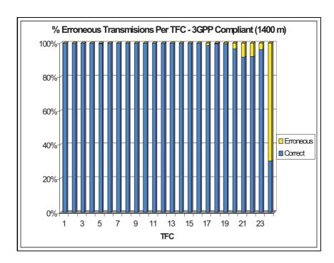
Figure 3.11: Percentage of correct-erroneous reception per selected TFC in the case of the 3GPP compliant algorithm.
