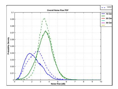
Figure 5.12: PDF of the noise rise, for the cases of the centralized and decentralized schemes.
