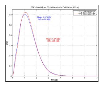
Figure 4.14: PDF of the noise rise (TFC Elimination "On and "Off", 8 UEs per cell, cell radius 933 m).
