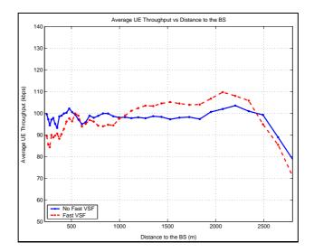
Figure 5.7: Average UE throughput during activity period (fast VSF "On" and "Off", 12 UEs per cell, traffic model scenario B).
