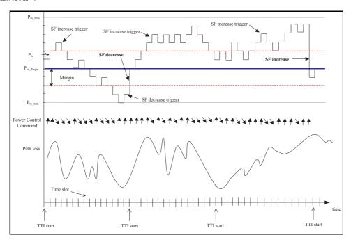
Figure 5.3: Implementation of the fast VSF scheme.
