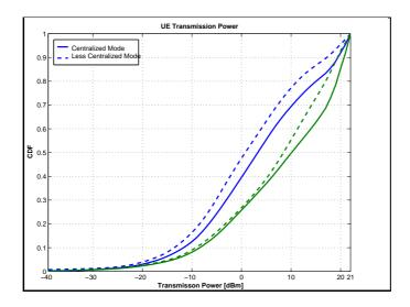
Figure 5.11: CDF of the UE transmission power, for the cases of the centralized and decentralized schemes.
