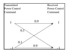
Figure A.1: Model of errors of the power control command
