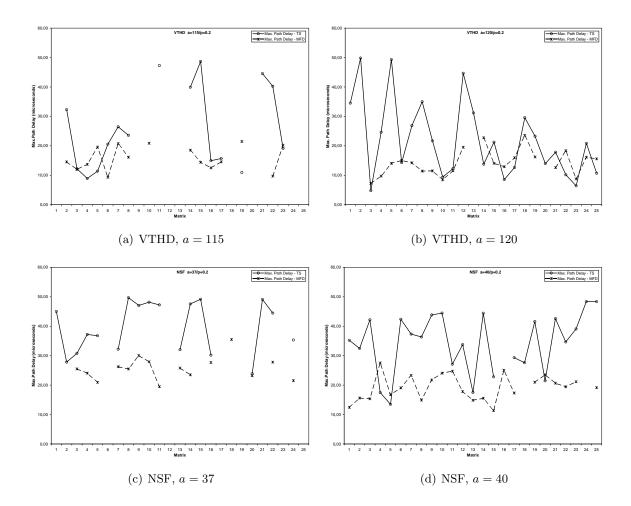
**Figure 6.5**: Maximum Path Delay in Layouts Obtained from MPSFAP1 for VTHD and NSF Network Topologies using TS and MFD Algorithms
