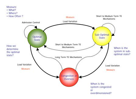
Figure 3.7: TE System and Network States
