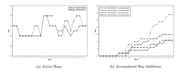
**Figure 8.1**: Used hops and accumulated hop additions for MPSFAP1 and MRPSFAP on NET2 for demand matrix series  $M_1$  using MINLP Solver (NEOS) and MFD-R Heuristic
