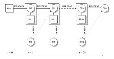
**Figure 7.4**: Overall process to compare layouts obtained from MPSFAP1 and MRPSFAP for a series from an original matrix
