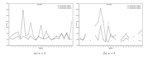
Figure 4.4: Average End-to-end Path Delay for NET1
