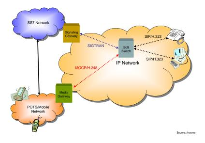
Figure 2.2: NGN Simplified Control Architecture
