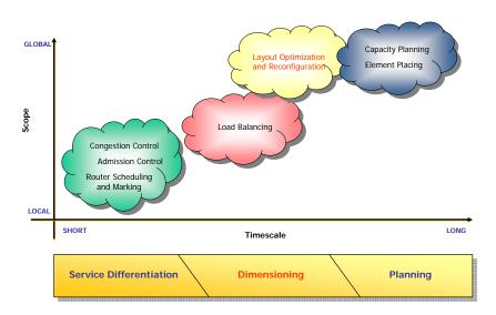
Figure 3.3: TE Mechanisms and Their Relationship to Timescales
