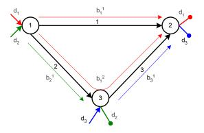
Figure 4.2: Example on the importance of avoiding path-delay constraints on unused paths
