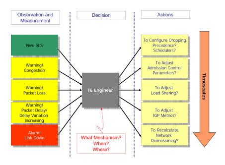
Figure 3.1: The Traffic Engineer and Timescales
