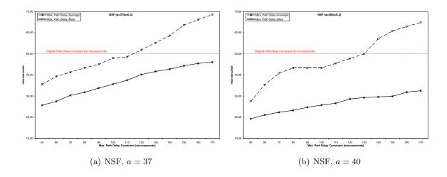
**Figure 6.7**: Maximum Path Delay and Average Maximum Path Delay for NSF Network Topologies Using MFD Algorithm, as a Function of Delay Constraint
