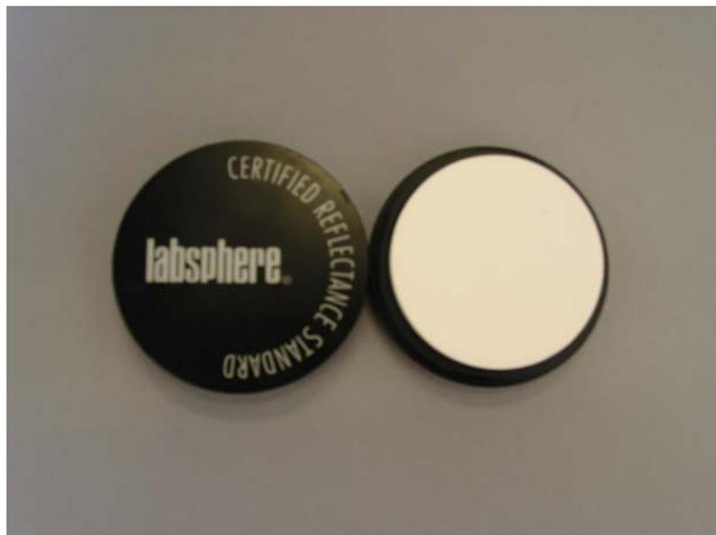
*Figure 6-29. Photograph of the calibrated white patch used in our experiments.*
