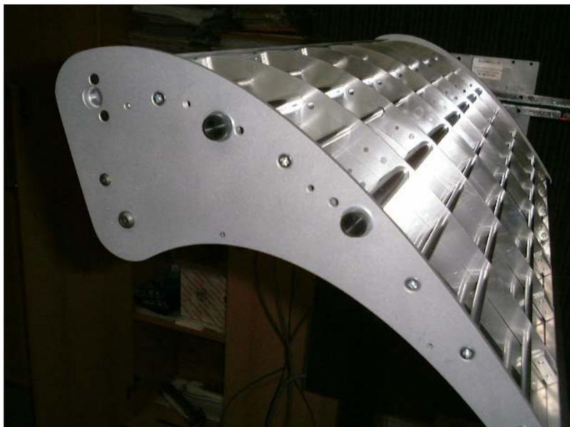
Figure 6-5 Photograph of an elliptical projector part of the CRISATEL system.
