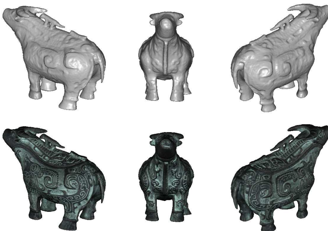
Figure 3.61: Final Buffalo model with 58734 vertices. Top: 3 shaded views. Bottom: the same views with texture mapping.
