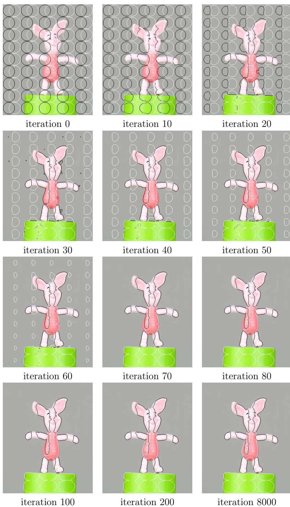
Figure A.12: 4-phase segmentation using [Vese and Chan, 2002] speed. The level sets get locked into a local minimum due to the initialization. \phi_0 and \phi_1 zero level set are drawn in black and white color, respectively.
