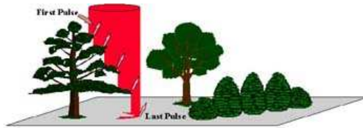
Figure 2.3: The first pulse comes from the top of the tree and the last one - from the ground (©TopoSys).
