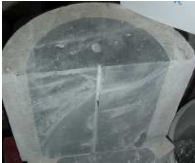
Figure I.2: A section of the composite concrete cylinder
