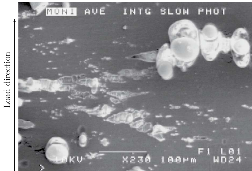
Figure 5.16: Illustration of the particle debonding and crazing for a glass bead volume fraction of 10% during an in-situ tensile test. The picture is taken for \Sigma_{11} \approx 10 MPa.
