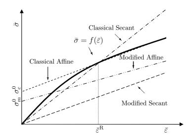
Figure 3.3: Schematic representation of the various empirical linearisation procedures expressed for the phase averages around a given reference strain level  $\bar{\varepsilon}^{\text{R}}$ . The thick line represents the actual behaviour of the nonlinear material and  $\sigma_m^0$  and  $\sigma_c^0$  are the polarisations for the modified and affine procedures, respectively.
