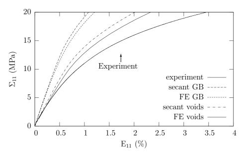
Figure 5.17: Comparison of the predictions of the secant model and the 3D FE mesh for composites with a volume fraction of 10% of glass beads (GB) and voids with experimental data for a tensile test at a uniform stress rate.
