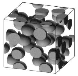
(b) FE mesh where the particles intersect with the cube sides with a periodic continuity [94]
