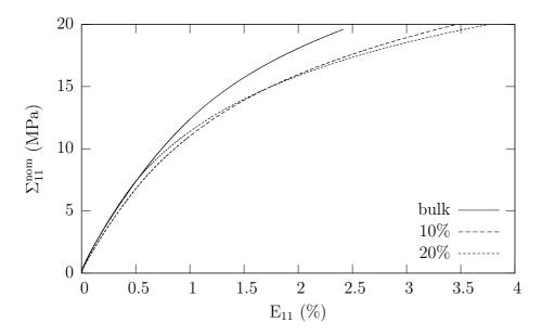
Figure 5.14: Stress/strain curves for a tensile test at a constant nominal stress rate of  $\frac{20 \text{ MPa}}{5600 \text{ sec}}$  for the bulk polypropylene as well as the 10% and 20% glass beads reinforced material.
