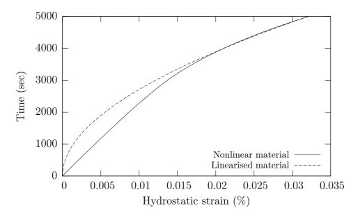
Figure 4.1: Hydrostatic component of strain associated with the secant condition for the linearised secant and nonlinear material (i.e.,  $\mathbf{J} : \hat{\boldsymbol{\varepsilon}}$  and  $\mathbf{J} : \tilde{\boldsymbol{\varepsilon}}$ ) as a function of time for  $\boldsymbol{\check{\sigma}} = \check{\sigma}_{11}(t)$
