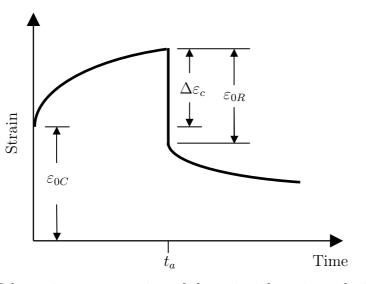
Figure 2.1: Schematic representation of the uniaxial strain evolution during a creep – recovery test
