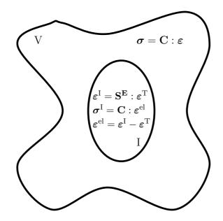
Figure 3.1: Eshelby's ellipsoidal inclusion problem [27]. An ellipsoidal subdomain I of V is subjected to a stress-free strain  $\varepsilon^{\mathrm{T}}$ . The resulting strain in the inclusion,  $\varepsilon^{\mathrm{I}}$  is given by  $\varepsilon^{\mathrm{I}} = \mathbf{S}^{\mathbf{E}} : \varepsilon^{\mathrm{T}}$ , where  $\mathbf{S}^{\mathbf{E}}$  Eshelby's tensor.
