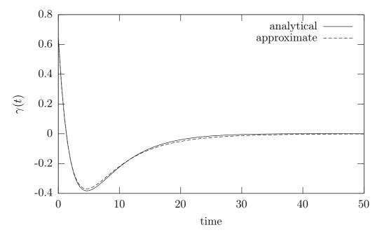
Figure 4.5: Inverse Laplace-Carson transform of  $\gamma^*$  for long elastic incompressible fibres embedded in an isotropic matrix which obeys a Zener behaviour law. The resulting material is transversely isotropic.
