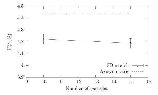
Figure 5.8: Mean value and 95% confidence interval for the macroscopic strain at 25 MPa  $\bar{E}_{11}^{25}$  as a function of the number of glass beads (10%) in the 3D meshes for a constant stress rate tensile loading and a nonlinearity factor  $\zeta = 3$ .
