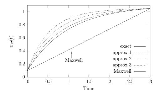
Figure 3.5: Comparison of the approximate and exact secant conditions for the shear compliance of the linear viscoelastic comparison material. The load history is a shear creep.
