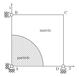
Figure 5.4: Illustration of the symmetry and periodic boundary conditions on the axisymmetric approximation of an hexagonal periodic unit cell. Symmetry conditions are applied on the sides AB and AD while periodic boundary conditions are applied on the sides BC and CD. The periodic boundary conditions impose that  $u_1$  is equal for all points on the line BC and that  $u_2$ is equal for all points on the CD line.
