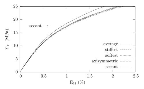
Figure 5.5: Comparison of the simulations of the secant model with the finite element simulations for a glass beads reinforced composite (10% volume fraction) under macroscopic tensile loading. The curve "softest" refers to the most compliant curve obtained with the 10 particles models and "stiffest" refers to the stiffest curve for the same type of meshes. "Average" refers to the average stress/strain curve obtained for the 10 particles models and "stiffest"
