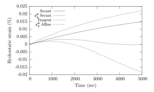
Figure 4.3: Hydrostatic components of the creep compliances and the stress free strains for the approximate secant and affine models for a reference stress history  $\breve{\sigma} = \breve{\sigma}_{11}(t)$
