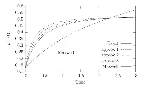
Figure 3.6: Comparison of the homogenised creep compliances  $(\tilde{\mu}^{-1}(t))$  of the linear viscoelastic comparison materials calculated in figure 3.5
