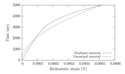
Figure 4.2: Hydrostatic component of strain associated with the tangent condition for the linearised affine and nonlinear material (i.e.,  $\mathbf{J} : \hat{\boldsymbol{\varepsilon}}$  and  $\mathbf{J} : \tilde{\boldsymbol{\varepsilon}}$ ) as a function of time for  $\boldsymbol{\check{\sigma}} = \check{\sigma}_{11}(t)$
