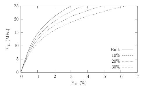
Figure 4.7: Stress-strain curves obtained for the nonlinear viscoelastic composite material for various volume fractions of spherical voids during a tensile test at a constant stress rate of  $\frac{25MPa}{7000s}$  for the secant model.
