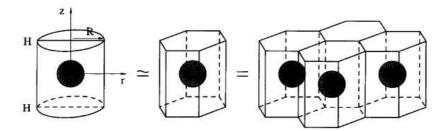
Figure 5.3: Circular base cylinder approximation of a hexagonal base cylinder periodic unit cell [61]
