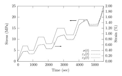
Figure 2.6: Stress history  $(\sigma(t))$  and material's response  $(\varepsilon_1(t) \text{ and } \varepsilon_2(t))$ used for the identification of the material's parameters
