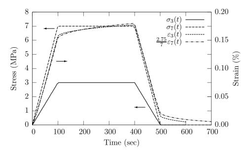
Figure 2.5: Stress histories and material responses used to determine the linear viscoelasticity domain of the polypropylene
