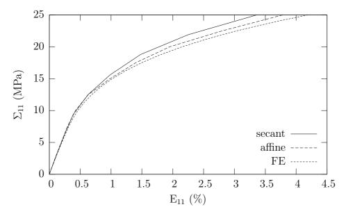
Figure 5.10: Comparison of the affine and secant models with FE simulations for a composite reinforced with glass beads and for a matrix with a nonlinearity factor  $\zeta = 3$ .
