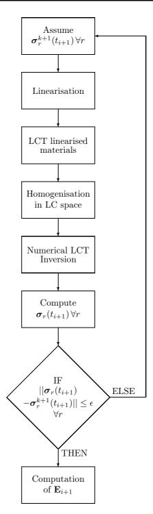
Figure 3.7: General solution algorithm for the homogenisation model during a time interval. r refers to a specific phase, LCT is the Laplace-Carson Transform and the subscript i+1 refers to the quantity evaluated at  $t = t_{i+1}$ ,  $\epsilon$ is the accuracy of the solution and k refers to the  $k^{\text{th}}$  iteration. This algorithm is repeated for  $i = 1 \dots a - 1$ .
