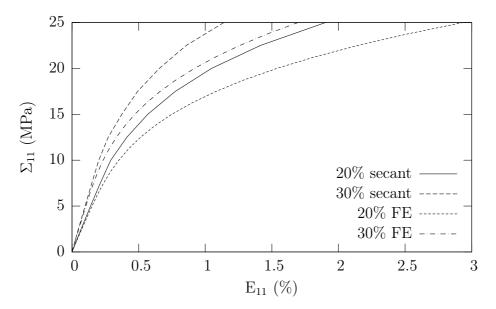
Figure 5.13: Comparison of the predictions of the secant model with FE similuations for 20% and 30% volume fraction glass beads for a nonlinearity factor  $\zeta = 3$
