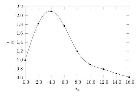
Figure 2.2: Values of  $\frac{1}{g_3}$  calculed by Lai and Bakker [48] for creep–recovery tests treated individually
