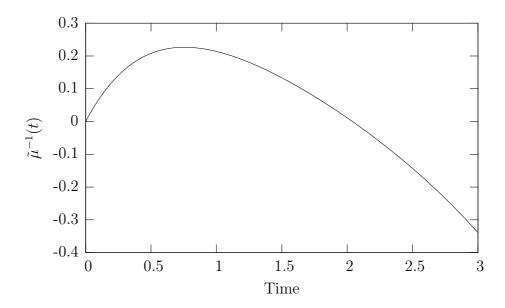
Figure 3.2: Homogenised shear creep compliance (denoted by  $\tilde{\mu}^{-1}(t)$ ) of a two phase composite material where the reinforcements are spherical and where the matrix and the reinforcements obey a Maxwell law. All the material parameters, except the viscous shear compliance of the matrix, are positive.
