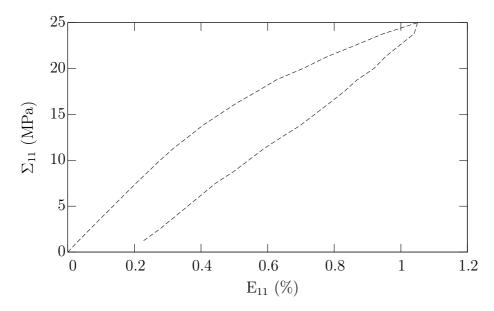
Figure 4.9: Stress-strain curves obtained for the nonlinear viscoelastic composite material for 20% of glass beads for a tensile loading-unloading test at a constant stress rate for the secant model.
