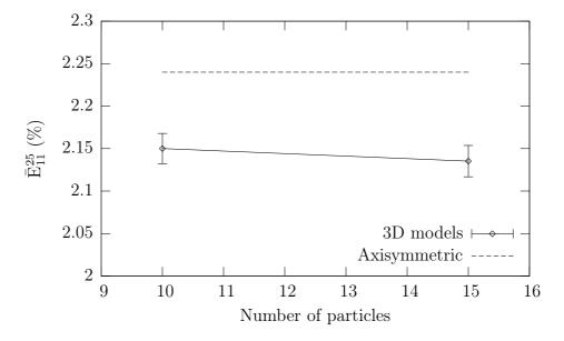
Figure 5.6: Mean value and 95% confidence interval for the macroscopic strain at 25 MPa  $\bar{E}_{11}^{25}$  as a function of the number of glass beads (10%) in the 3D meshes for a constant stress rate tensile loading.
