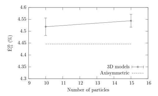
Figure 5.7: Mean value and 95% confidence interval for the macroscopic strain at 25 MPa  $\bar{E}_{11}^{25}$  as a function of the number of spherical voids (10%) in the 3D meshes for a constant stress rate tensile loading.
