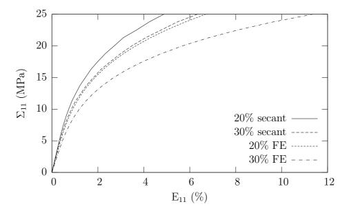
Figure 5.12: Comparison of the predictions of the secant model with FE similuations for 20% and 30% volume fraction spherical voids
