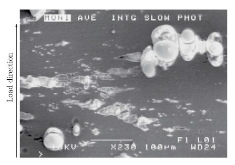
Figure 5.16: Illustration of the particle debonding and crazing for a glass bead volume fraction of 10% during an in-situ tensile test. The picture is taken for  $\Sigma_{11} \approx 10$  MPa.
