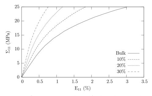
Figure 4.6: Stress-strain curves obtained for the nonlinear viscoelastic composite material for various volume fractions of glass beads during a tensile test at a constant stress rate of  $\frac{25MPa}{7000s}$  for the secant model.
