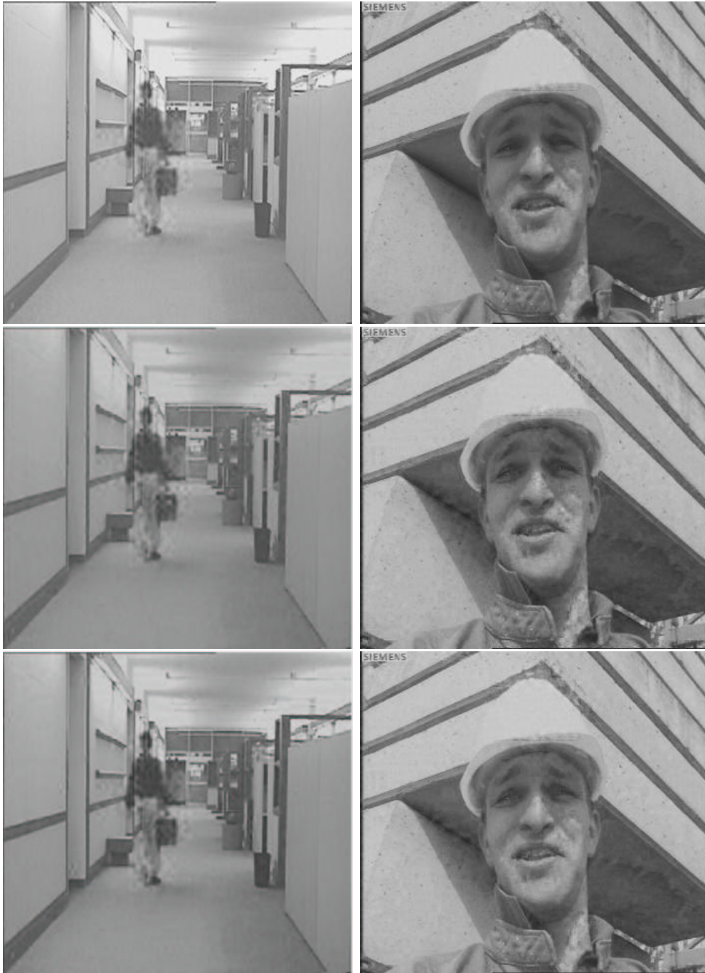
FIG. 6.6 – Reconstructed frames of "foreman" at 1104 kbs with motion estimation and "hall-monitor" at 566 kbs without motion estimation when RM is partially applied as index assignment. First line : reconstructed frames in a noiseless environment. Second line : reconstructed frames after transmission over a Gaussian channel with \text{SNR}=4.33 dB. Third line : reconstructed frames after transmission over a Gaussian channel with \text{SNR}=6.75 dB.
