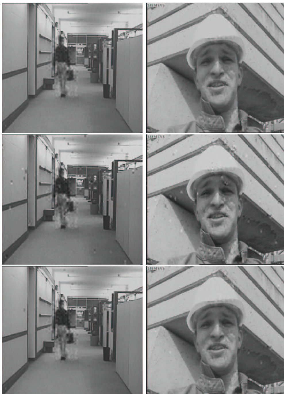
FIG. 6.5 – Reconstructed Frames of "foreman" at 1104 kbs with motion estimation and "hall-monitor" at 566 kbs without motion estimation. First line : reconstructed frames in a noiseless environment. Second line : reconstructed frames over a Gaussian channel with SNR=6.75 dB. Third line : reconstructed frames over a Gaussian channel with SNR=8.0 dB.
