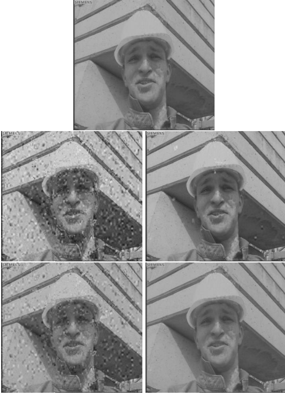
FIG. 7.6 – Reconstructed Frames. First line : reconstructed frame in a noiseless environment. Second line : reconstructed frame after transmission over a Rayleigh fading channel with \text{SNR}=9.00 dB ; Left : when no rotation matrix is used. Right : with rotation matrix prior transmission. Third line : reconstructed frame after transmission over a Rayleigh fading channel with \text{SNR}=11.00 dB ; Left : when no rotation matrix is used. Right : with rotation matrix prior transmission.
