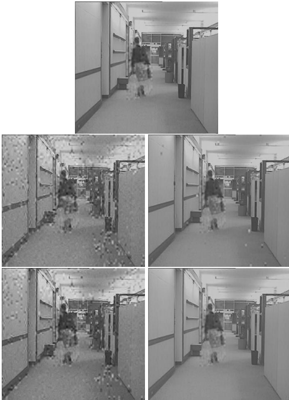
FIG. 7.5 – Reconstructed Frames. First line : reconstructed frame in a noiseless environment. Second line : reconstructed frame after transmission over a Rayleigh fading channel with \text{SNR}=9.00 dB ; Left : when no rotation matrix is used. Right : with rotation matrix prior transmission. Third line : reconstructed frame after transmission over a Rayleigh fading channel with \text{SNR}=11.00 dB ; Left : when no rotation matrix is used. Right : with rotation matrix prior transmission.
