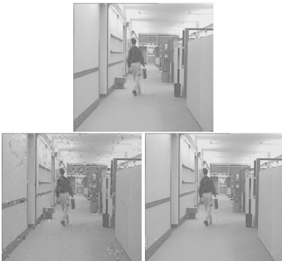
FIG. 6.4 – Reconstructed Frames. First line : reconstructed frame in a noiseless environment. Second line, left : reconstructed frame when no protection by a code is used over a Gaussian channel with \text{SNR}=4.33 dB. Second line, right : the reconstructed frame when the coarsest spatial resolution level of the temporal approximation frame is protected (Gaussian channel with \text{SNR}=4.33 dB).
