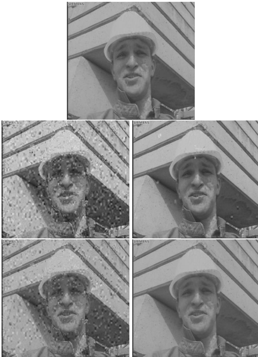
FIG. 7.6 – Reconstructed Frames. First line : reconstructed frame in a noiseless environment. Second line : reconstructed frame after transmission over a Rayleigh fading channel with SNR=9.00 dB ; Left : when no rotation matrix is used. Right : with rotation matrix prior transmission. Third line : reconstructed frame after transmission over a Rayleigh fading channel with SNR=11.00 dB ; Left : when no rotation matrix is used. Right : with rotation matrix prior transmission.
