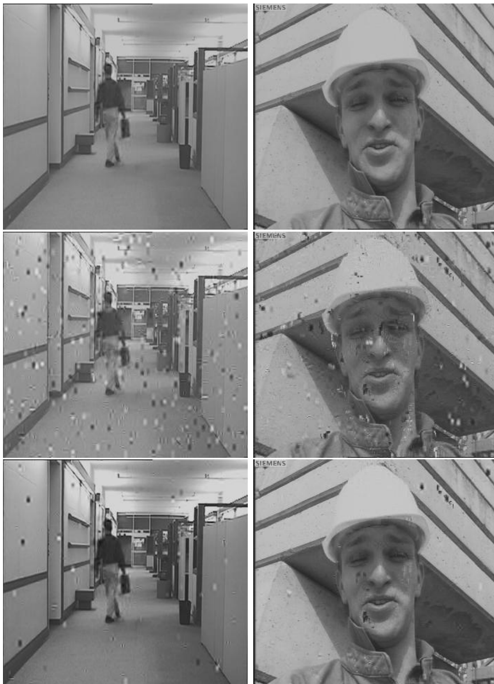
FIG. 6.7 – Reconstructed Frames of "foreman" at 1104 kbs with motion estimation and "hall-monitor" at 566 kbs without motion estimation using GLA and minimax index assignment. First line : reconstructed frames in a noiseless environment. Second line : reconstructed frames after transmission over a Gaussian channel with \text{SNR}=4.33 dB. Third line : reconstructed frames after transmission over a Gaussian channel with \text{SNR}=6.75 dB.
