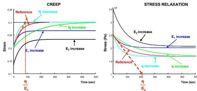
**FIGURE 1** – Influence of  $E_1$ ,  $E_2$  and  $\eta$  fluctuations on creep and stress relaxation responses, based on a reference curve; initial slopes can graphically lead to characteristic times  $\eta/E_1$  and  $\eta/E_2$ .
