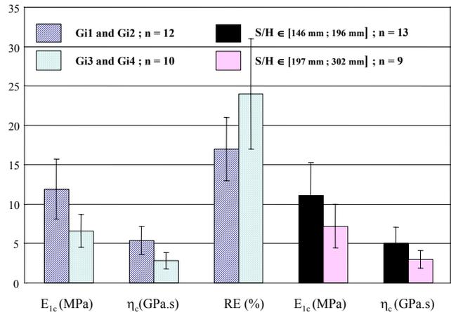
FIGURE 5 – Influence of degeneration (MRI grading) on creep and hysteresis parameters, and of S/H on creep parameters only (S = surface; H = disc height); mean values are presented  $\pm 1$  standard deviation; n = number of IVDs.
