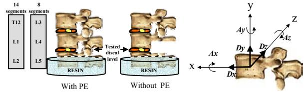
**FIGURE 1** - Specimen preparation for the mobility tests with and without posterior elements (PE); reference axis located as followed: Ax, Ay, Az = frontal, axial, sagittal rotations; Dx, Dy, Dz = postero-anterior, vertical, transverse translations.
