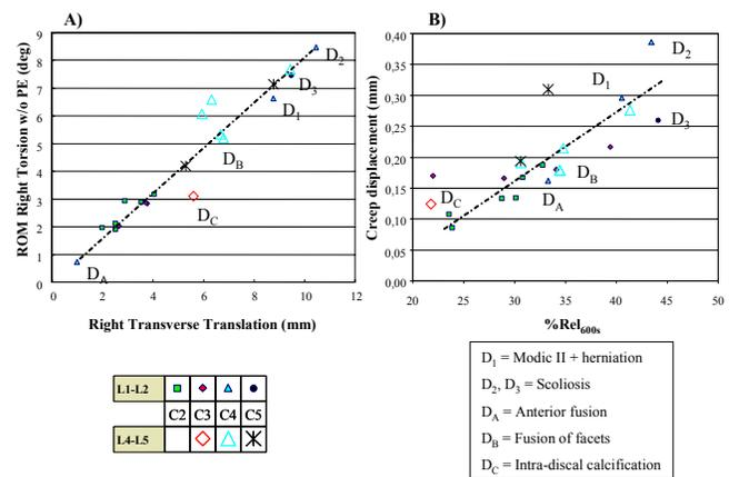
**FIGURE 5** – Correlations including the 22 lumbar discs between A) Torsion range of motion and transverse translation, and B) Creep displacement and percentage of relaxed load after 600 seconds; no IVD was outlier.
