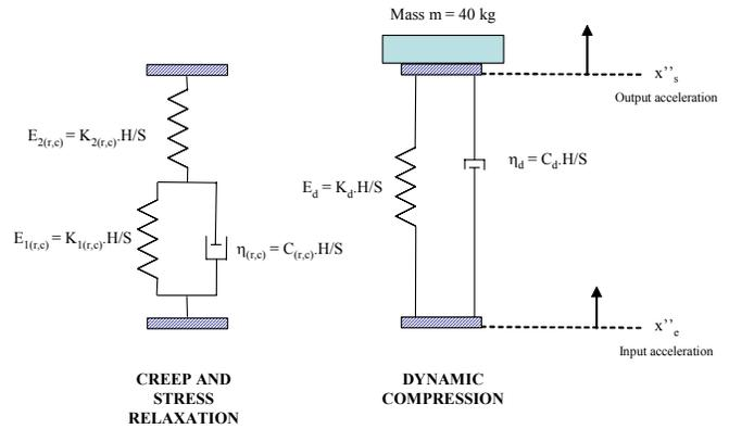
FIGURE 2 – Rheologic models of IVD using three elements ( $E_{1c}, E_{2c}, \eta_c$ ) for creep, three elements ( $E_{1r}, E_{2r}, \eta_r$ ) for stress relaxation, and two elements ( $E_d, \eta_d$ ) for dynamics;  $K_{1c}, K_{1r}, K_{2c}, K_{2r}$ , and  $K_d$  are the stiffness of the associated springs;  $C_c, C_r$ , et  $C_d$  are the damping values;  $H$  et  $S$  are the disc height and cross-sectional area, respectively.
