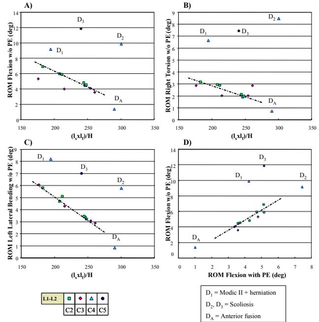
**FIGURE 4** – Ranges of motion (ROM) without (w/o) posterior elements (PE) versus  $(l_s \times l_f)/H$  for the 14 L1-L2 IVDs in A) flexion, B) right torsion and C) left lateral bending; D) ROM in flexion with PE versus w/o PE; H = disc height;  $l_s, l_f$  = sagittal and frontal diameters; D<sub>1</sub>, D<sub>2</sub> and D<sub>3</sub> are always outliers.
