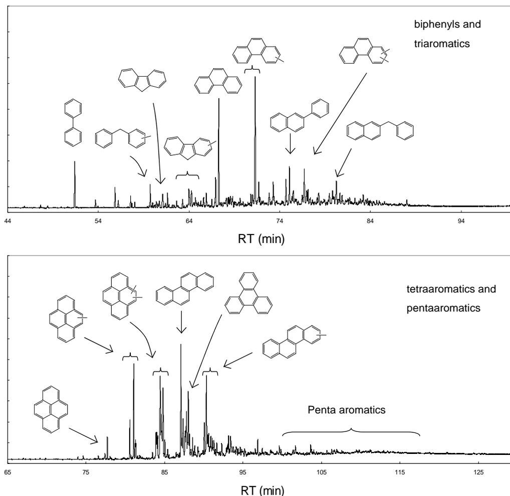
Figure III.11. GC traces of the  $C_{14+}$  pentane-soluble sub-fractions separated by HPLC (450 °C/16 h experiment).
