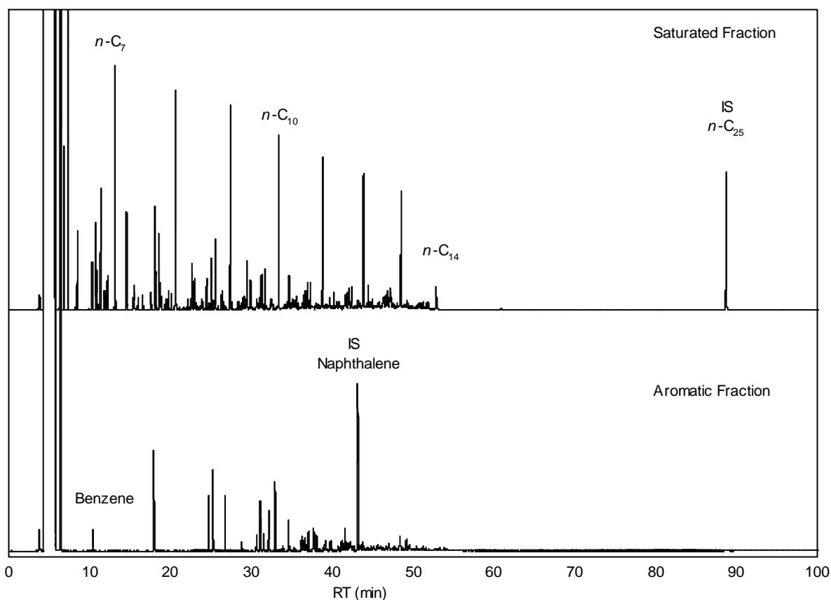
Figure II.4. Chromatogram of the saturated and aromatic fractions of Safaniya 250. cut separated on mini-column (GC-FID on HP5 capillary column-conditions as in §II.1).
