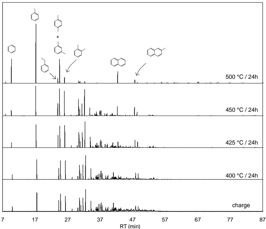
Figure III.4. GC trace of the charge and of the pentane-soluble C<sub>6</sub>-C<sub>14</sub> pyrolysis products obtained for some of the temperature screening experiments
