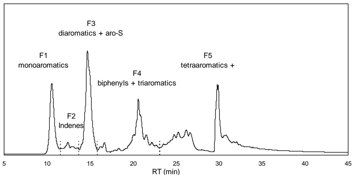
Figure III.3. HPLC separation of pentane-soluble pyrolysis products.
