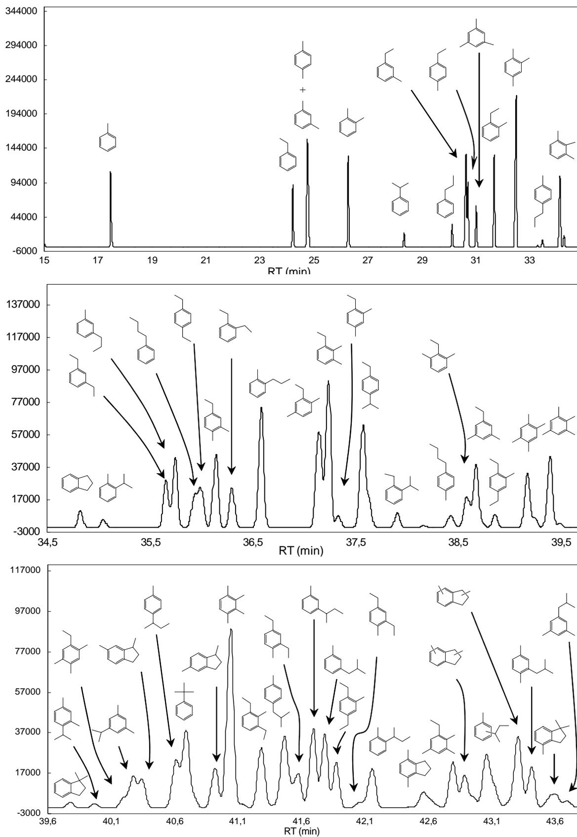
Figure II.7-a. Chromatogram of the monoaromatic sub-fraction of Safaniya 250. cut (first part of the chromatogram)
