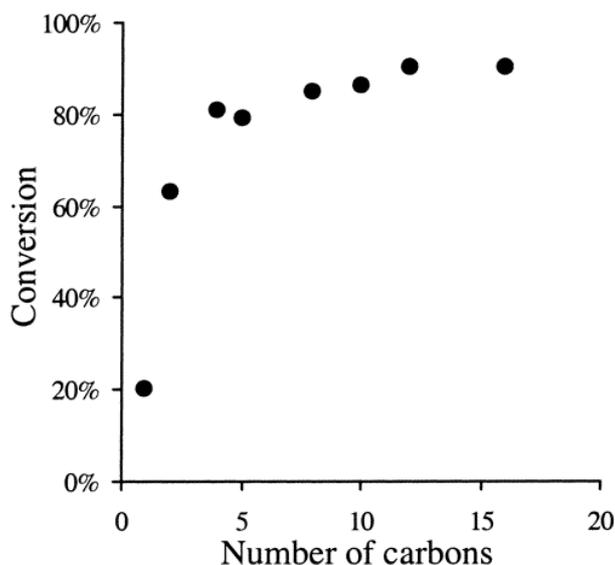
Figure III.16. Influence of the alkyl chain length on the thermal stability of monoalkylaromatics (after Smith and Savage 1991)
