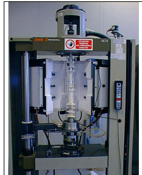
Figure IV-23: Opened Pyrox Furnace.
