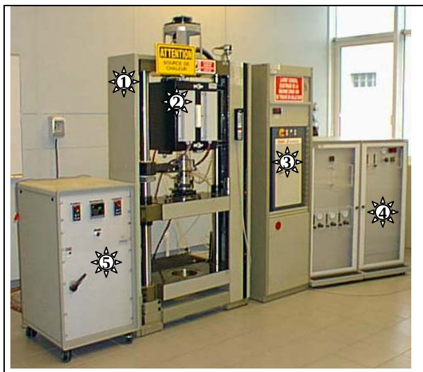
Figure IV-21: General presentation of the Zwick 1474 machine.
