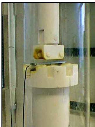
Figure IV-24: Specimen installation in the silica tube.
