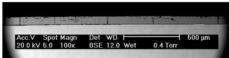
Figure IV-47: Micrograph of ReP specimen cross-section: defl: 3mm – 1mm/min – oxide: 70 \mu m – 1000°C.
