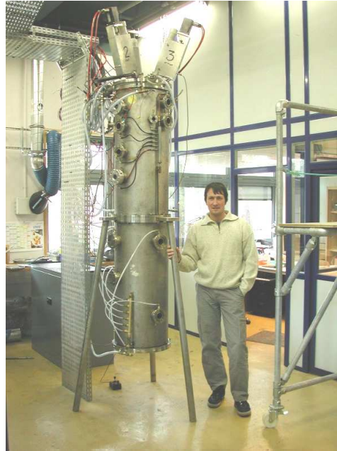
Figure IV-15 The pilot plant for the plasma process with the various sampling points in the reactor [194]
