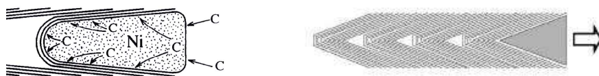
Figure V-20 Schematic representation of the proposed growth mechanism for bamboo like nanotubes (left Saïto [53] and right Okuno [215])
