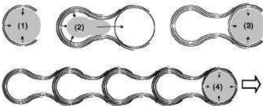
Figure V-23 Schematic representation of proposed growth mechanisms for carbon nano-necklaces. The black lines and curves represent the graphitic layers and the catalytic particle is illustrated in light grey. The small black arrows represent the pressure on the catalytic particle while the big arrow shows the direction of the motion of the catalytic particle during the growth process (Okuno - [215])
