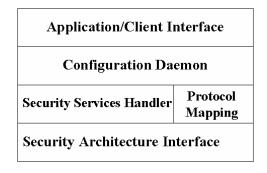
Fig 2: Security Broker Architecture
