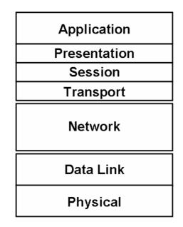
Figure 4.4: SS7 layers architecture
