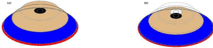
FIGURE 2.8. (a) : mode (3)  $freq_3 = 27,85 \text{ Hz}$ , (b) : mode (4)  $freq_4 = 32,69 \text{ Hz}$
