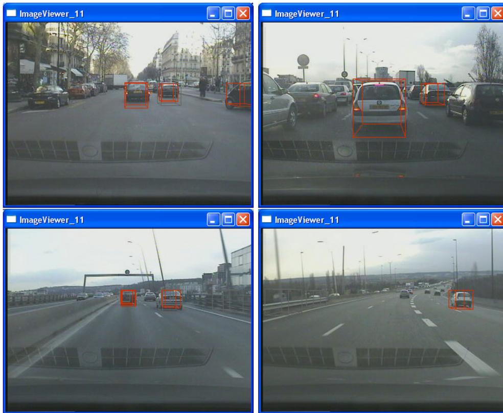
FIG. 6.31 – Successful detections in a variety of conditions.
