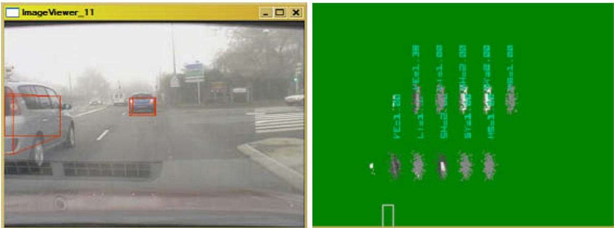
FIG. 6.4 – The likelihood function. On the left, a frontal view of a typical situation. On the right, a birds-eye view of the particles (the left "cloud" of each group) and the likelihood functions of 5 algorithms (the 5 right clouds in each group)
