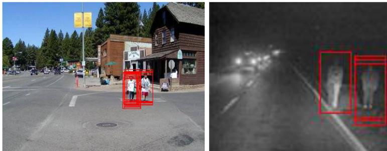
FIG. 3.18 – Successful detections in outdoor images. One can see that the feature operates equally at night and day, without any normalization of the image.
