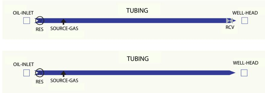
FIGURE 3.8. Block scheme of the OLGA<sup>®</sup>2000 simulation setup. First case (top) with a production choke, second case (bottom).
