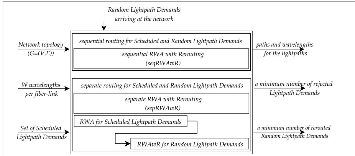
Figure 8.1 : Schematic representation of the LRR problem
