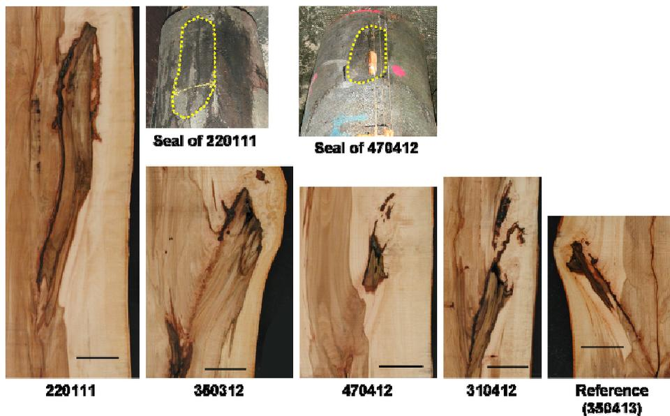
**Figure 27.** Examples of knots with very high differences between estimated and measured values, which were identified in Figure 23, Figure 24, Figure 25 and Figure 26; an example of a knot with very good correspondence of estimated and measured values is given as a reference; the length of the black line in each knot image equals 10 cm.
