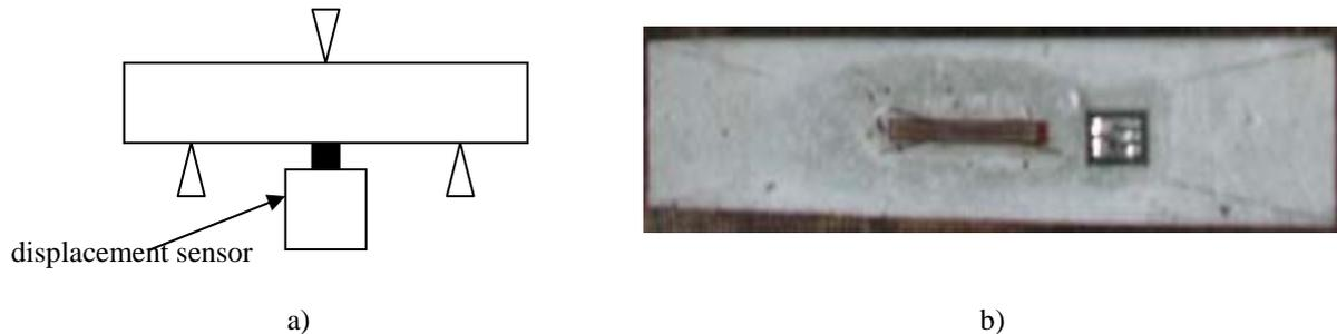
Figure 4-9.a) Displacement sensor; b) Strain gauge is located horizontally on the concrete beam for the three point bending test.
