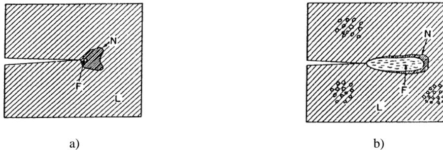
Figure 7-7. Non-linear behavior in a) brittle-ductile material, b) quasi-brittle material (concrete)
