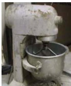
a) Small mixer to make mortar samples
