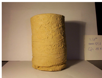
Essai No: 1, Sol 1,20m q_{cyc} = 25 \text{ kPa} \epsilon_a = 20\%
