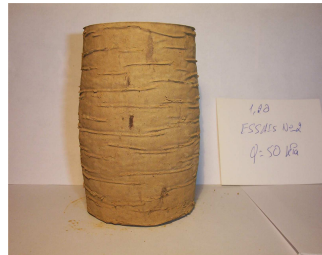
Essai No: 2, Sol 1,20m q_{cyc} = 50 \text{ kPa} \epsilon_a = 22\%
