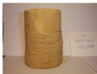
Essai No: 2, Sol 3,50m q_{cyc} = 15 \text{ kPa} \epsilon_a = 0,8\%
