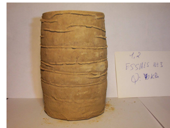
Essai No: 3, Sol 1,20m q_{cyc} = 70 \text{ kPa} \epsilon_a = 22\%
