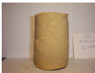
Essai No: 1, Sol 3,50m q_{cyc} = 10 \text{ kPa} \epsilon_a = 0,6\%
