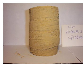
Essai No: 3, Sol 1,20m q_{cyc} = 70 \text{ kPa} \epsilon_a = 22\%
