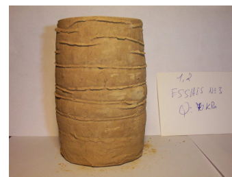
Essai No: 3, Sol 1,20m q_{cyc} = 70 \text{ kPa} \epsilon_a = 22\%
