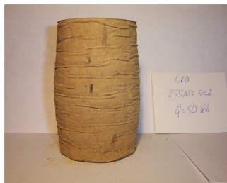
Essai No: 2, Sol 1,20m q_{cyc} = 50 \text{ kPa} \epsilon_a = 22\%
