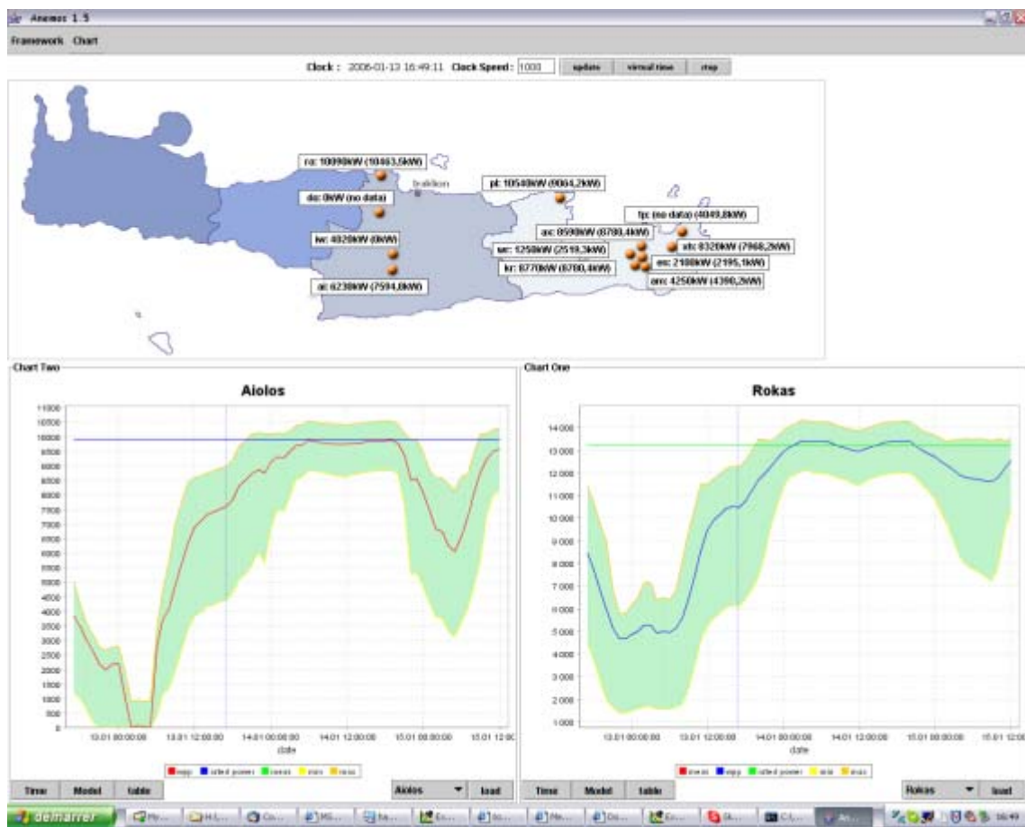
Figure C.1: The man-machine interface of the ANEMOS prediction platform for a Windows XP operating system.
