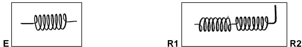
Figure 91. Scheme of the emitter coil E (left) and the receiver coils R1 and R2 connected in differential way.
