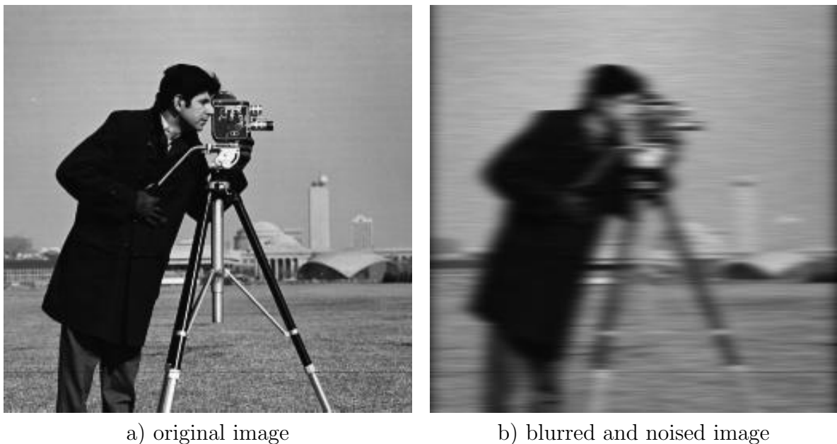
Figure 2.1: The original image a) has been blurred with an horizontal Gaussian kernel and 10% noise added, resulting in b). The goal of deconvolution techniques is to invert this degradation and recover the original image a) from b).
