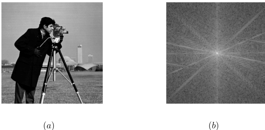
Figure 2.5: a) Original image “cameraman”, and b) its Fourier transform, log-compressed for displaying purposes.
