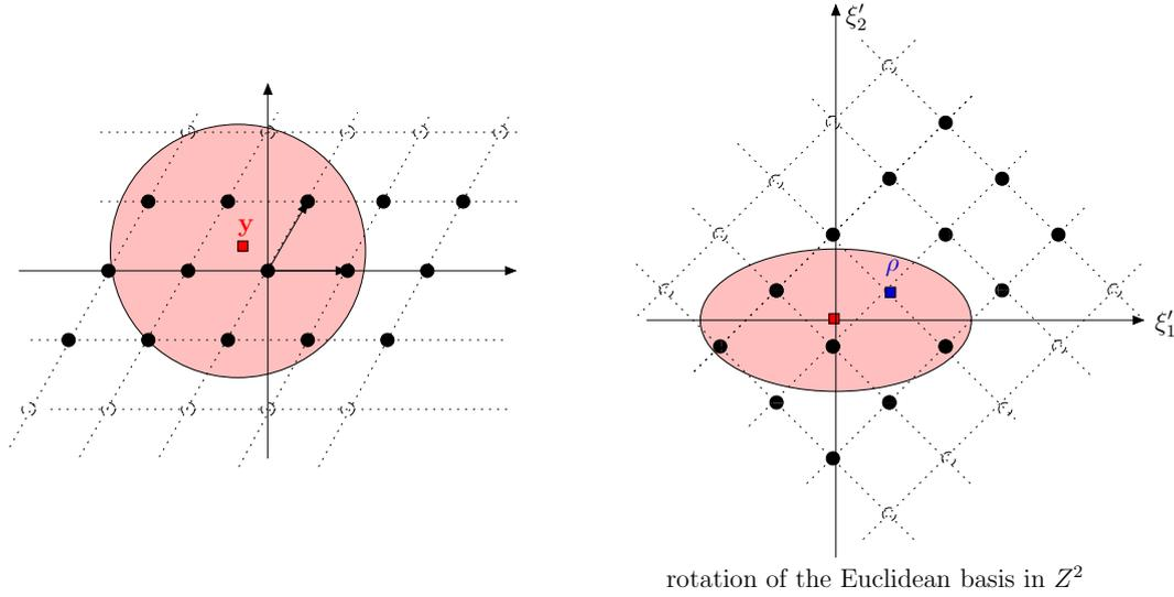
Figure 2.6: An example of a sphere decoder search in a 2-dimensional lattice code.
