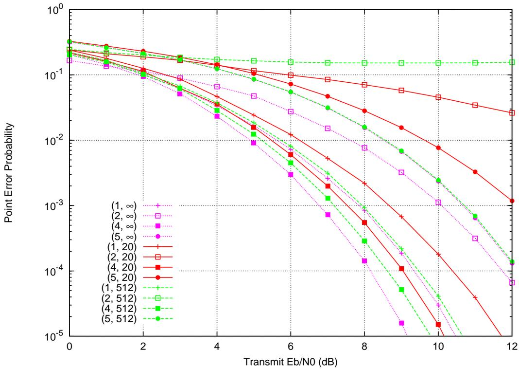
Figure 5.16: Point error rate performance for  $n = 2$  antennas using centroids for detection. Classification using geodesic metric. Components of  $\mathbf{z}$  are Gaussian integers taken from a 4-QAM constellation (uncoded).
