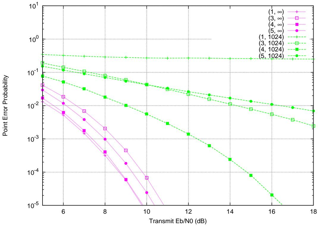
Figure 5.18: Point error rate performance for  $n = 4$  antennas using centroids for detection. Classification using geodesic metric. Components of  $\mathbf{z}$  are Gaussian integers taken from a 4-QAM constellation (uncoded).
