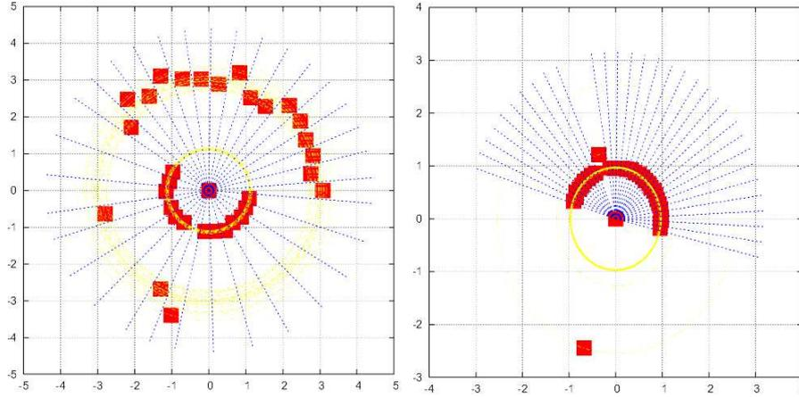
Figure 5.11: MIMO classification : Geodesic (on the left) and Frobenius (on the right) orbits for  $n = 4$  antennas, correlated & uncorrelated models,  $K = 32$  classes,  $n_L = 120$  Lloyd iterations.
