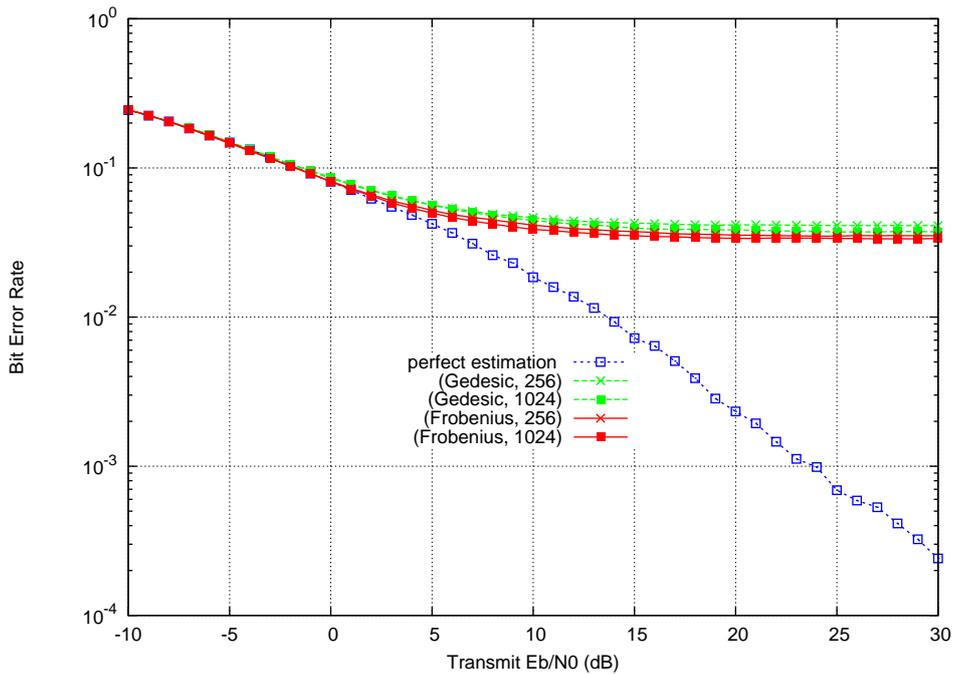
Figure 5.25: Bit error rate performance for 4 SISO channels resulting from the SVD of  $4 \times 4$  static MIMO channel using the proposed quantization approach. 4-QAM modulation applied on Tx antennas.
