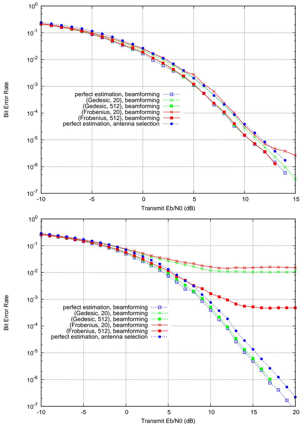
Figure 5.22: Bit error rate for the best eigen mode SISO channel resulting from the SVD of  $2 \times 2$  static MIMO channel using the proposed quantization approach for beamforming. 4-QAM modulation (on the top) and 16-QAM modulation (on the bottom) applied on Tx antennas.
