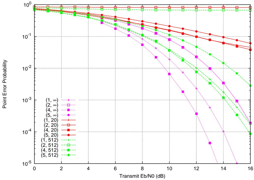
Figure 5.17: Point error rate performance for  $n = 2$  antennas using centroids for detection. Classification using geodesic metric. Components of  $\mathbf{z}$  are Gaussian integers taken from a 16-QAM constellation (uncoded).
