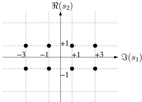
Figure 1.7: Projection of multidimensional constellation (16-QAM, 4-QAM) onto a plane.
