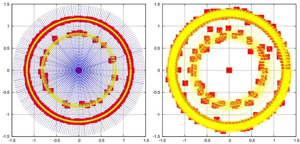
Figure 5.9: MIMO classification : Frobenius orbits for  $n = 4$  antennas, uncorrelated model,  $K = 256$  (on the left),  $K = 1024$  (on the right) classes,  $n_L = 120$  Lloyd iterations.
