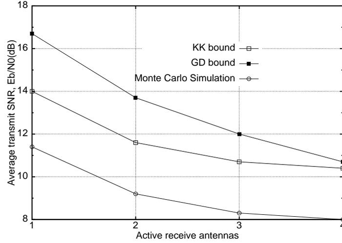
Figure 4.9: Variation of the required transmit SNR w.r.t the number of selected antennas at the receiver for an error probability =  $10^{-4}$ .
