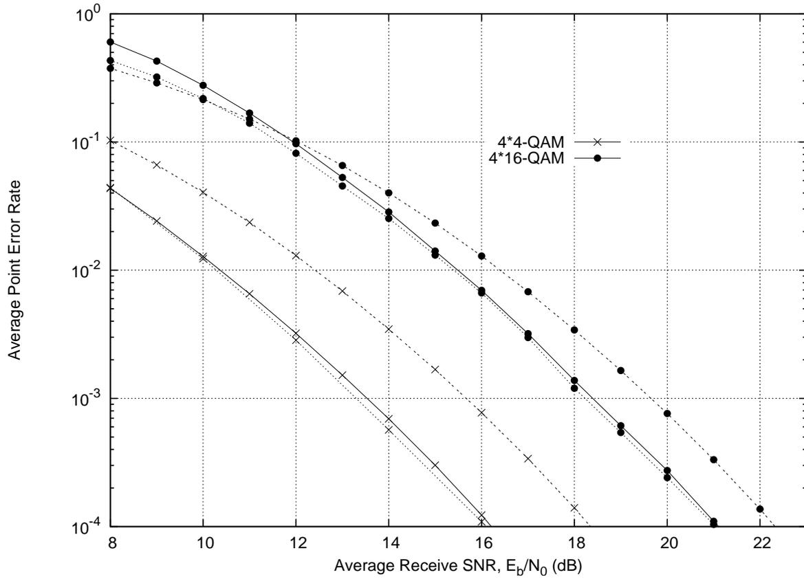
Figure 3.10: Average error probability of a  $4 \times 4$  quasi-static MIMO channel ( $T_c = 10$ ). Analytic approximation given in (3.20) based on local theta series (continuous lines), bound given in (3.4) based on minimum Euclidean distance (dashed lines), and Monte Carlo simulation (dotted lines).
