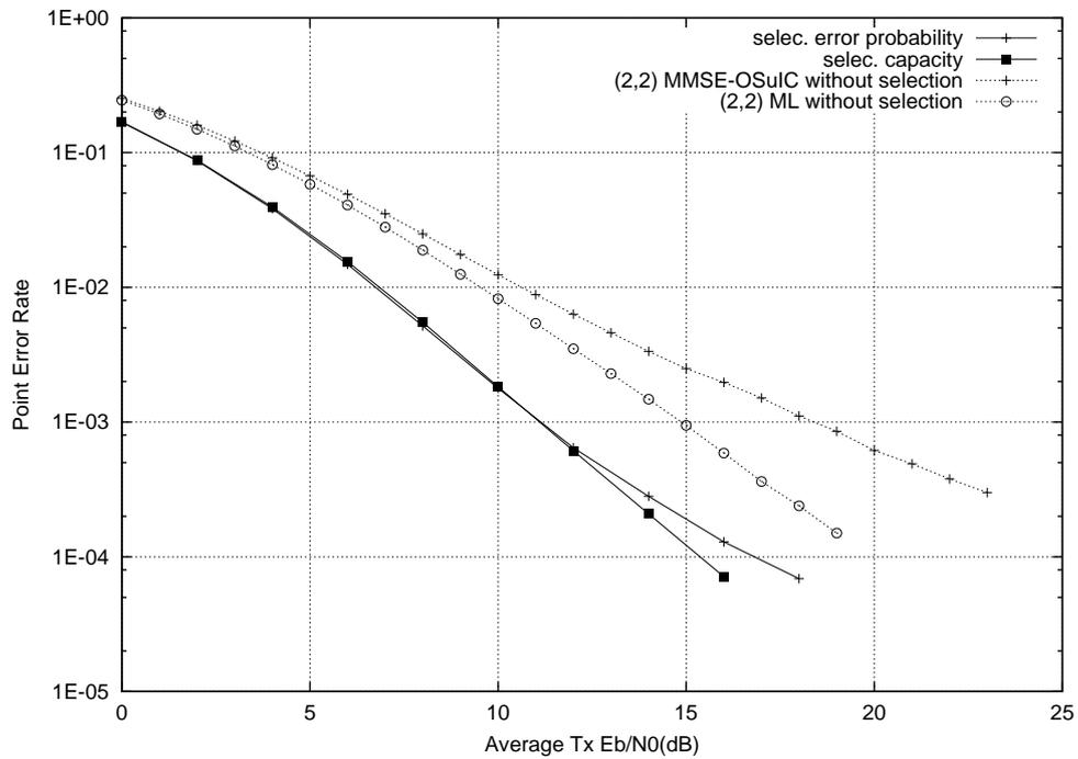
Figure 4.13: Average error probability with transmit/receive selection with MMSE-OSuIC. Select 2 antennas among 3 Tx antennas (on the top). Select 2 antennas among 3 Rx antennas (on the bottom).
