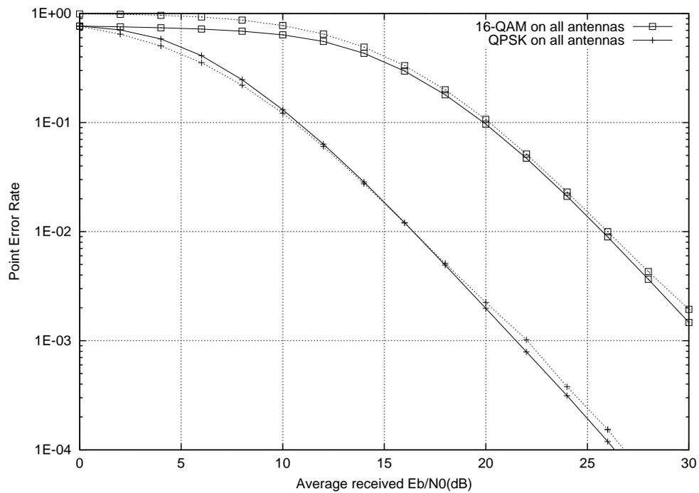
Figure 3.12: Average error probability of a  $4 \times 2$  quasi-static MIMO channel ( $T_c = 100$ ). Analytic approximation (continuous lines) and Monte Carlo simulation (dotted lines).
