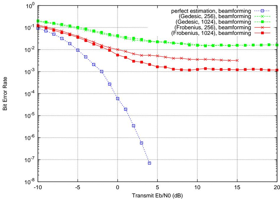
Figure 5.23: Bit error rate for the best eigen mode SISO channel resulting from the SVD of  $4 \times 4$  static MIMO channel using the proposed quantization approach for beamforming. 4-QAM modulation applied on Tx antennas.
