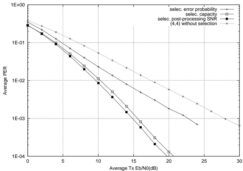
Figure 4.12: Average error probability with transmit/receive selection and MMSE receiver. Select 4 among 5 Tx antennas (on the top). Select 4 among 5 Rx antennas (on the bottom).
