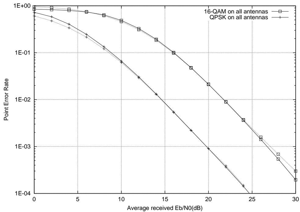
Figure 3.11: Average error probability of a  $3 \times 2$  quasi-static MIMO channel ( $T_c = 100$ ). Analytic approximation (continuous lines) and Monte Carlo simulation (dotted lines).
