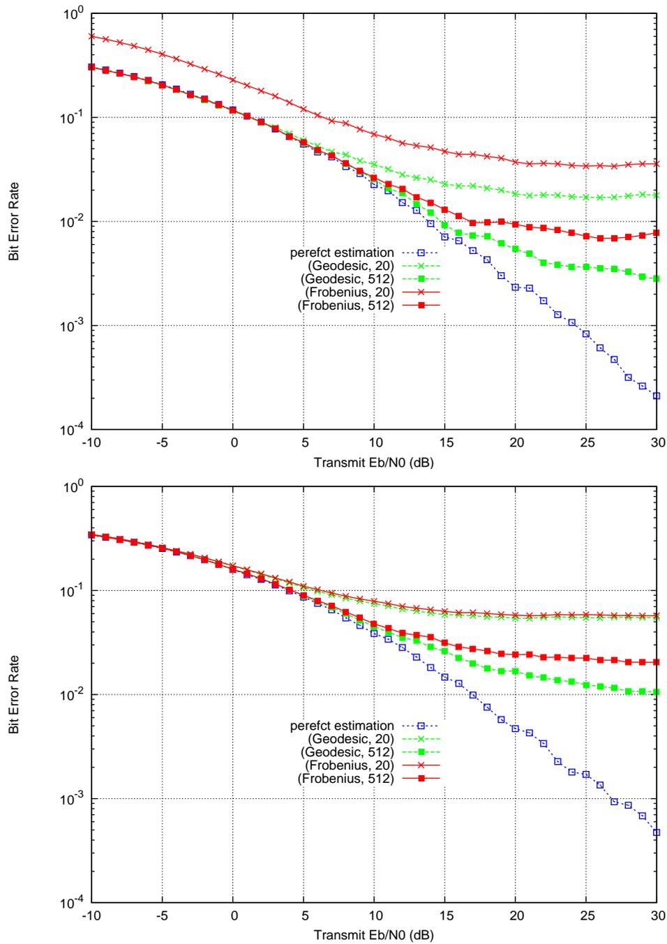
Figure 5.24: Bit error rate performance for 2 SISO channels resulting from the SVD of  $2 \times 2$  static MIMO channel using the proposed quantization approach. 4-QAM modulation (on the top) and 16-QAM modulation (on the bottom) applied on Tx antennas.
