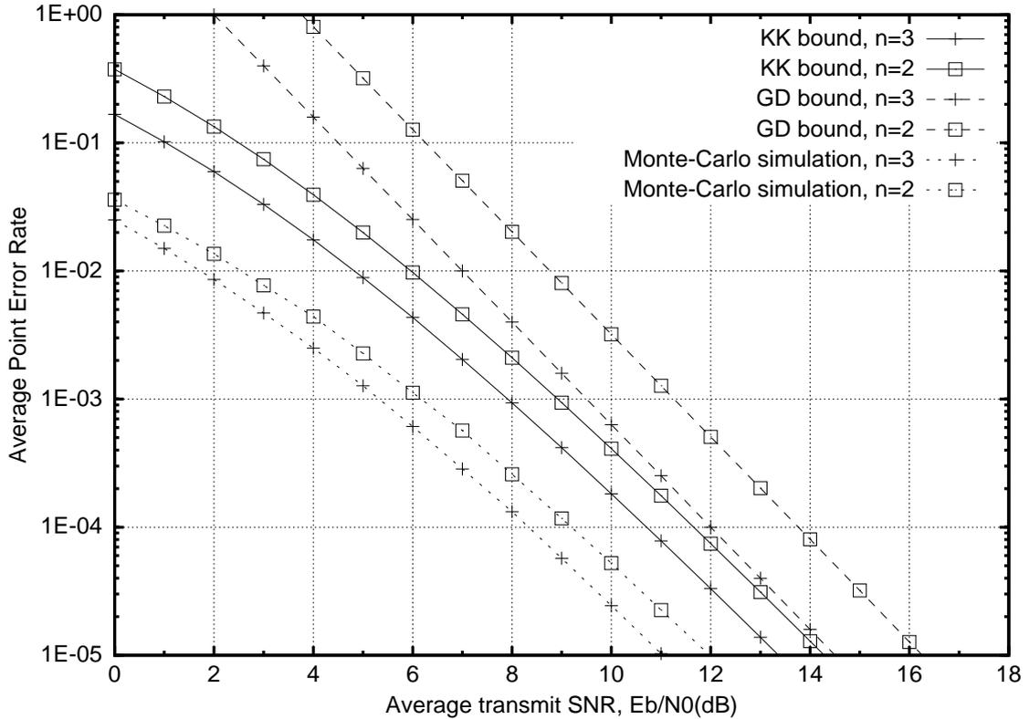
Figure 4.8: Average error probability for a  $1 \times 4$  quasi-static system with receive selection.
