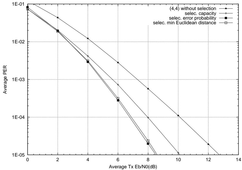
Figure 4.10: Average error probability with transmit selection and ML receiver. Select 2 antennas among 3 Tx antennas (on the top). Select 4 antennas among 5 Tx antennas (on the bottom).
