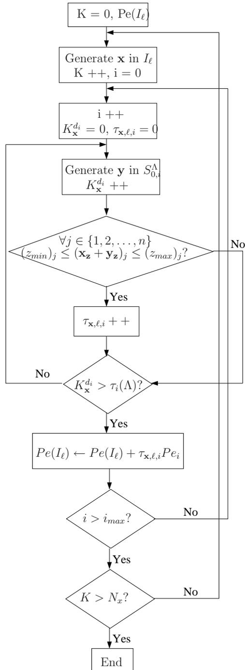
Figure 3.7: Flowchart of the algorithm used to compute the error probability  $Pe(I_\ell)$ .
