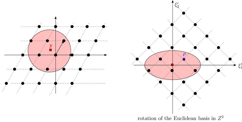
Figure 2.5: Example of sphere decoder search in bidimensional lattice.
