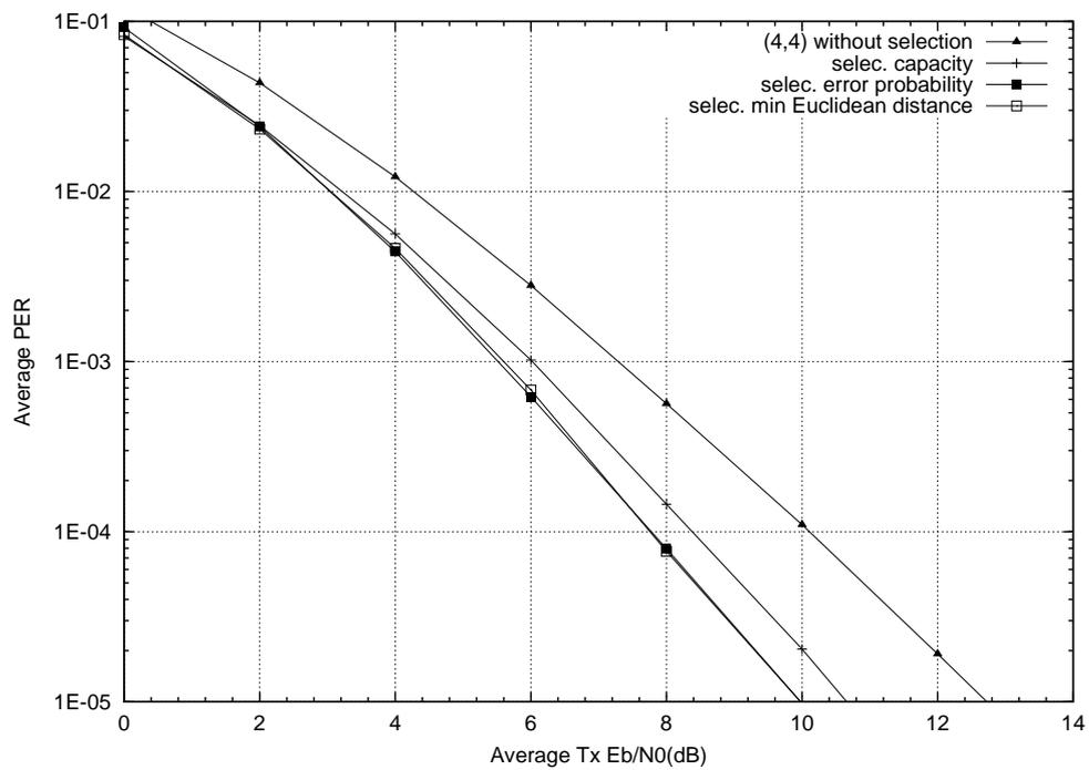
Figure 4.11: Average error probability with receive selection and ML receiver. Select 2 antennas among 3 Rx antennas (on the top). Select 4 antennas among 5 Rx antennas (on the bottom).
