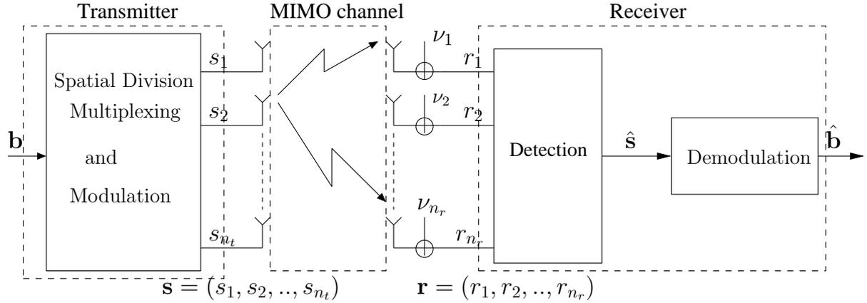
Figure 1.5: MIMO system model with spatial multiplexing.
