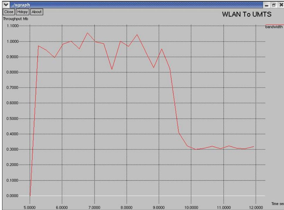
Figure 4.9 Throughput performance (WLAN/UMTS, using AVHO)
