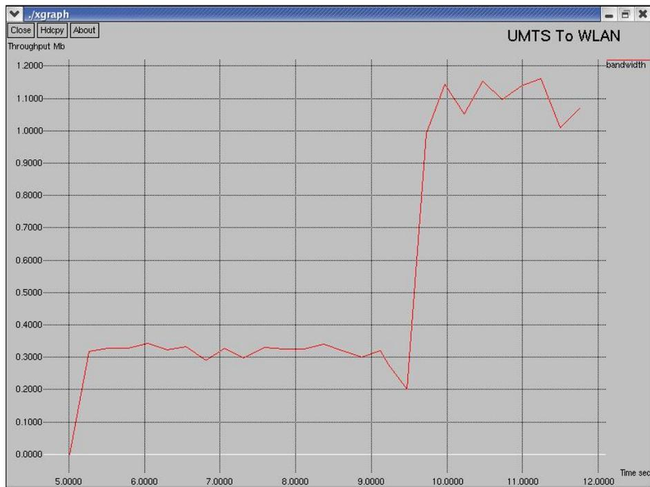
Figure 4.4 Throughput performance from UMTS to WLAN using mipv6
