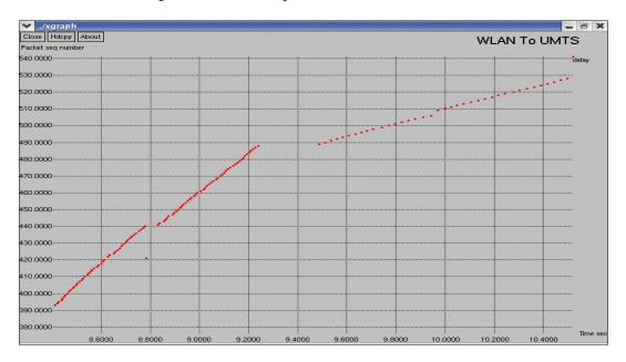
Figure 4.7 handover delay using AVHO
