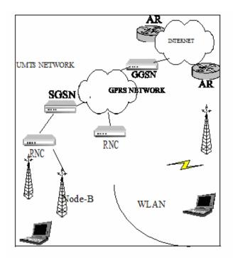
Figure 4.1 Topology of the simulated scenario
