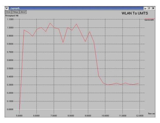
Figure 4.9 Throughput performance (WLAN/UMTS, using AVHO)
