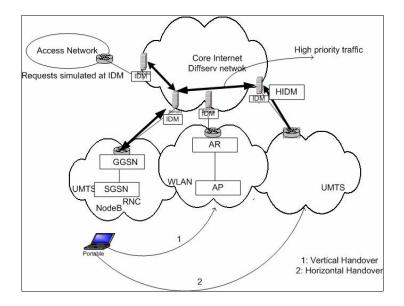
Figure 5.1 Integration Architecture with IDM
