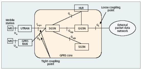
Figure 3.1 Loose and tight coupling.
