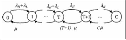
Figure 6.4 IDM model for WLAN handovers
