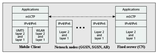
Figure 3.3 mSCTP interaction with the existing nodes
