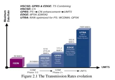
The first digital cellular system, the GSM offered a data rate of 9.6 Kbps knowing that the access scheme applied was a combination of FDMA and TDMA. Further technical
