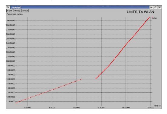
Figure 4.3 HO Delay from UMTS to WLAN using AVHO-FMIPv6
