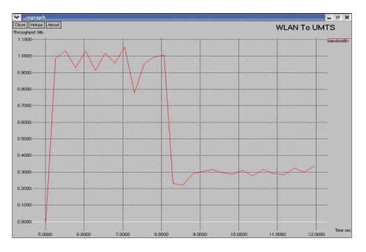
Figure 4.8 Throughput performance (WLAN/UMTS, using mipv6)
