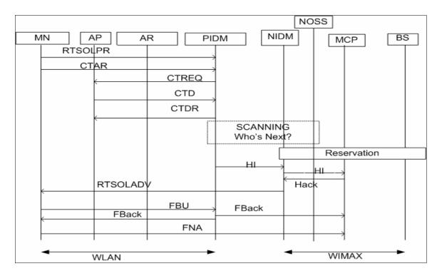
Figure 7.3 Handover from WLAN to WiMax
