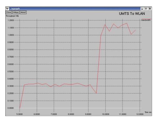
Figure 4.4 Throughput performance from UMTS to WLAN using mipv6
