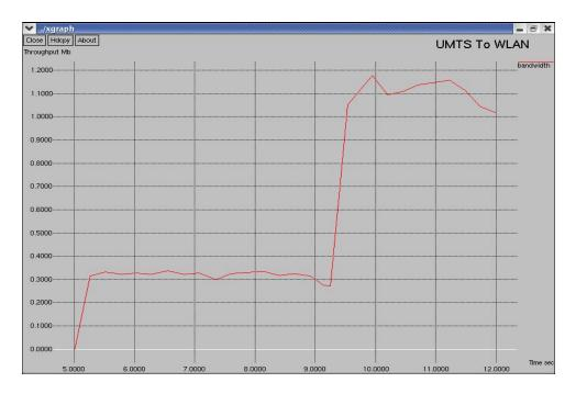
Figure 4.5 Throughput performance, from UMTS and WLAN using AVHO
