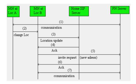
Figure 3.5 Signaling for SIP connection initialization
