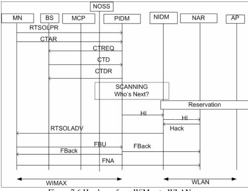
Figure 7.6 Handover from WiMax to WLAN
