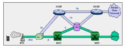
Figure 2.3 GSM/GPRS Network
