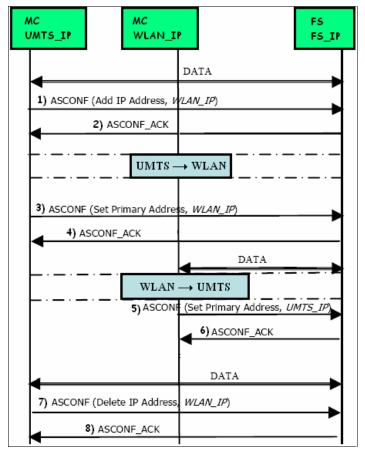
Figure 3.4 Signaling exchange for mSCTP
