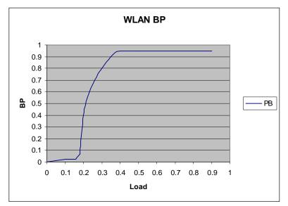
Figure 5.7 Blocking probability in function of IDM load (WLAN)
