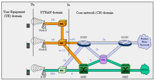
Figure 2.4 UMTS Release 99 Network
