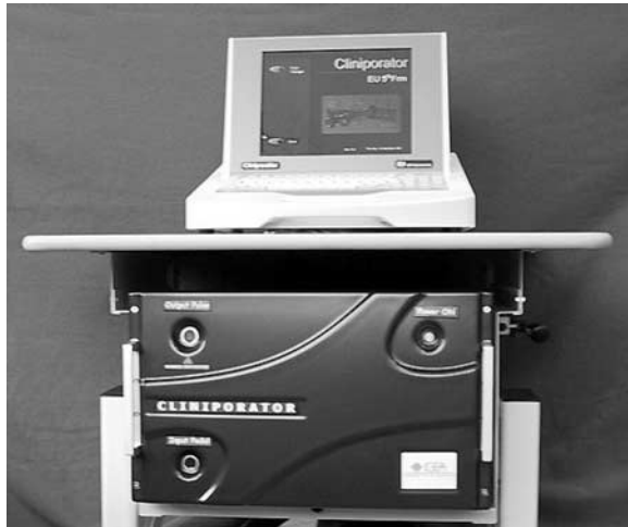
Figure 2 The Cliniporator. This new pulse generator (Cliniporator™, IGEA s.r.l., Carpi, Italy) has been developed within the Cliniporator project (QLK3-1999-00484) of the 5th Framework Program of the European Union. It delivers combinations of HV and LV pulses.
