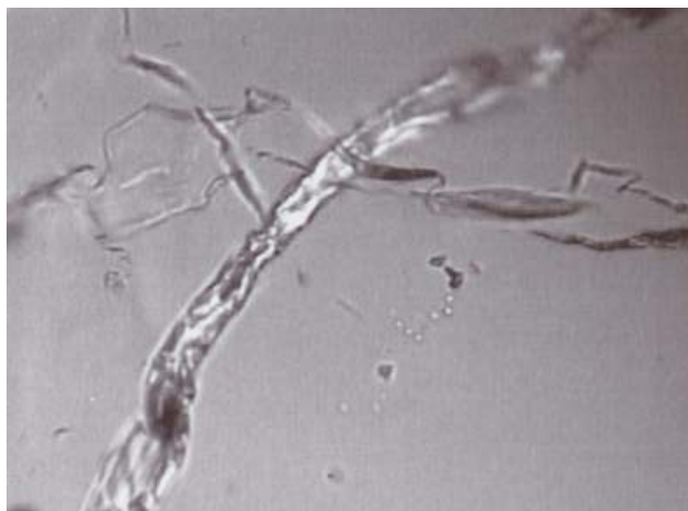
Figure 2. Borregaard fibre swollen in NMMO – water at 17% (optical microscopy in transmitted light).
