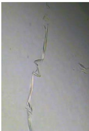
Figure 5. Unwinding step for the treated cotton and wood fibres (treated cotton fibre at a peeling rate of 10% in NMMO – water solution at 20%)
