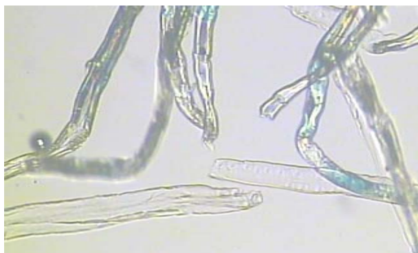
Figure 1. Homogeneous swelling of the enzymatically treated Borregard fibres with a peeling rate of 11.2%, swollen in NMMO – water at 23.5%
