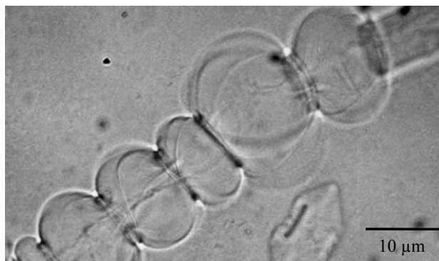
Figure 9. Regular helical ribbon in the balloons membrane (cotton swollen in NMMO – water at 20%, optical microscopy in transmitted light, T = 90°C).
