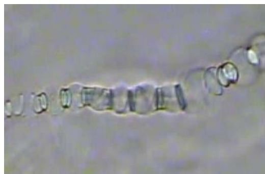
Figure 4. Swelling by ballooning. Xanthate cellulose sample (with a content of CS 2 of 35%) in NaOH (6%) – water solution, optical microscopy, T= 4°C.
