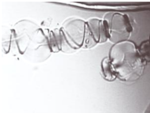
Figure 6. Swelling by ballooning in NaOH – water - ZnO solutions (Borregard fibre swollen in NaOH (7.6%) – water – ZnO (1.5%) solution, T = -5^{\circ}\text{C} , optical microscopy in transmitted light)
