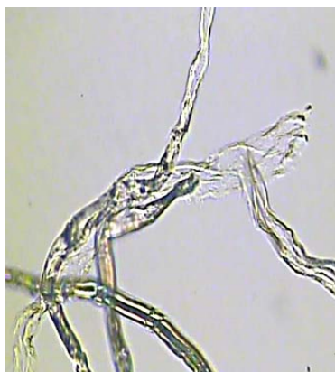
Figure 3. Separation of treated wood fibres into two sub – fibres during the swelling and unwinding step (enzymatically treated Buckeye sample at a peeling rate of 9.41%, swollen in NMMO – 20%)
