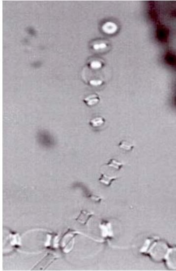
Figure 6. Swelling and dissolution mechanisms – phase 2 (cotton swollen in NMMO – water at 20%, optical microscopy in transmitted light).
