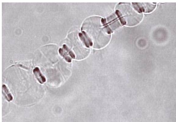
Figure 5. Swelling by ballooning in NaOH – water - urea solutions (Buckeye fibre swollen in NaOH (7.6%) – water – urea (12%) solution, T = -5^{\circ}\text{C} , optical microscopy in transmitted light)
