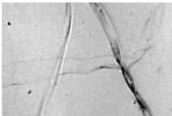
Figure 7. Treated cotton sample in ionic liquid [Bmim]Br seen by optical microscopy in transmitted light, T = 80^{\circ}\text{C}
