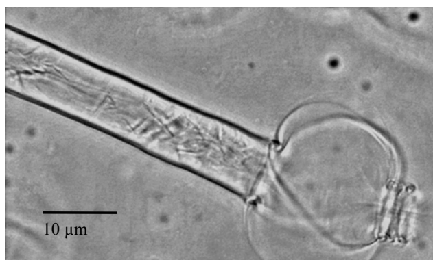
Figure 10. Regular helical ribbon in the balloons membrane (Buckeye fibre swollen in NMMO – water at 23.5%, optical microscopy in transmitted light, T = 90°C).
