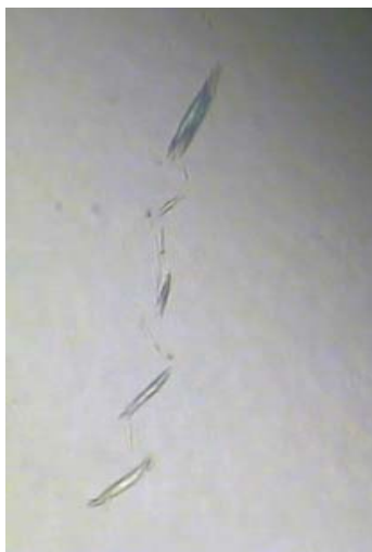
Figure 4. Dissolution by fragmentation of treated cellulose fibres (treated cotton fibre at a peeling rate of 10% in NMMO – water solution at 20%)
