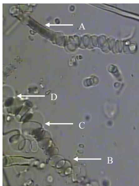
Figure 4. Swelling by ballooning, mode 2. Pulp jute in NMMO – water at 20%, T = 90°C.
