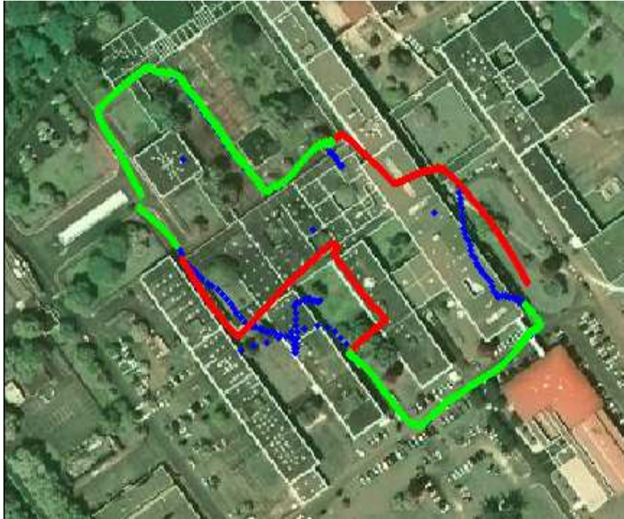
Figure 6.40: AGPS/IMU hybridisation results. Long test with corrected regression coefficients (post processing results).
