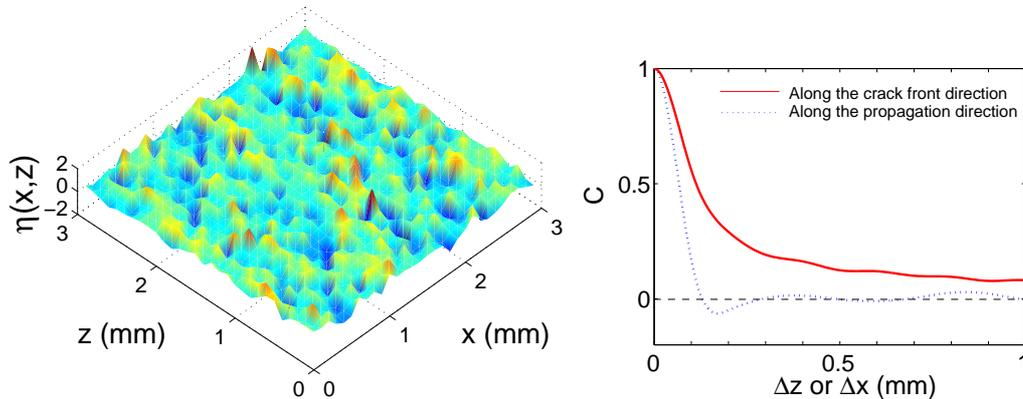
Figure 4.8: (left): 3D representation of the disorder  $\eta(x, z)$  on a fracture surface of a glass ceramics with  $\phi = 26\%$  obtained by the inverse method described in the text using Eq. (4.18). (right): The solid and dotted lines are the spatial correlation functions computed along the  $z$ -axis and  $x$ -axis respectively.
