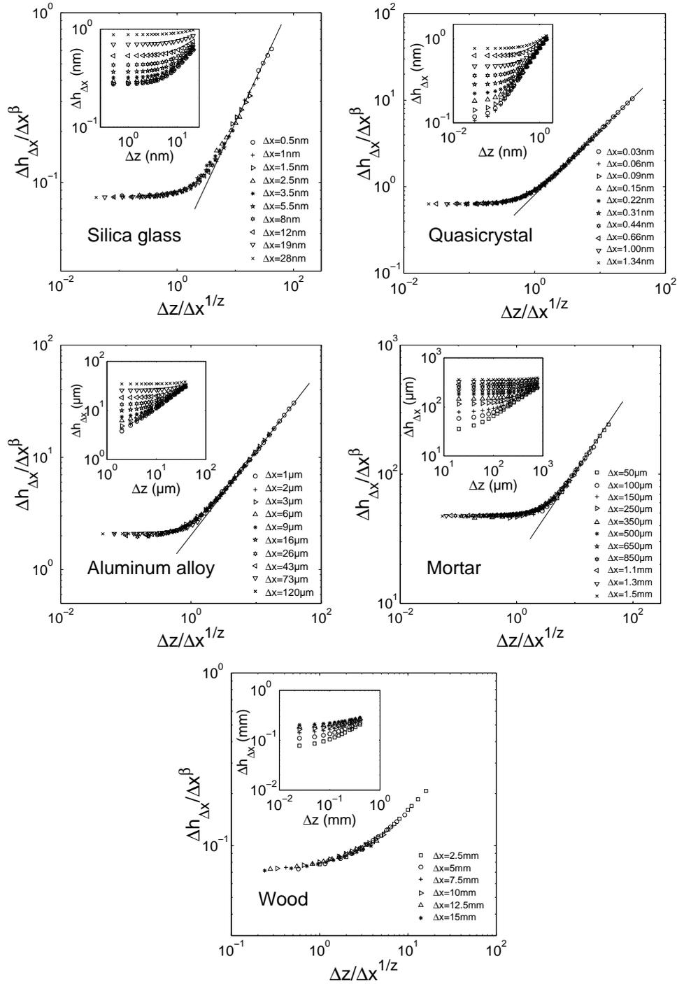
Figure 2.9: Normalized 2D height–height correlation function variations with  $\Delta z$  for various values of  $\Delta x$  for silica glass, AlPdMn quasicrystals, aluminum alloy, mortar and wood. The data collapse was obtained from Eq. (2.5) using exponents reported in Tab. 2.3.
