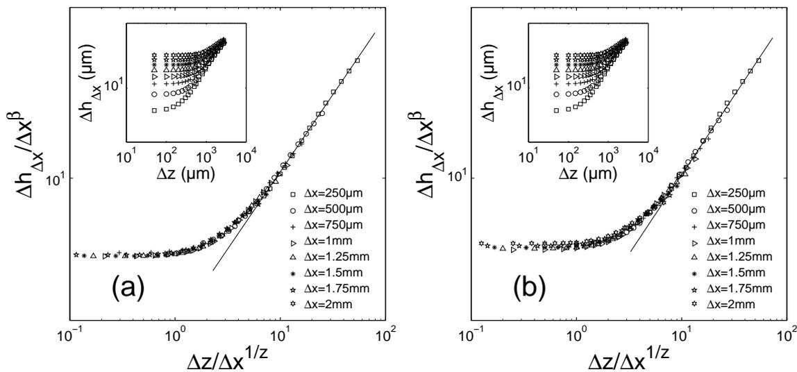
Figure 3.17: Normalized 2D variations with  $\Delta z$  of the height–height correlation function at various values of  $\Delta x$  for the surface of the fractured sandstone sample of width  $L = 14$  mm: (a)  $\beta = 0.50$  and  $z = 0.90$  are chosen to optimize the data collapse using Eq. (2.5). The straight line that corresponds to the fit of the power-law regime of the collapsing function has a slope of  $\zeta = 0.43$ ; (b) Best data collapse obtained by setting  $z = 1$ .
