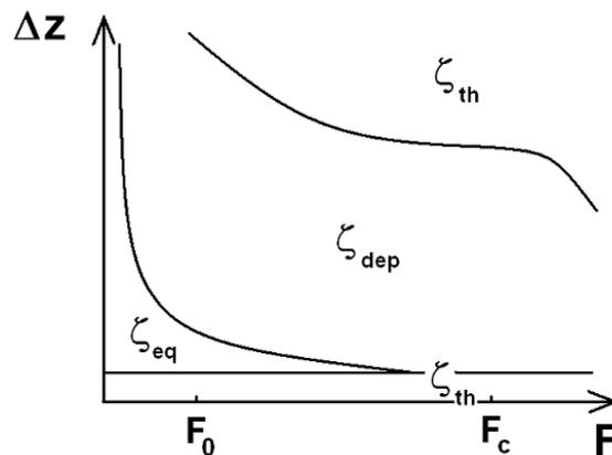
Figure 4.3: Phase diagram giving the geometry of an elastic line driven in random potential at finite temperature. The roughness exponent of the line -perpendicularly to the crack growth direction of the fracture surface - depends both on the length scale  $\Delta z$  and the driving force  $F$ . The relevant situation to predict the fracture surface morphology (Eq. (4.16)) corresponds to  $F_0 \ll F_c$ .
