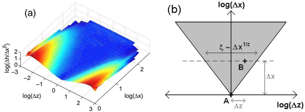
Figure 2.12: (a): 2D representation of the height–height correlation function for an aluminum fracture surface ( $\Delta h$  is normalized by  $\Delta x^\beta$  with  $\beta = 0.58$ ). (b): Domains of different types of variation of the height–height correlation function in the  $(\Delta z, \Delta x)$  plane. The grey zone corresponds to a height–height correlation function varying as  $\Delta h \propto \Delta x^\beta$ .
