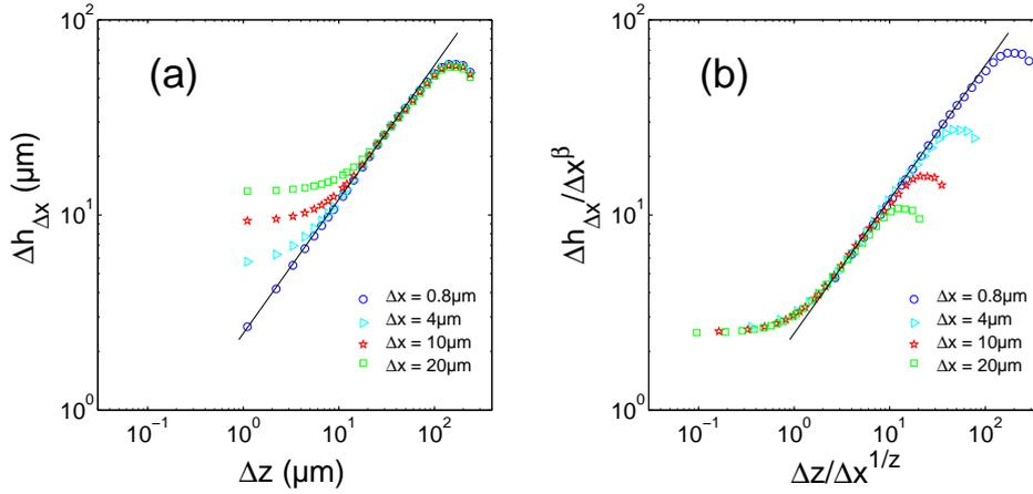
Figure 2.8: (a): 2D correlation function variations computed on a aluminum alloy fracture surface. The straight line correspond to a power-law fit with  $\zeta = 0.74$ . (b): The data collapse is obtained from Eq. (2.5) using  $\beta = 0.58$  and  $z = 1.26$ .
