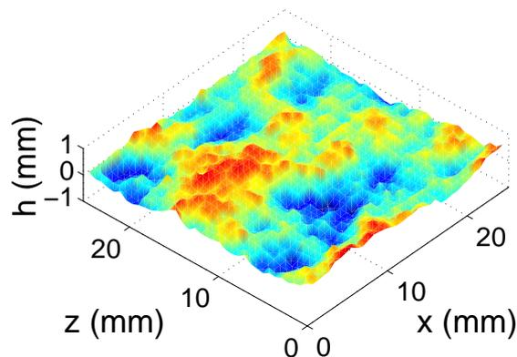
Figure 3.5: Topographic image of a fractured sandstone surface. The  $x$ -axis and  $z$ -axis correspond to the crack propagation direction and to the crack front direction, respectively.
