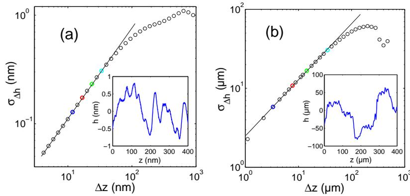
Figure 2.2: Height–height correlation function computed on profiles extracted along the  $z$ -axis of fracture surfaces of silica glass (a) and aluminum alloy (b). The straight lines correspond to power-law fits  $\sigma = \ell_z^{1-\zeta} \Delta z^\zeta$  with  $\zeta = 0.81$ ,  $\ell_z = 0.58$  fm (a) and  $\zeta = 0.74$ ,  $\ell_z = 14$   $\mu\text{m}$  (b).
