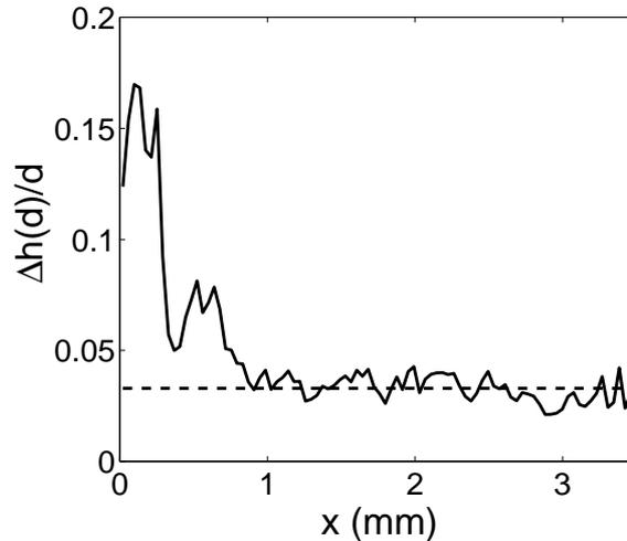
Figure 3.9: Variations of the roughness characteristic exponent  $\zeta$  and amplitude  $\Delta h(d)$  with the distance  $x$  to the initiation notch for the same sample ( $\phi = 3\%$ ) as in Fig. 3.6.
