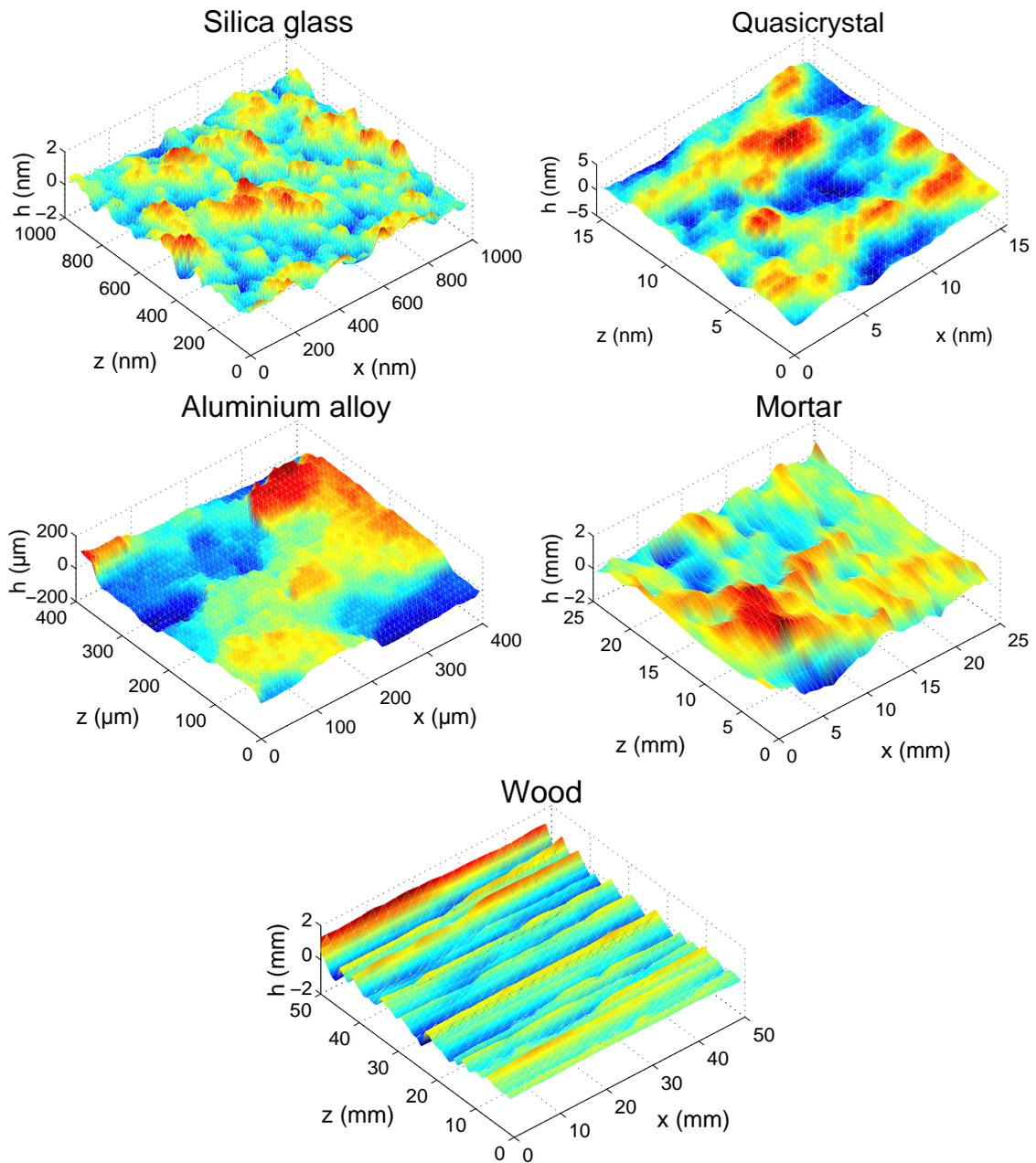
Figure 2.1: Topographic images of fracture surfaces of silica glass, AlPdMn quasicrystal, aluminum alloy, mortar and wood. Square fracture regions are represented here for the sake of clarity. The  $x$ -axis and  $z$ -axis correspond to the crack propagation direction and to the crack front direction respectively.
