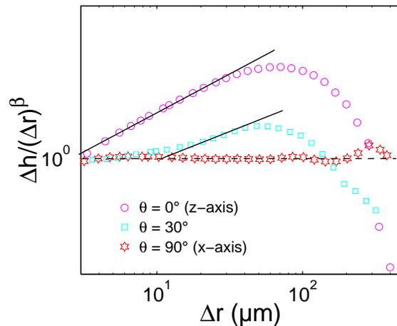
Figure 2.6: 1D normalized height–height correlation functions measured on an aluminum fracture surface for three directions corresponding to angles of  $0^\circ$ ,  $30^\circ$  and  $90^\circ$  with the  $z$ -axis. The functions are normalized by  $(\Delta r)^\beta$  with  $\beta = 0.57$ . The straight solid lines correspond to the power-law behavior with exponent  $\zeta - \beta = 0.17$ .
