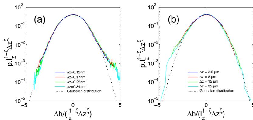
Figure 2.4: Normalized distribution of height fluctuations presented in Fig. 2.3 in a semi-logarithmic representation for fractured silica glass (a) and aluminum alloy (b) surfaces. The Gaussian distribution  $p(x) = 1/\sqrt{2\pi}e^{-x^2/2}$  is represented as a dashed line.
