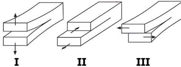
Figure 1.3: The three modes of fracture: I, tensile mode; II, shearing mode; III, tearing mode.
