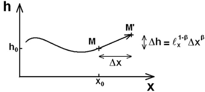
Figure 4.2: Trajectory of a point  $M$  of the crack front. While the point is moving over a distance  $\Delta x$  along the  $x$ -axis, it is also moving over the distance  $\Delta h = \ell_x^{1-\beta} \Delta x^\beta$  along the  $y$ -axis (see Eq. (4.14)).
