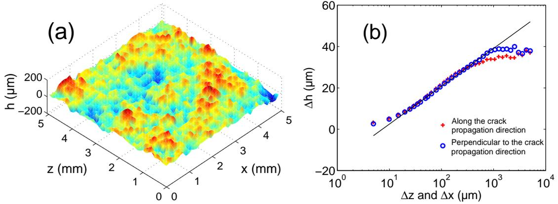
Figure 4.13: (a): Fracture surface of a metallic alloy broken at low temperature  $T = 20^\circ\text{K}$ . (b): Its correlation function computed along the  $z$  and  $x$ -axis does not follow a power-law. The corresponding curves plotted in a semi-logarithmic scales suggest that the correlation of height are logarithmic.
