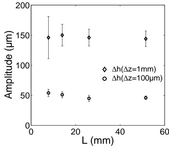
Figure 3.10: Absence of variation of the roughness amplitude of fracture surfaces of sandstone with the width  $L$  of the sample – the roughness amplitude is measured as the value of the 1D correlation function  $\Delta h(\Delta z)$  for two values of  $\Delta z$ .
