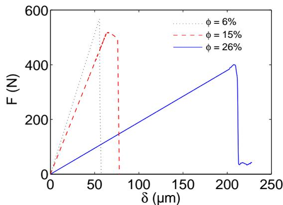
Figure A.1: Typical load versus displacement values obtained from three TDCB samples of glass ceramics with different porosities.
