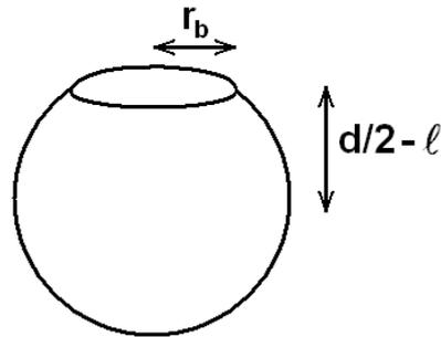
Figure A.4: Scheme of a bead with one broken bridge.
