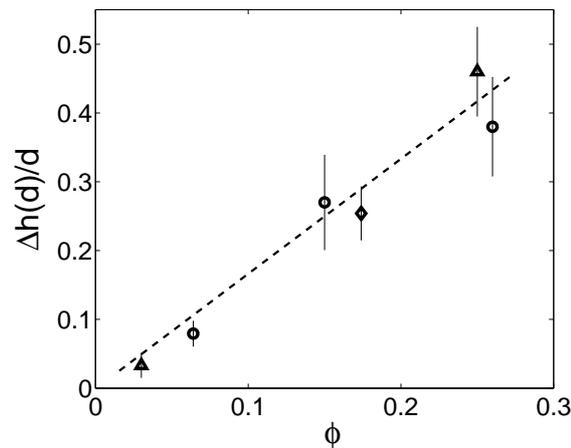
Figure 3.11: Variation of  $\Delta h(d)/d$  as a function of porosity  $\phi$  for the glass ceramics samples: Range of bead diameters used to realize samples -  $104 - 128 \mu\text{m}$  ( $\triangle$ ) : dynamic fracture ( $\circ$ ) : quasistatic fracture -  $50 - 65 \mu\text{m}$  ( $\diamond$ ) rapid fracture. The slope of the dashed line is 1.7.
