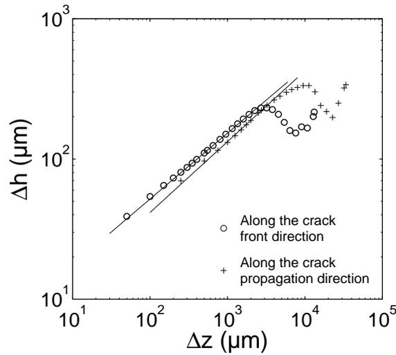
Figure 3.16: 1D height–height correlation functions measured parallel to the direction of crack propagation and to the crack front for the surface of a fractured sandstone sample with  $L = 14$  mm. The straight lines are power-law fits in the self-affine domain for  $\Delta z > d \simeq 240$   $\mu\text{m}$ . The scaling exponents, corresponding to the slope of these lines, are respectively equal to 0.46 and 0.50 parallel to the crack front and to the crack propagation.
