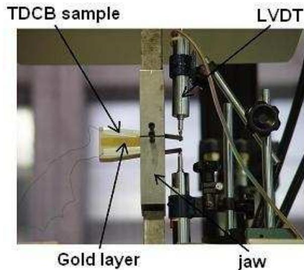
Figure 3.2: Experimental setup used to perform the quasistatic fracture tests.
