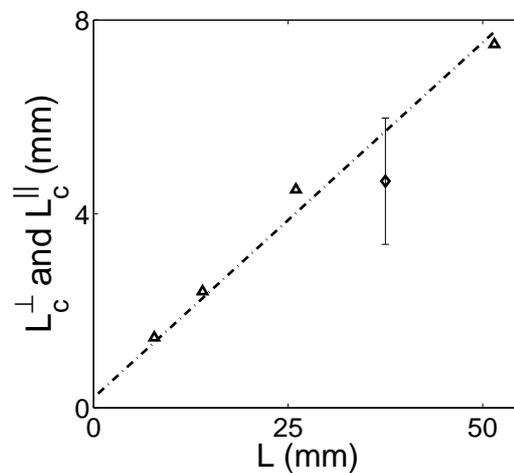
Figure 3.15: The correlation length  $L_c^\perp$  ( $\Delta$ ) (resp.  $L_c^\parallel$  ( $\diamond$ )) is plotted as a function of the specimen width (resp. the specimen length). The slope of the dashed line is 0.15.
