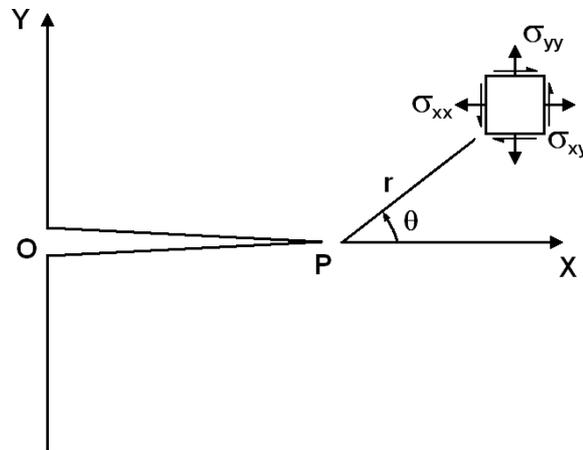
Figure 1.4: Stress field in the vicinity of the crack tip P.
