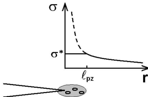
Figure 1.5: Variation of the tensile stress  $\sigma$  at the crack tip of a single crack. The distance to the crack tip for which the stress field without damage ( $\sigma = \frac{K_I}{\sqrt{2\pi r}}$ ) is equal to the intrinsic strength  $\sigma^*$  of the material gives a good estimate of the process zone size  $l_{pz}$  (see Eq. (1.9)).
