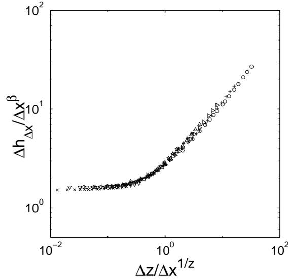
Figure 2.10: Normalized 2D height–height correlation function for an aluminum fracture surface under the condition  $z = 1$  corresponding to an isotropic surface. The collapse is found clearly better if the value  $z = 1.26$  is chosen as in Fig. 2.9. This is an additional proof of the anisotropy of fracture surfaces.
