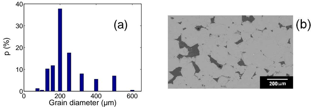
Figure 3.4: (a) : Diameter distribution of grains composing the sandstone. The mean grain size is  $d \simeq 240 \mu\text{m}$ ; (b) : Typical example of SEM images of thin strip of sandstone. The analysis of various images corresponding to different zones of the sandstone block leads to a mean porosity  $\phi = 10 \%$ .
