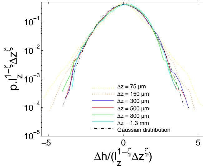
Figure 3.13: Normalized distribution of height fluctuations in a semi-logarithmic representation. For  $\zeta = 0.43$  and  $\ell_z = 35 \mu\text{m}$ , all variation curves corresponding to  $\Delta z > d = 240 \mu\text{m}$  collapse onto a single Gaussian distribution  $p(x) = 1/\sqrt{2\pi}e^{-x^2/2}$  displayed as a dashed line. It is worth noting that for  $\Delta z < d = 240 \mu\text{m}$ , data points do not collapse any more onto the master curve (dotted lines).
