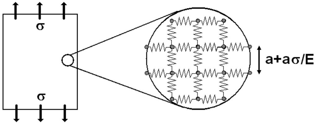
Figure 1.1: An ideal flawless solid is submitted to an exterior stress  $\sigma$ . Its atomic bonds – described by springs of stiffness  $E$  and length  $a$  – can undergo a deformation  $\delta a = a\sigma/E \simeq a/5$  before rupture. This leads to a "theoretical" strength  $E/5$  for a perfect material.
