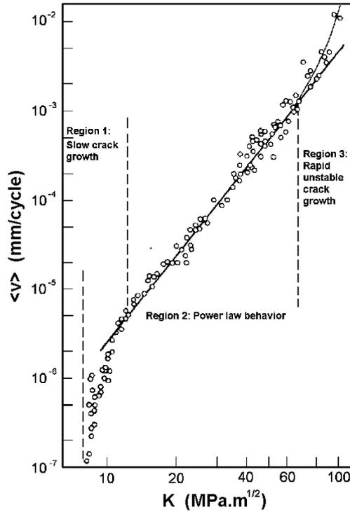
Figure 1.8: Mean crack growth velocity  $\langle v \rangle$  of a crack front propagating in a steel under cyclic loading – fatigue regime – as a function of the stress intensity factor  $\Delta K = K_{\max} - K_{\min}$  [23].
