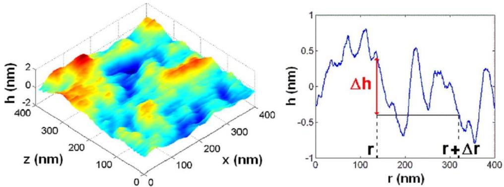
Figure 1.9: Computation of the 1D height–height correlation function  $\Delta h(\Delta r)$  on the example of a fracture surface of silica glass. The profile of interest (right) is measured along a given direction of the fracture surface (left). In addition to the use of a 3D representation, the colors on the left figure correspond to the height of each point of the fracture surface. This allows for a good visualization of the surface roughness.
