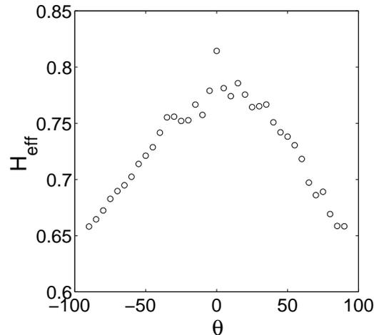
Figure 2.7: Variation of the effective Hurst exponent  $H$  measured along a direction making an angle  $\theta$  with the  $z$ -axis. The maximum and minimum (at  $0^\circ$  and  $90^\circ$  respectively) of  $H$  coincide with the  $z$  and  $x$ -axis, *i.e.* the direction of crack propagation and the direction of the crack front respectively.
