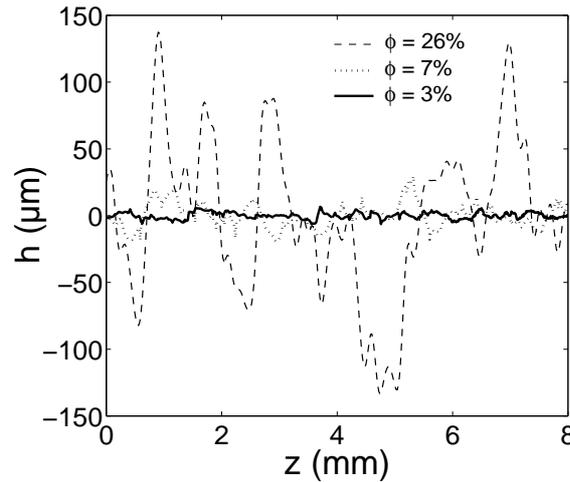
Figure 3.3: Height profiles extracted from fracture surfaces of three sintered glasses with three different porosities but with beads with the same diameter 104 – 128  $\mu\text{m}$ .
