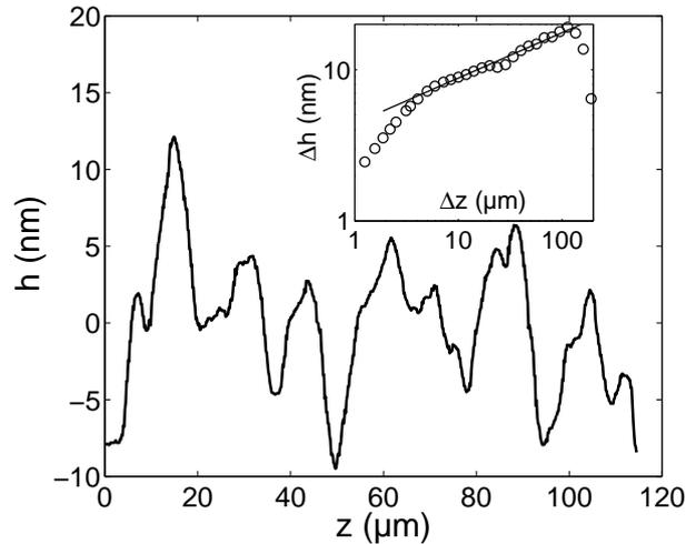
Figure 4.12: Profile extracted on a fracture surface of silica glass broken in the stress corrosion regime ( $v_{\text{crack}} < 10^{-6} \text{ m s}^{-1}$ ).
