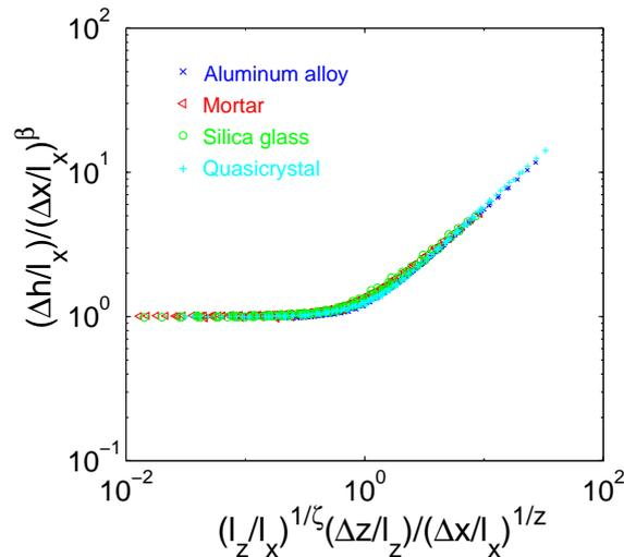
Figure 2.11: Scaling function  $f$  involved in Eq. (2.6) and measured on four different materials.
