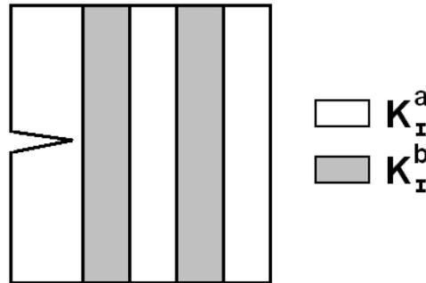
Figure 1.6: Ideal two-compounds material characterized by a one-dimensional disorder. If the toughness  $K_I^a$  of the compound  $a$  is lower than  $K_I^b$ , that of the compound  $b$ , then the macroscopic toughness of the material is  $K_I^b$ , irrespective of the properties of the compound  $a$ .
