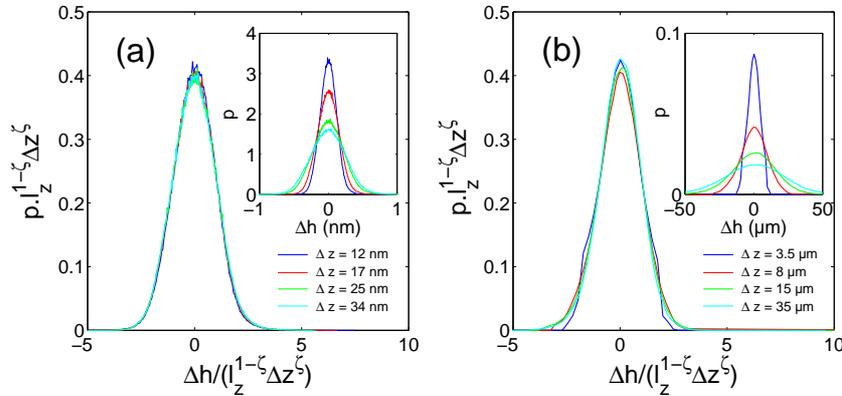
Figure 2.3: The insets show the distribution of the height fluctuations  $\Delta h$  for various values of  $\Delta z$  for fractured silica glass (a) and aluminum alloy (b) surfaces. The collapse of the curves was obtained using Eq. (2.2) with the values of the exponents  $\zeta$  and topographies  $\ell_z$  measured from the calculation of the height–height correlation function (cf. Fig. 2.2).
