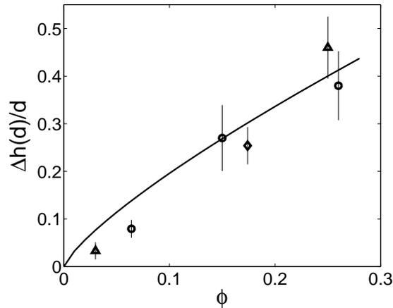
Figure 4.10: Variation of the amplitude of the roughness  $\Delta h(d)/d$  of fracture surfaces of glass ceramics samples with respect to their porosity  $\phi$ . The solid line is the theoretical prediction of the model proposed in this chapter. Note that this curve has been derived without any adjustable parameters.
