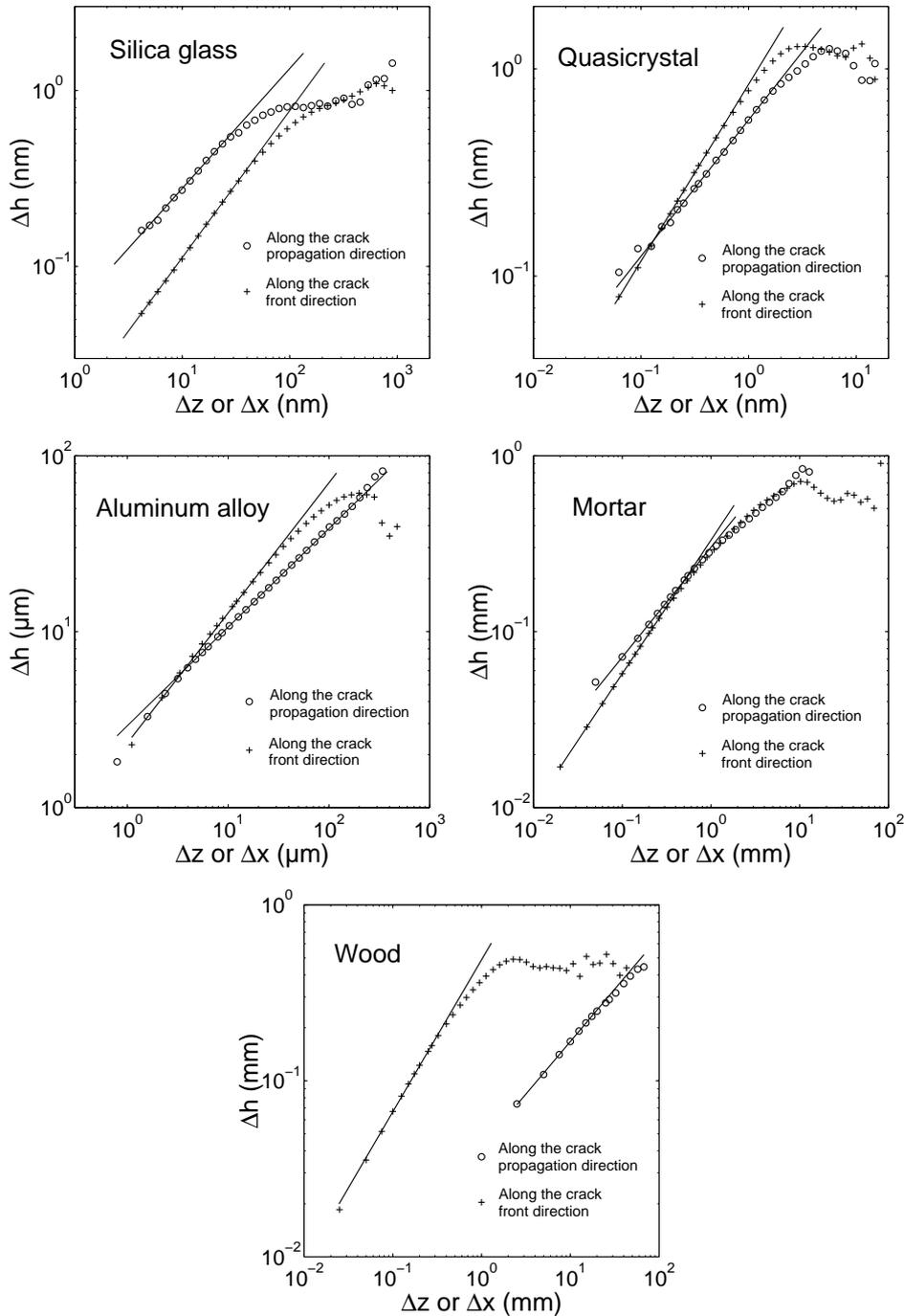
Figure 2.5: 1D height–height correlation functions measured parallel to the crack propagation direction and to the crack front for silica glass, quasicrystals, aluminum alloy, mortar and wood. The straight lines are power-law fits. The scaling exponents, corresponding to the slope of these lines, are listed in Table 2.2.
