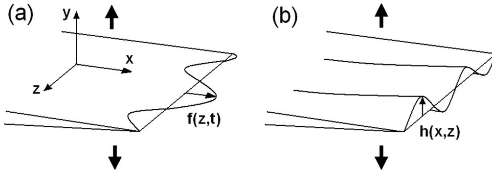
Figure 4.1: Geometry of perturbed cracks subject to mode I loading (large arrows indicating the direction of macroscopic loading). (a): In-plane perturbations. (b): Out-of-plane perturbations. The shape of the fracture surface is effectively the history of the out-of-plane perturbations of the crack front. (Taken from Ref. [40]).
