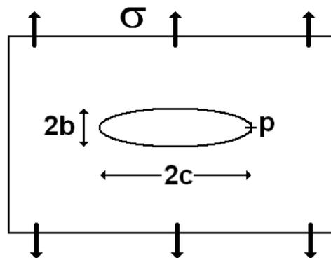
Figure 1.2: Plate containing an elliptical cavity, semi-axes  $b$  and  $c$ , subjected to uniform applied tension  $\sigma$ .
