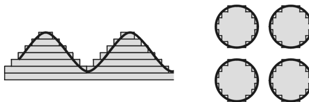
Figure 5.3: Staircase approximation of a sine grating (left) and an array of circular rods (right)
