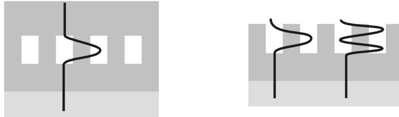
Figure 4.75: (Left) QGM in a GaN/PhC/GaN structure: the mode is trapped in the low-index region, and constitutes an easily injectable photonic crystal membrane. (Right) Generalization of the QGM to higher-order quasi-guided resonances in the PhC region. Here, the first and second resonances are depicted.
