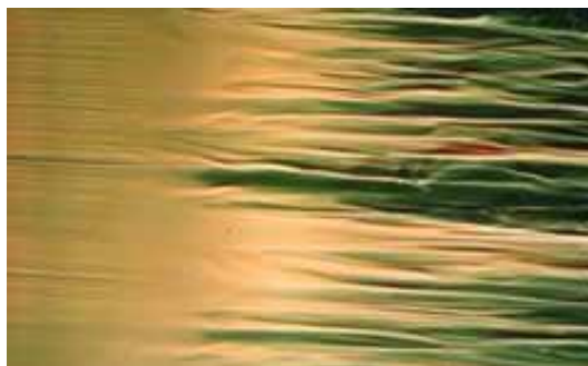
Figure 1.3: Boundary-layer transition on the surface of a flat plate, seen from the top. Flow is from left to right and dye visualization shows the transition from laminar (on the left) to turbulent flow (on the right). (Photograph courtesy of ONERA)
