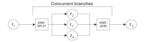
Figure 1.2: AND-SPLIT/AND-JOIN execution patterns
