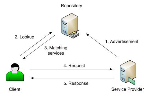
Figure 1.6: Service Oriented Architecture concepts
