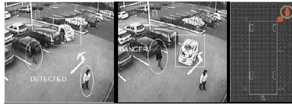
Figure 10.14: (left) two pedestrians are crossing the road. They are detected by our system. The Cycab is arriving turning right. (center) The system estimates that there is a high probability of collision between the pedestrian starting crossing the road. (right) It alerts the driver with a signal on the interface
