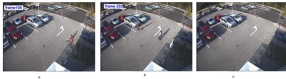
Figure 5.16: (A) frame 106, (B) frame 202, (C) estimated background
