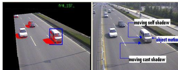
Figure 5.8: Illumination of an object surface
