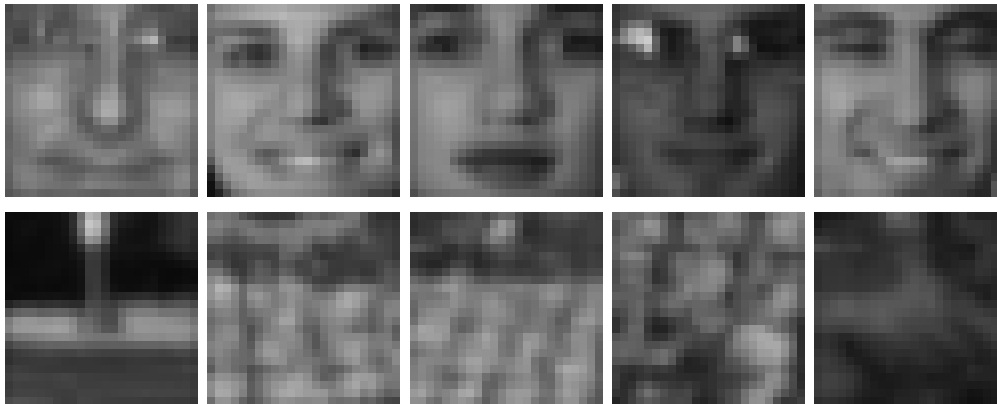
Figure 6.32: Face examples from the learning set: upper line for the positive samples and lower line for the negative examples
