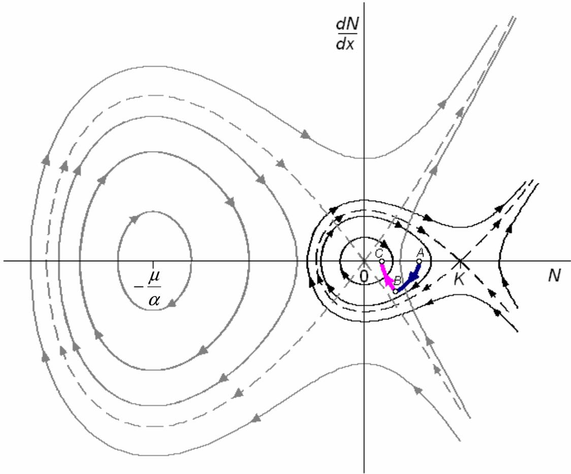
**Fig. 2.12.** Phase portrait of system (2.41). Phase trajectories of system are marked with black lines in the refuge  $\Omega_{ref}$  and with grey lines in the Bt-field  $\Omega_{Bt}$ . Separatrices are marked with dotted lines. Arc  $AB$  corresponds to the section of the closed phase trajectory which is generated by system within the refuge. Arc  $BC$  corresponds to the section of the non-closed phase trajectory of hyperbolic type, which is generated by system within the Bt-field.
