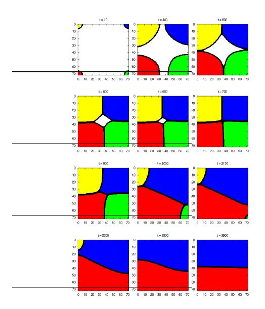
Figure 5.22: Four solids with different crystalline orientation, namely 0° (yellow), 14.3° (blue), 28.6° (red) and 43.0° (green) are growing towards each other from the corners. The interface in shown black. To ensure that the system solidifies entirely, heat is extracted from the initially undercooled system equally everywhere. As the system is totally solidified, the grain boundaries continue to move according to the curvature. The anisotropy in the system is given by  $\epsilon_4 = 0.05$ .
