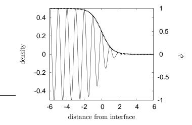
Figure 2.2: Schematic representation of the density of atom centers as function of the distance to the solid-liquid interface. The periodic structure decays over a length of a few atomic layers into the liquid. As envelope, a possible physical interpretation of the phase field  $\phi$  is shown with a heavy dashed line, varying from one to zero.
