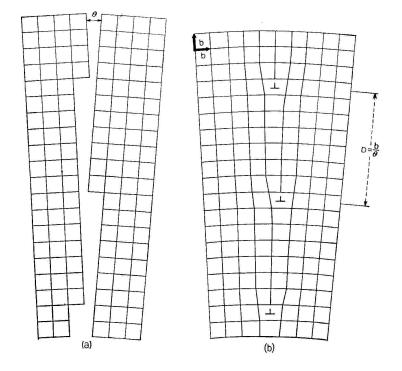
Figure 2.7: The symmetric-tilt grain boundary in a single cubic crystal is obtained by rotating two grains by an angle  $\theta$  (a) and joining them again (b). Crystalline lines end at dislocations, whose distance D is inversely proportional to the misorientation  $\theta$ . From [20].
