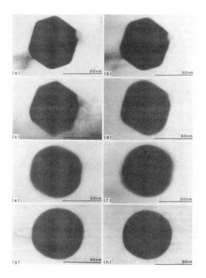
Figure 2.5: TEM images of a lead particle in a melt-spun aluminum-5 wt.% lead alloy for different temperatures: (a) room temperature, (b)  $100^{\circ}$  C, (c)  $300^{\circ}$  C, (d)  $350^{\circ}$  C, (e)  $400^{\circ}$  C, (f)  $450^{\circ}$  C, (g)  $500^{\circ}$  C, (h)  $550^{\circ}$  C. One can see how the shape changes. From the shape, the anisotropy in the solid-liquid interface energy can be obtained. From [17].
