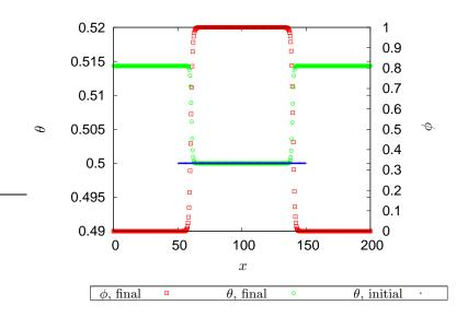
Figure 5.18: A one-dimensional system of a solid slab is surrounded by its liquid. For a stationary system with constant volume,  $u = 3.34 \times 10^{-5}$  and an anisotropy of  $\epsilon_4 = 0.05$ . In squares  $\phi$  and in circles  $\theta$  are shown.
