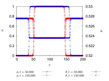
Figure 5.13: Two one-dimensional liquid-solid-liquid system at melting temperature with a solid orientation  $\theta = \pi/6$  and an anisotropy of  $\epsilon_4 = 0.05$ . The phase field  $\phi$  (circles) and the orientation  $\theta$  (squares) are shown at different times t. Contrary to the system shown in figure 5.12,  $\partial_{\theta}W \neq 0$ , the angle varies in the interface and the interface moves with time.
