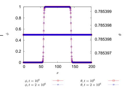
Figure 5.12: Two one-dimensional liquid-solid-liquid system at melting temperature, where the solid has a crystalline orientation  $\theta = \pi/4$  and the anisotropy is given by  $\epsilon_4 = 0.05$ . The phase field  $\phi$  (circles) and the orientation  $\theta$  (squares) are shown at different times t. Here,  $\partial_{\theta}W = 0$ , the angle is constant in the entire system and the interface does not move.
