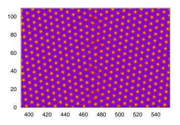
Figure 4.11: Snapshot of a grain boundary with a misorientation  $\theta = 13.2^{\circ}$ .
