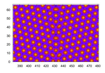
Figure 4.10: Snapshot of a grain boundary with a misorientation  $\theta=21.8^\circ\,.$
