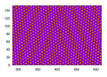
Figure 4.12: Snapshot of a grain boundary with a misorientation  $\theta=9.4^\circ\,.$
