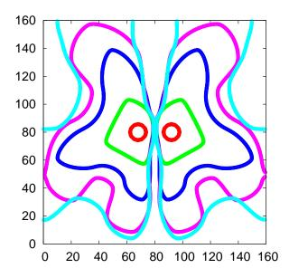
Figure 5.21: Two-dimensional system of two solids of different orientation ( $\theta = \pm \pi/10$ ) growing towards each other. In the system, the anisotropy is given by  $\epsilon_4 = 0.05$ . The interface is shown at different times.
