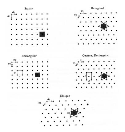
Figure 2.1: The Bravais lattices possible in two dimensions. Also shown possible basis vectors  $\vec{a}_i$  and the Wigner-Seitz cell in gray. From [1].
