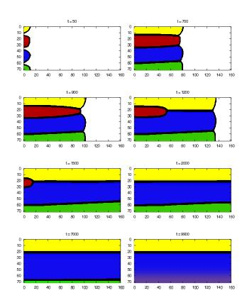
Figure 5.23: Four solids with different local crystalline orientation, namely  $0^{\circ}$  (yellow), 8.6° (blue), 25.8° (green) and 34.4 (red) are growing side by side. The interface is shown in black. One can nicely see how the growth velocity depends on the orientation and how two grains disappear during the simulation. The anisotropy in the system is given by  $\epsilon_4 = 0.05$ .
