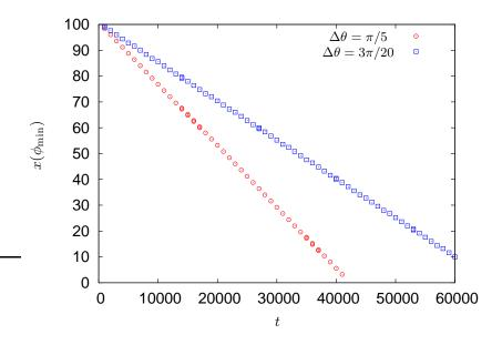
Figure 5.17: Interface position  $x(\phi_{\min})$  versus time for the systems shown in figures 5.15 and 5.16. The interface velocity is given by the slope of the curves. One can see that the system with the larger misorientation moves faster.
