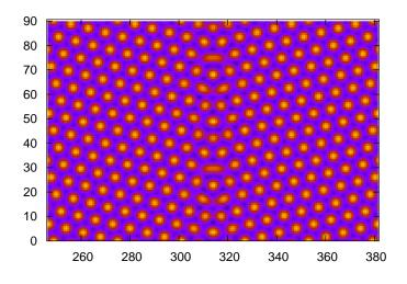
Figure 4.8: Snapshot of a grain boundary with a misorientation  $\theta=32.2^\circ\,.$
