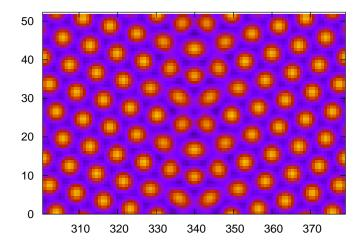
Figure 4.9: Snapshot of a grain boundary with a misorientation  $\theta = 27.8^{\circ}$ .
