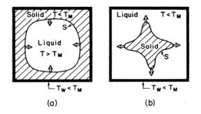
Figure 2.8: Different possibilities of solidification of a system with a boundary at a fixed temperature  $T_{\rm W} < T_{\rm M}$ , where  $T_{\rm M}$  is the melting temperature. In (a), the solidification starts from the boundary and grows into the liquid at  $T > T_{\rm M}$ and is stable. In (b), the solidification starts at a seed in the center and the solid grows into the undercooled liquid. This case is intrinsically unstable. From [23].
