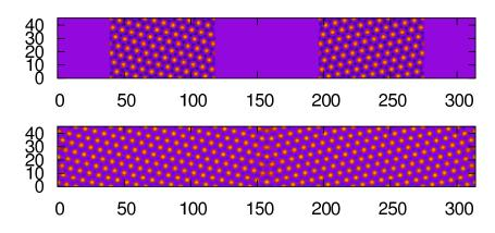
Figure 4.4: Top: Initial condition for the grain boundary simulations. Two solids with different orientations are separated by liquid layers. Bottom: After a few time steps, the liquid solidifies and the grain boundaries build up. Due to periodic boundary conditions, there are always two solid-solid interfaces: one in the middle of the system and the other one at the boundaries.
