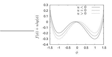
Figure 2.12: Bulk free energy density in dependency of the phase-field variable  $\phi$ . For temperatures below the melting temperature, (u < 0), the solid phase  $(\phi = 1)$  is preferred. At melting (u = 0), the energies of both phases are equal while at u > 0 the liquid phase  $(\phi = 1)$  is preferred.
