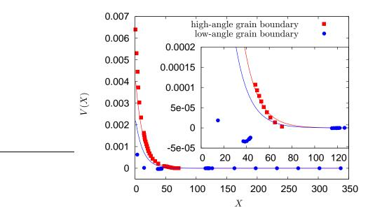
Figure 4.23: Contact potential for an high-angle and a low-angle grain boundary compared to the theory by Rappaz et al. [78]. For high-angle grain boundaries the simulations agree well with the theory, whereas for low-angle grain boundaries it fails.
