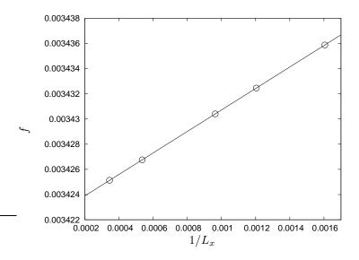
Figure 4.15: The grain boundary energy is obtained by plotting the free energy of systems with the same misorientation and average densities  $\bar{\psi}$  but different lengths  $L_x$  perpendicular to the interface against  $1/L_x$ . The slope gives twice the grain boundary energy, where the factor of two is due to the fact that in periodic systems there are always two grain boundaries.
