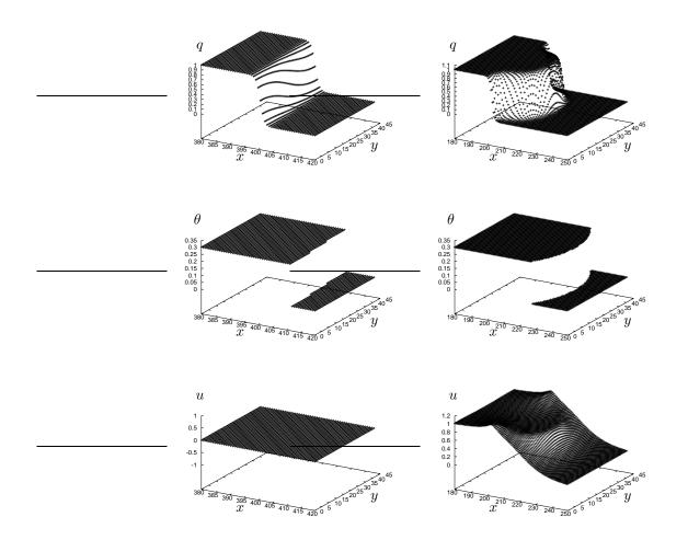
Figure 3.5: In this figure, the initial (left) and the final state (right) of a system without anisotropy and constant angle ( $\theta = 0.3$ ) is shown. The interface is initially perturbed which causes the final stationary cell to build up. The fields shown, from top to bottom: magnitude of order q, orientation angle  $\theta$  and normalized chemical potential u.
