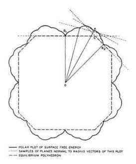
Figure 2.3: Wulff plot of a surface energy with corresponding Wulff construction to obtain the equilibrium shape. From [12].
