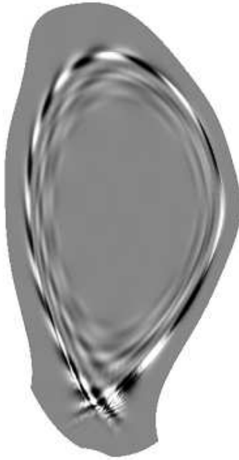
Figure 6.3: Perturbations of the toroidal current density ( J^{n=3} ) at t = 700\tau_A for the JOEK simulation without any toroidal rotation.
