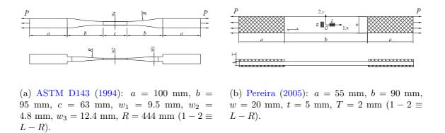
Figure 1.3: Schematic representation of tensile tests using two specimen configurations.
