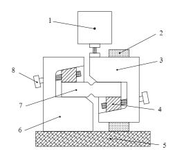
(b) 1-attachment to the test machine; 2-fixture linear guide rod; 3-movable part of the fixture; 4-adjustable wedges to tighten the specimen; 5-base; 6-stationary part of fixture; 7-specimen; 8-wedge adjusting screw.
