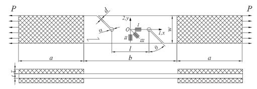
(a) a=75 mm, b=90 mm, w=30 mm, t=T=5 mm, l=30 mm, d=1 mm,  $\alpha = 4$  mm and  $\tan \theta = \{-1.5, -1, -0.5, 0, 0.5, 1, 1.5\}$   $(1-2 \equiv L-T)$ .
