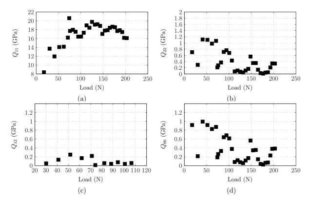
Figure 5.15: Identified stiffness parameters as function of the applied load for a 30° specimen: (a)  $Q_{11}$ , (b)  $Q_{22}$ , (c)  $Q_{12}$ , (d)  $Q_{66}$ .
