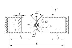
(a) clear wood specimen: l = 80 mm,  $l_1 = 32 \text{ mm}$ ,  $l_2 = 20 \text{ mm}$ , w = 20 mm, t = 8 mm, d = 12 mm, r = 2 mm and  $\theta = 90^{\circ}$ .
