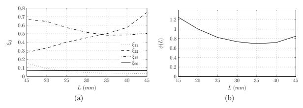
Figure 4.3: (a) Variation of the sensitivity coefficients,  $\xi_{ij} = \eta_{ij}/Q_{ij}$ , with regard to the gauge length L; (b) evaluation of the objective function  $\phi(L)$ .
