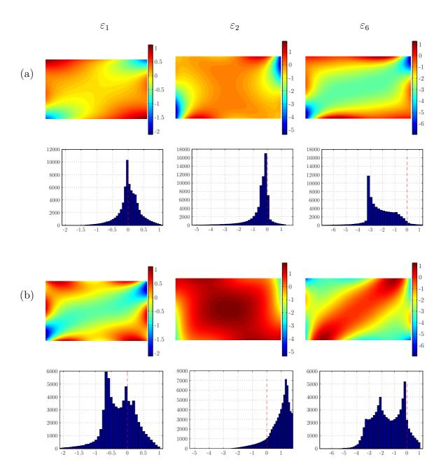
Figure 4.16: Strain field maps ( $\varepsilon_1$ ,  $\varepsilon_2$  and  $\varepsilon_6$ ), along with their histograms plots, obtained for the (L = 35 mm): (a) 0° configuration, (b) 30° configuration (unit:  $\times 10^{-3}$ ).
