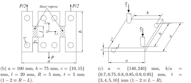
Figure 1.9: Schematic representations of the shear tests: (a) the in-plane shear test (Yoshihara and Matsumoto, 2005); (b) the quasi-simple shear test (Naruse, 2003); (c) the square-plate twist test (Yoshihara and Sawamura, 2006).
