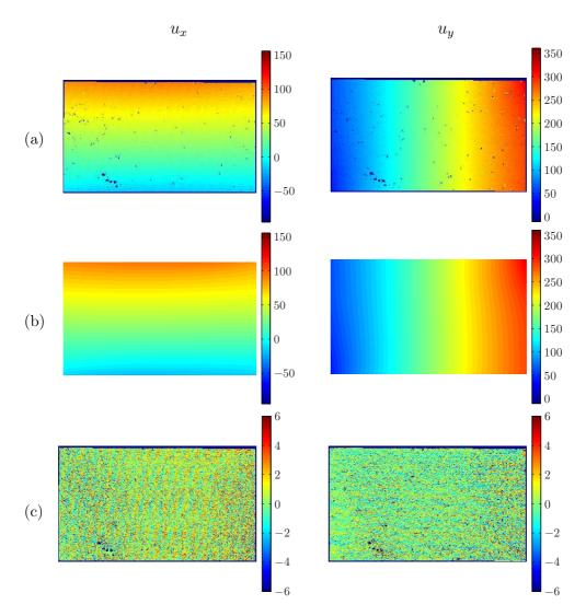
Figure 5.7: (a) Measured, (b) approximated (7th-degree polynomial) and (c) residual for  $u_x$  and  $u_y$  obtained for a 0° specimen (P = -139.4~N) (unit:  $\mu$ m).
