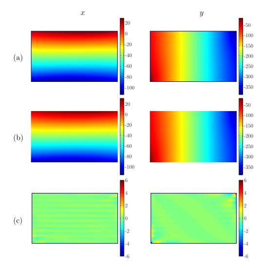
Figure 4.11: (a) Simulated, (b) approximated (7th-degree polynomial) and (c) residual x and y displacement components obtained for the layered material model  $(n = 10, w^{l} = 0.4)$ and k=2) (unit:  $\mu$ m).
