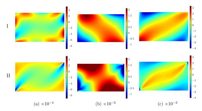
Figure 5.12: Typical (I) experimental and (II) numerical strain fields obtained for a 45° specimen ( $P = -143.0 \ N$ ): (a)  $\varepsilon_1$ , (b)  $\varepsilon_2$ , (b)  $\varepsilon_6$ .
