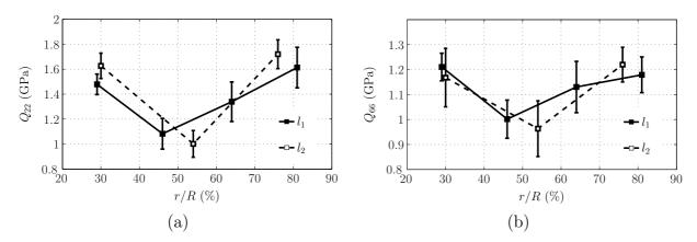
Figure 6.9: Variation of the stiffness parameters: (a)  $Q_{22}$ ; (b)  $Q_{66}$ , identified at the two vertical locations 1 ( $\blacksquare$ ) and 2 ( $\square$ ) as a function of the radial position (r/R).
