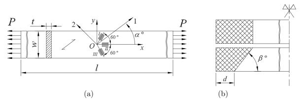
Figure 1.6: Off-axis tensile test: (a) schematic representation (l = 200 mm, w = 20 mm, t = 5 mm,  $\alpha = 15^{\circ}$ ); (b) rectangular and oblique end tabs.
