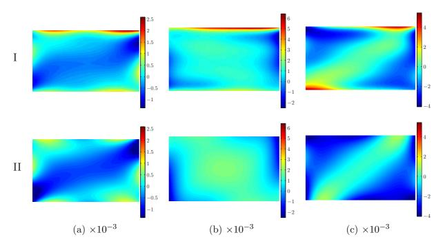
Figure 5.14: Typical (I) experimental and (II) numerical strain fields obtained for a 30° specimen ( $P = -176.5 \ N$ ): (a)  $\varepsilon_1$ , (b)  $\varepsilon_2$ , (b)  $\varepsilon_6$ .
