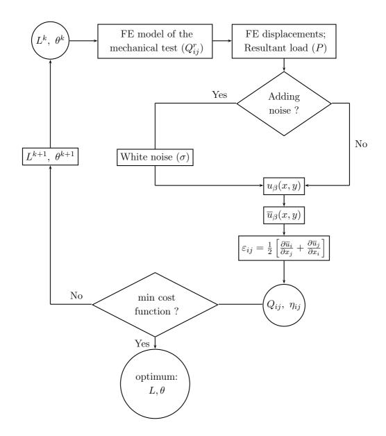
Figure 4.14: Algorithm used in the optimisation scheme of the configuration of the unnotched Iosipescu specimen.
