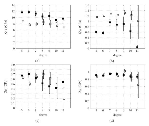
Figure 5.6: Variation of the stiffness parameters with respect to the degree of the fitting polynomial for  $0^{\circ}$  ( $\blacksquare$ ) and  $45^{\circ}$  ( $\square$ ) specimens: (a)  $Q_{11}$ , (b)  $Q_{12}$ , (c)  $Q_{22}$ , (d)  $Q_{66}$ .
