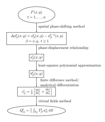
Figure 3.3: Image processing and identification flowchart.
