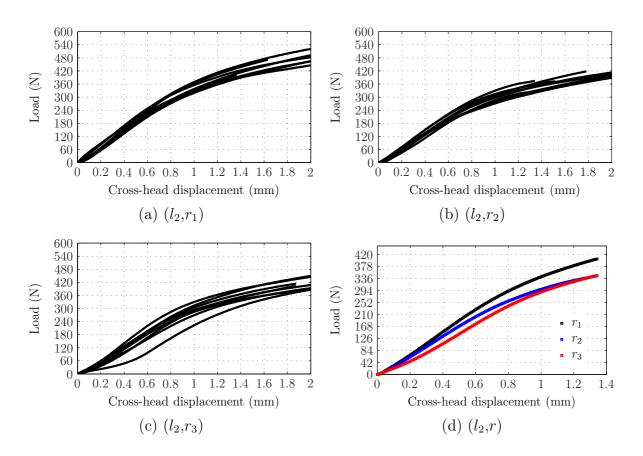
Figure 6.3: Curves of load versus cross-head displacement obtained at vertical location 2 for the radial positions: (a)  $r_1$ ; (b)  $r_2$ ; (c)  $r_3$ ; (d) average curves (displacement rate of 1 mm/min).
