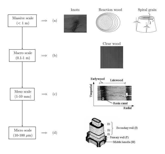
Figure 1.1: Hierarchical scales of wood.
