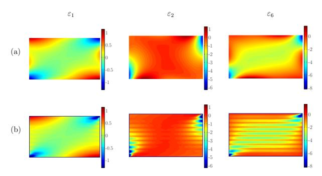
Figure 4.12: Strain field components ( $\varepsilon_1$ ,  $\varepsilon_2$  and  $\varepsilon_6$ ) of the layered material model (P = -261.2 N): (a) obtained from numerical differentiation of the polynomial displacement fields; (b) delivered directly from ANSYS (unit:  $\times 10^{-3}$ ).
