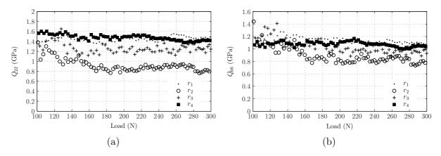
Figure 6.5: Identified stiffness parameters at vertical location 1 as a function of the applied load: (a)  $Q_{22}$ ; (b)  $Q_{66}$ .
