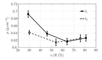
Figure 6.4: Variation of the oven-dry density  $(\rho)$  at vertical locations 1  $(\blacksquare)$  and 2  $(\square)$  with the radial positions.
