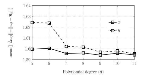
Figure 4.6: Evaluation of the residual  $(\Delta u_{\beta}, \beta = x, y)$  of the difference between simulated  $(u_{\beta})$  and approximated  $(\overline{u}_{\beta})$  displacement fields, with the increase of the degree (d) of the fitting polynomial (unit:  $\mu$ m).
