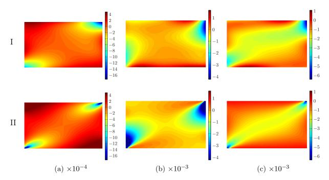
Figure 5.8: Typical (I) experimental and (II) numerical strain fields obtained for a 0° specimen  $(P = -139.4 \ N)$ : (a)  $\varepsilon_1$ , (b)  $\varepsilon_2$ , (b)  $\varepsilon_6$ .
