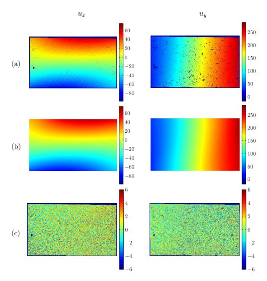
Figure 5.11: (a) Measured, (b) approximated (7th-degree polynomial) and (c) residual for  $u_x$  and  $u_y$  obtained for a 45° specimen (P = -143.0~N) (unit:  $\mu$ m).
