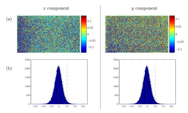
Figure 5.5: (a) Residual maps of the displacement typically obtained from experimental measurements; (b) Verification of the Gaussian distribution of the residual values of the displacement  $(-\cdot -: 2\sigma)$  (unit:  $\mu m$ ).
