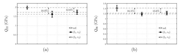
Figure 6.10: Comparison of the stiffness parameters: (a)  $Q_{22}$ ; (b)  $Q_{66}$ , identified at the two vertical locations 1 ( $\blacksquare$ ) and 2 ( $\square$ ) at the outmost radial position,  $r_4$  and  $r_3$ , respectively, with regard to reference values ( $\bigcirc$ ).
