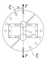
Figure 1.8: Schematic representations of: (a) the Arcan shear test (for clear wood specimen: l=70 mm, w=50 mm, t=8 mm, d=30 mm, r=2 mm and  $\theta=110^{\circ}$ ); (b) the Arcan fixture.
