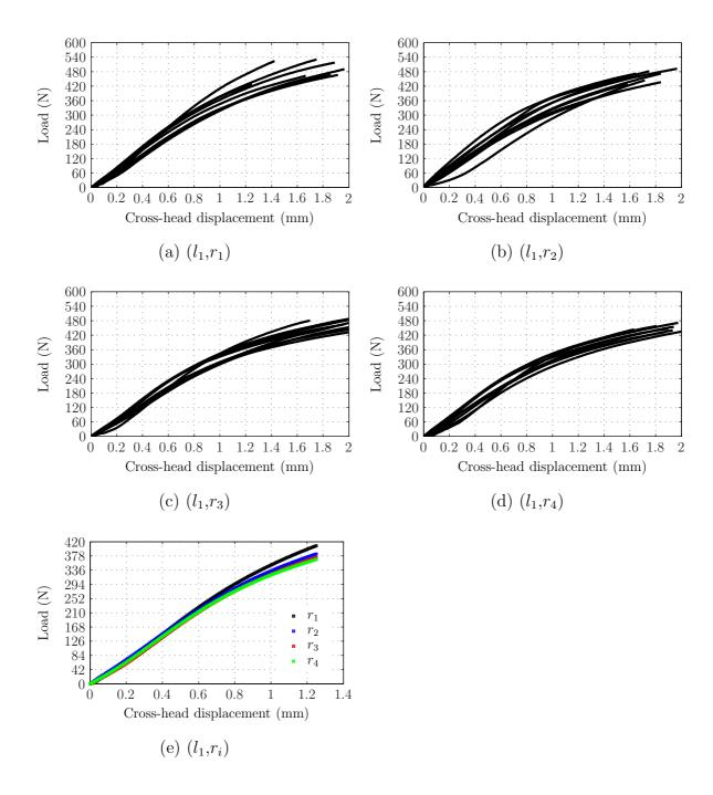
Figure 6.2: Curves of load versus cross-head displacement obtained at vertical location 1 for the radial positions: (a)  $r_1$ ; (b)  $r_2$ ; (c)  $r_3$ ; (d)  $r_4$ ; (e) average curves (displacement rate of 1 mm/min).
