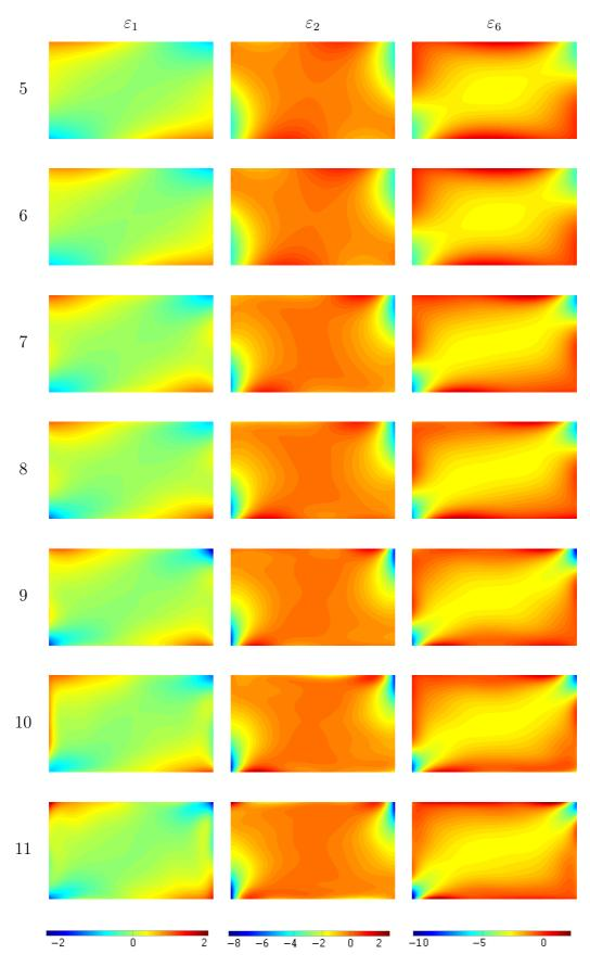
Figure 4.7: Typical strain fields (P = -261.8 N): (a)  $\varepsilon_1$ , (b)  $\varepsilon_2$ , (b)  $\varepsilon_6$ , obtained for the 0° specimen by differentiating (finite difference scheme) 2D polynomial displacements with degrees (d) ranging from 5 to 11 (unit:  $\times 10^{-3}$ ).
