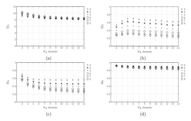
Figure 5.9: Variation of the identified stiffness components with respect to the number of elements used to set up the *virtual* mesh of the 0° specimen: (a)  $Q_{11}$ , (b)  $Q_{12}$ , (c)  $Q_{22}$ , (d)  $Q_{66}$ .
