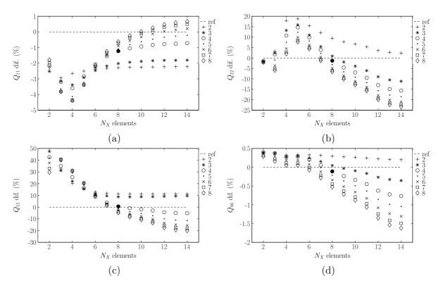
Figure 4.8: Relative differences of the (a)  $Q_{11}$ , (b)  $Q_{22}$ , (c)  $Q_{12}$  and (d)  $Q_{66}$  stiffness components, with regard to reference values, identified using piecewise virtual fields defined over a mesh of  $N_X = \{2, 3, ..., 14\}$  and  $N_Y = \{2, 3, ..., 8\}$  elements (using a 7th-degree polynomial displacement without noise).
