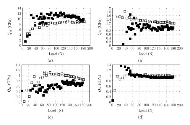
Figure 5.10: Identified stiffness parameters as a function of the applied load for a 0° ( $\blacksquare$ ) and 45° ( $\square$ ) specimens: (a)  $Q_{11}$ , (b)  $Q_{22}$ , (c)  $Q_{12}$ , (d)  $Q_{66}$ .
