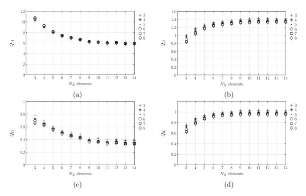
Figure 5.13: Variation of the identified stiffness components with regard to the number of elements used to set up the *virtual* mesh of the 45° specimen: (a)  $Q_{11}$ , (b)  $Q_{12}$ , (c)  $Q_{22}$ , (d)  $Q_{66}$ .
