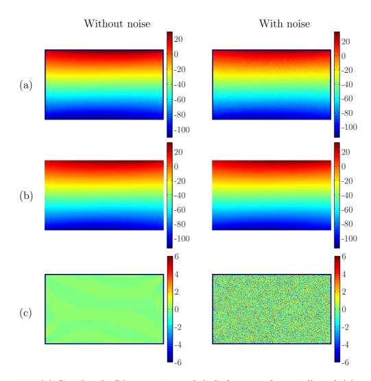
Figure 4.4: (a) Simulated, (b) approximated (7th-degree polynomial) and (c) residual  $u_x$  displacement component obtained for the 0° specimen (without and with adding a Gaussian white noise with  $\sigma_u = 2 \ \mu \text{m}$ ) (unit:  $\mu \text{m}$ ).
