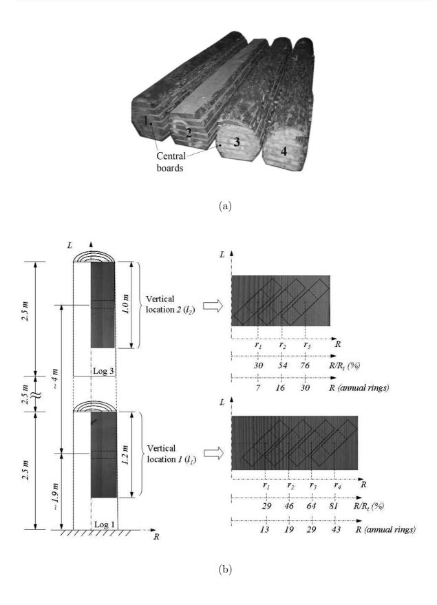
Figure 6.1: (a) Logs (1, 2, 3 and 4) of the *P. pinaster* tree from where specimens were manufactured; (b) schematic representation of the specimen sampling within the stem.
