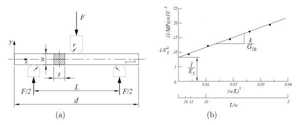
Figure 1.10: Schematic representation of: (a) the 3 point bending test (for clear wood specimen:  $d \ge 420$  mm,  $L = \{107, 129, 173, 400\}$  mm, w = 20 mm, t = 20 mm and t = 15 mm); (b) the variable span method for the identification of the longitudinal and shear moduli ( $\beta = R, T$ ).
