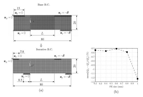
Figure 4.2: (a) Finite element model of the unnotched Iosipescu test, with L=34 mm ( $\delta=0.4$  mm, FE size = 0.6 mm); (b) meshing refinement study –  $Q_{ij}^r$  and  $Q_{ij}$  are, respectively, the reference and identified stiffness parameters.
