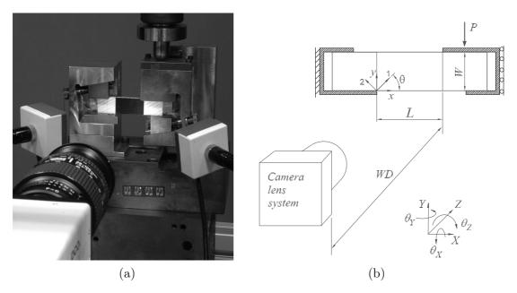
Figure 5.3: (a) Photo and (b) schematic of the mechanical set—up (WD (working distance)  $\sim 450$  mm).
