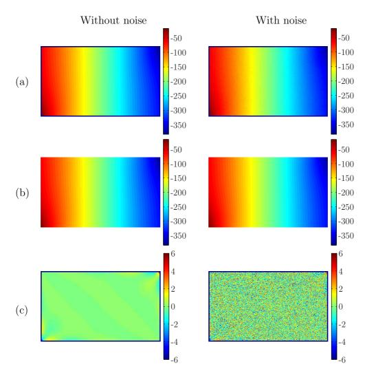
Figure 4.5: (a) Simulated, (b) approximated (7th-degree polynomial) and (c) residual  $u_y$  displacement component obtained for the 0° specimen (without and with adding a Gaussian white noise with  $\sigma_u = 2 \ \mu \text{m}$ ) (unit:  $\mu \text{m}$ ).
