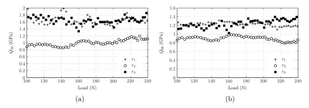
Figure 6.6: Identified stiffness parameters at vertical location 2 as a function of the applied load: (a)  $Q_{22}$ ; (b)  $Q_{66}$ .
