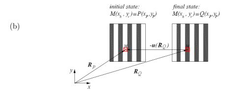
Figure 3.2: (a) Schematic representation of the grid principle: (a) imaging system (b) grid deformation.
