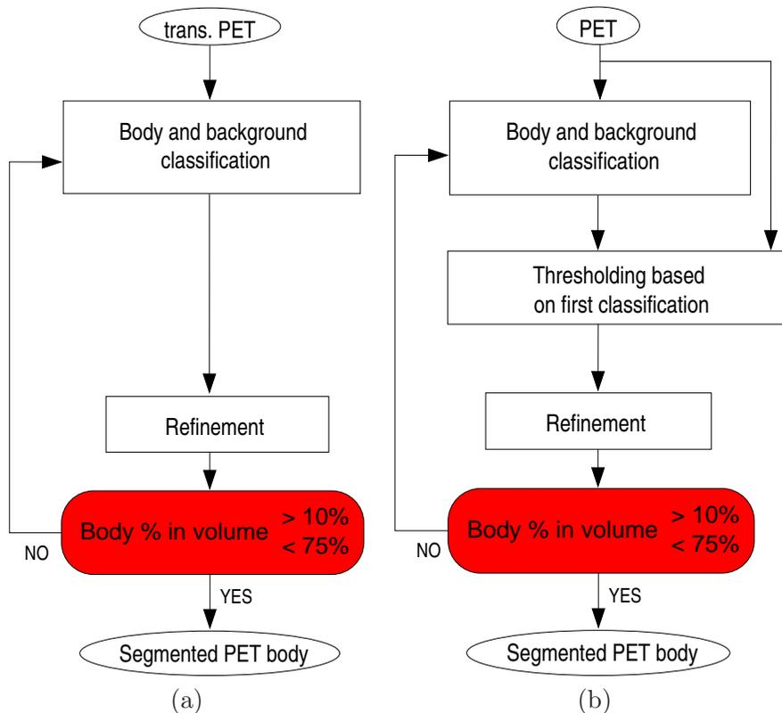
**Figure 3.5:** Diagrams of the segmentation of the body in PET images (a) using the transmission PET image (when available) and (b) using directly the original PET image. Red boxes indicate integration of anatomical knowledge *in order to detect potential errors and repair*.
