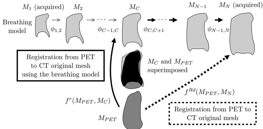
**Figure 5.4:** Registration framework on PET ( $M_{PET}$ ) and CT mesh ( $M_N$ ) – The  $M_C$  mesh is the closest to the  $M_{PET}$  mesh. We can register  $M_{PET}$  to the  $M_N$  mesh (original CT) following one of the two paths.
