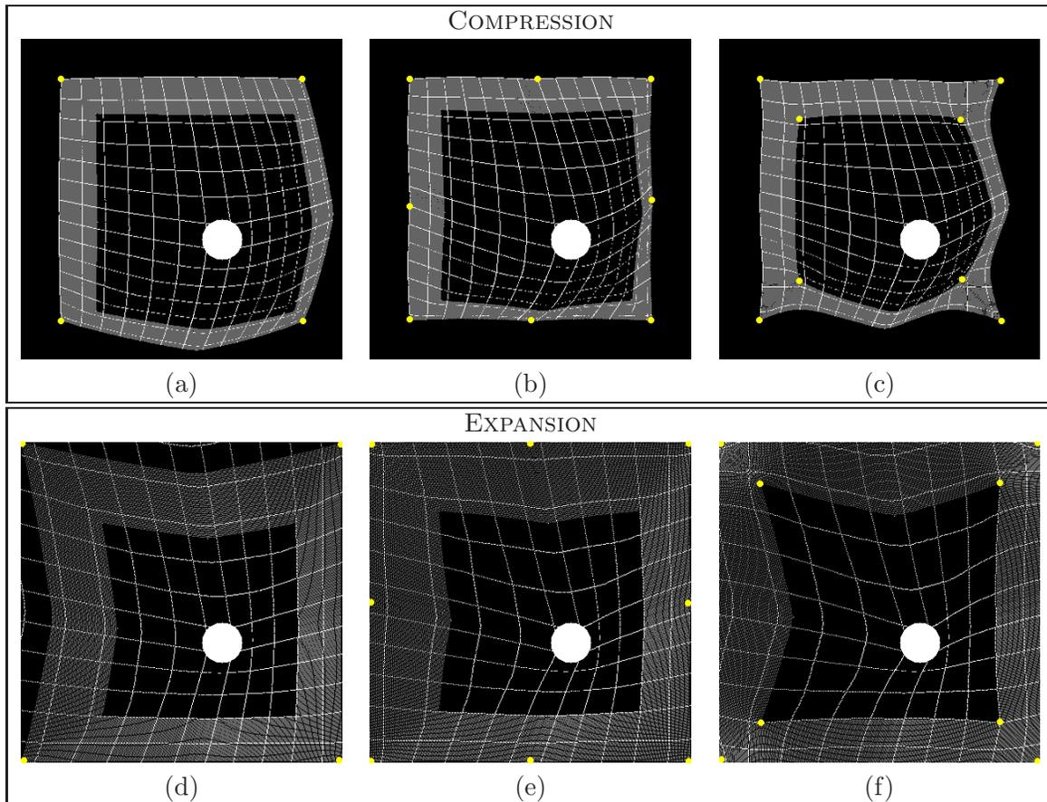
**Figure 4.7:** More registration results on synthetic images when shrinking (a-c) and expanding a frame (d-f). The registration is computed using 4 landmarks in (a) and (d), 8 landmarks on the external edge of the grey frame in (b) and (e), and 8 landmarks on the internal and external corners of the grey frame in (c) and (f).
