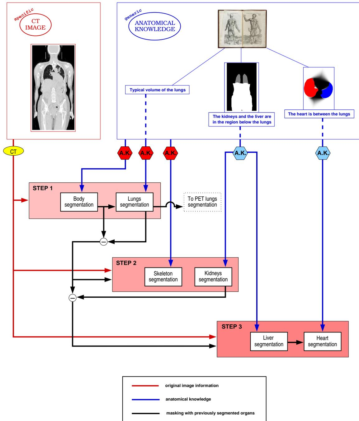
**Figure 3.1:** General diagram for segmentation of CT images. *General anatomical knowledge (A.K.) is integrated a priori (ellipses in yellow), directly in the method (hexagons in light blue) and in order to detect potential errors and repair (hexagons in red) as explained in Chapter 2, Figure 2.5.*
