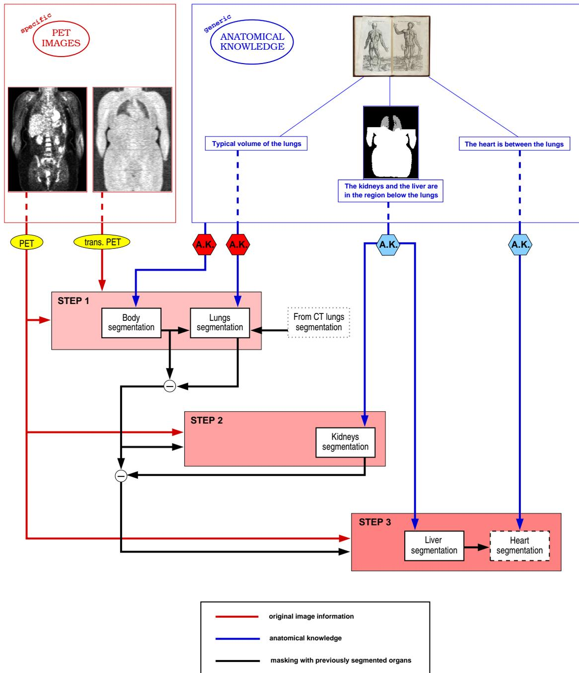
**Figure 3.2:** General diagram for segmentation of PET images. *General anatomical knowledge (A.K.) is integrated a priori (ellipses in yellow), directly in the method (hexagons in light blue) and in order to detect potential errors and repair (hexagons in red) as explained in Chapter 2, Figure 2.5.*
