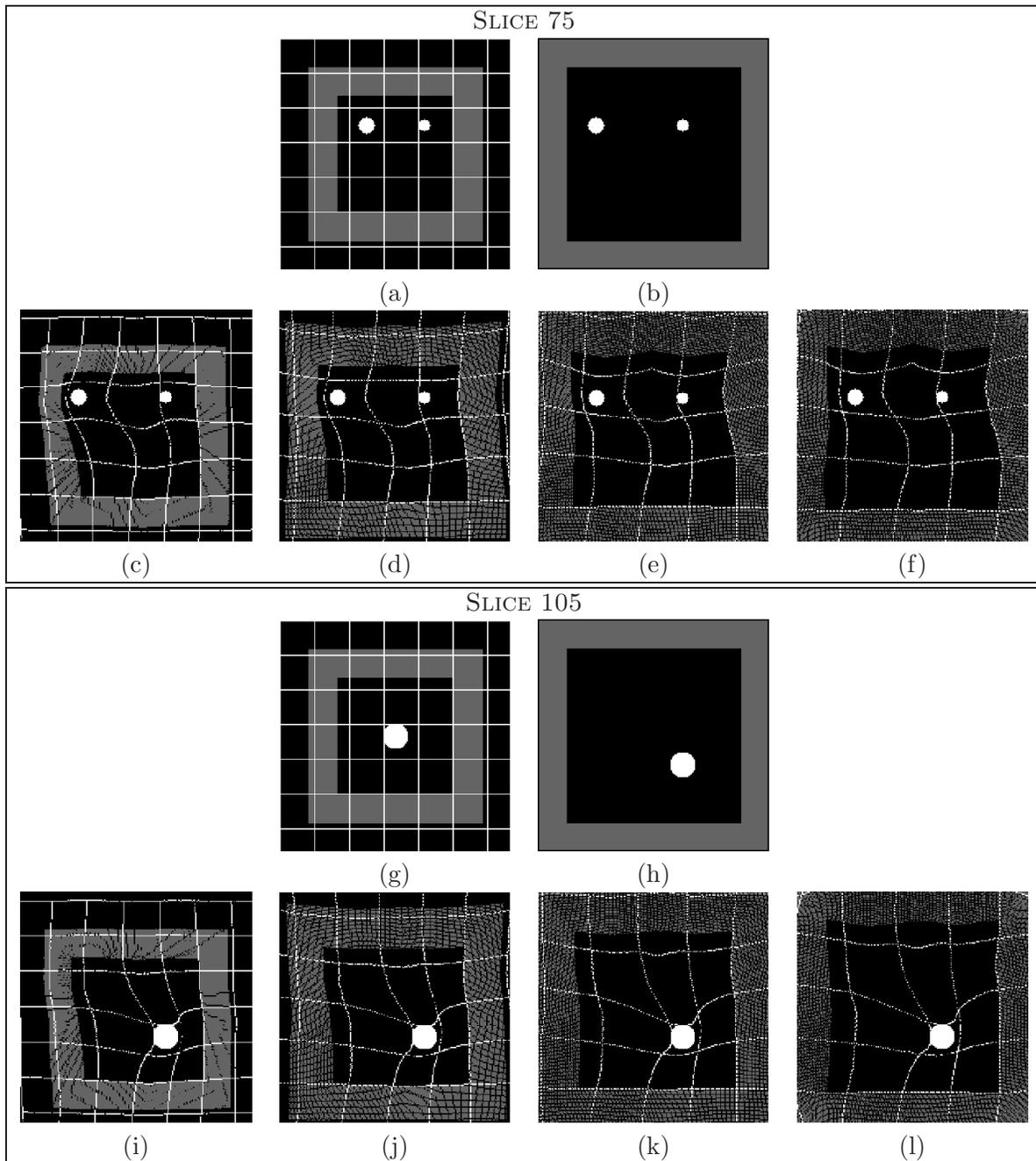
**Figure 4.8:** Results of registration on 3D synthetic images including three rigid structures. The results are shown on two different slices of the volumes. (a) and (g) correspond to the source image (with a grid), and (b) and (h) to the target image. (c-f) and (i-l) are the results of the transformation with 0, 8, 16 and 40 landmarks respectively. The landmarks are placed on the corners and on the middle of the edges of the grey 3D frame (not in the selected slices).
