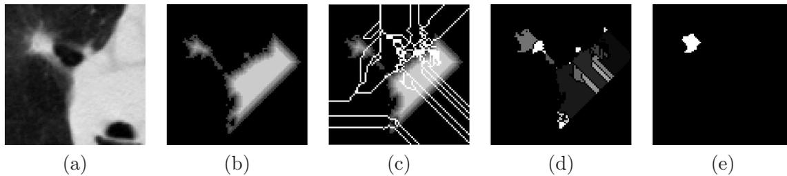
**Figure 3.33:** Illustration of the refinement algorithm: (a) detail of the original CT image, (b) distance function to the complementary of the rough segmentation, (c) result of the watershed on the inverted distance function (superimposed on the distance function), (d) components separated by the watershed and included in the rough segmentation, (e) final segmentation (selected component).
