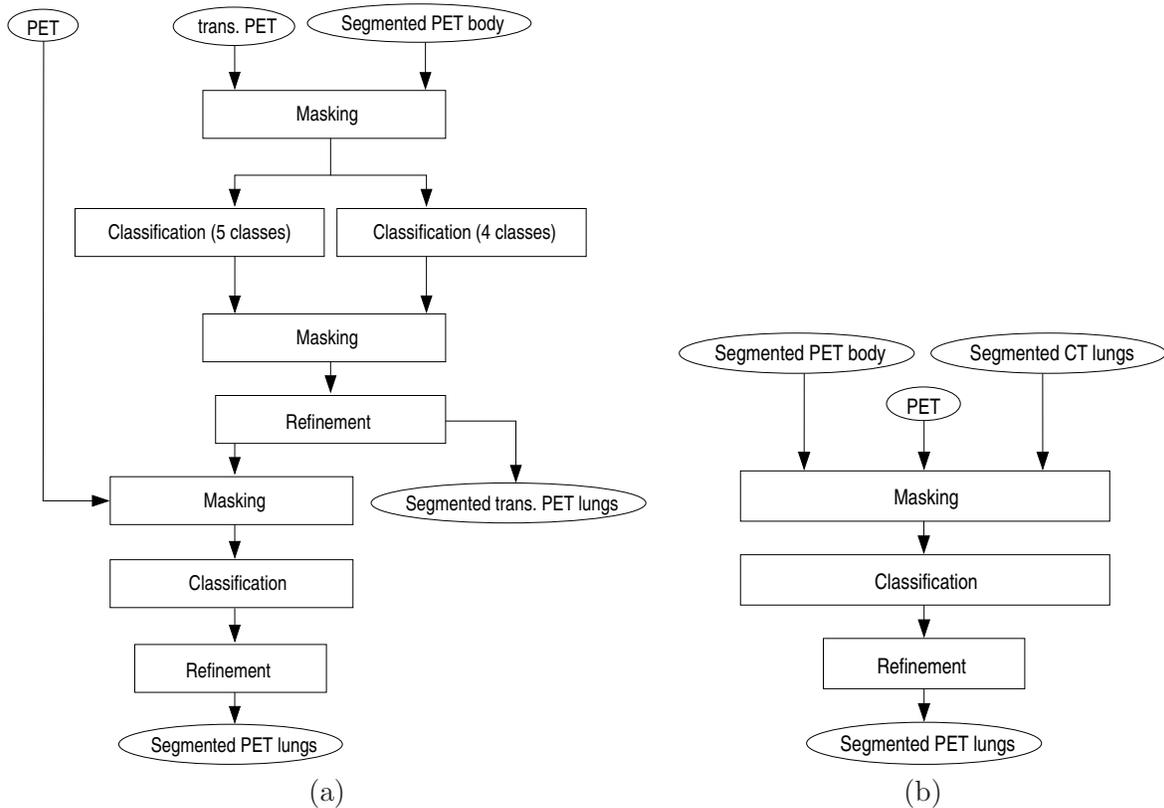
**Figure 3.12:** Diagrams of the segmentation of the lungs in PET images (a) using the transmission PET image (when available) and (b) using the segmented lungs in CT (when images come from a CT/PET combined device).
