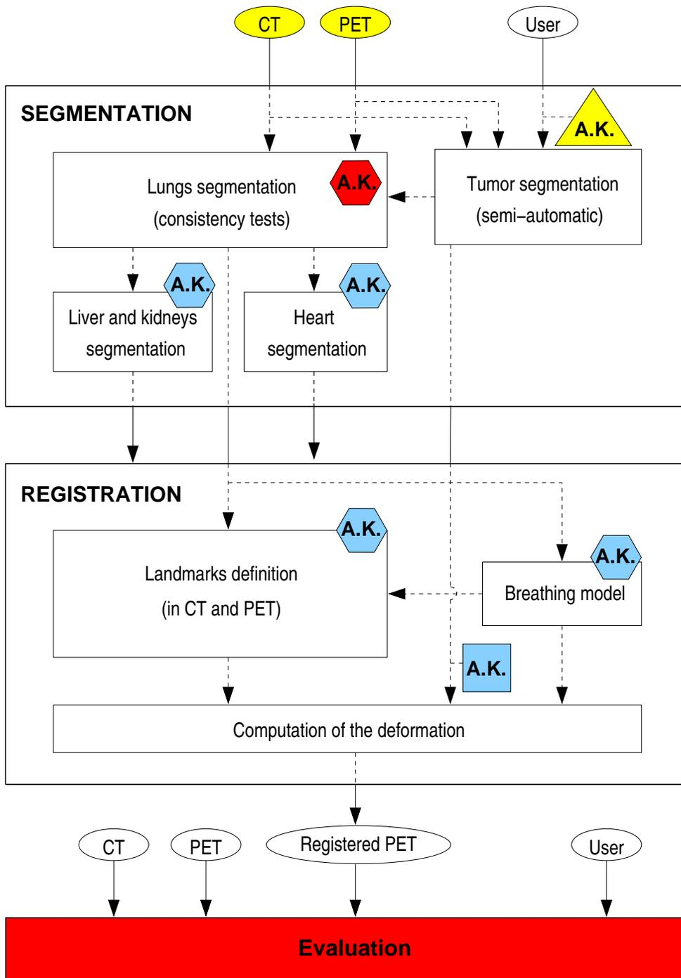
**Figure 2.5:** Diagram of our general algorithm for registration of CT and PET images using anatomical knowledge (A.K.). *General* knowledge is represented by hexagons, *individual* knowledge by triangles and *adapted* knowledge by squares. The different types of integration are marked with colors: yellow means integration *a priori*; light blue, integration *directly in the method*; and red, integration *in order to detect potential errors and repair*.
