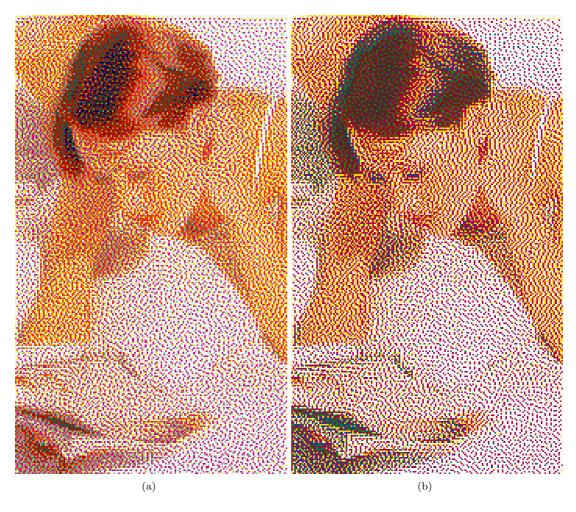
Figure C.13: Halftoning by **sVED with pre-processing and scaling** of the *WR* spectral image for the 6 and 7 colorant printers in (a) and (b) respectively.
